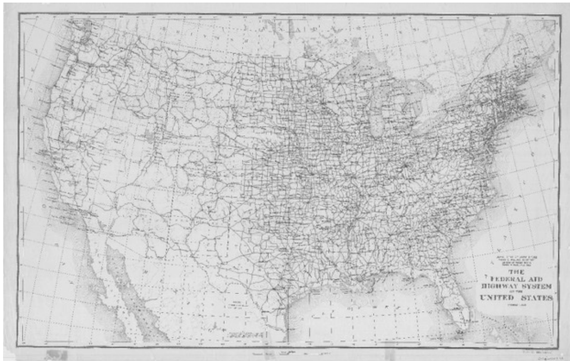
Figure 1.3: In 1923, the USDA approved the first complete national highway map. This federal aid system map represents the aggregation of state route maps, which the USDA informed and approved. Source: Original FAHS Nov. 1923, Folder 4, Series Maps of Highway System, RG 30, NARA-II.
