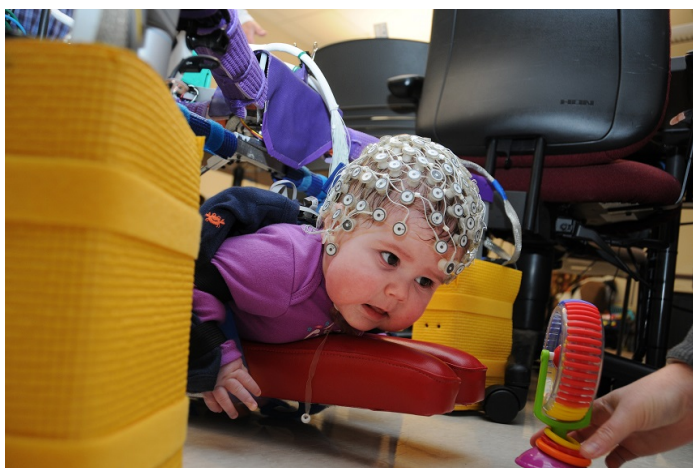
Figure 1.1: SIPPC-3, the latest generation of early intervention robotic devices for infants with CP. Image source: Sooner Magazine/Hugh Scott.
