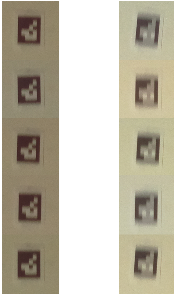
Figure 4.10: Experiment to verify predicted maximum camera shutter exposure time for a marker moving at 0.5 m/s. Left, representative marker image when it is detectable. Right, representative marker image when it is not detectable.
