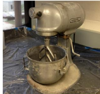
(b) Hobart mixer paddle and setup (for ASTM C305)
