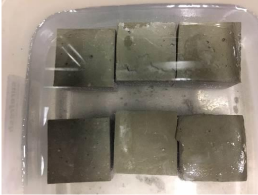
Figure 4.6 Curing cement samples in deionized water
