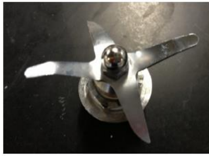
(a) Chandler high shear mixer blade and setup (for ASTM C1738)
