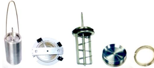
Figure 4.2 (Left to right). Slurry cup assembly, potentiometer, paddle assembly, bottom cell cap, top locking ring
