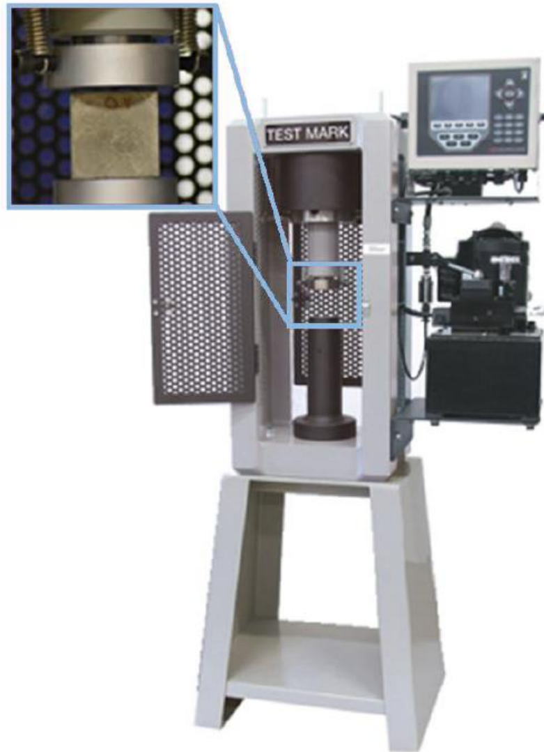
Figure 4.9 Certified UCS test machine used for destructive testing of cement samples.
