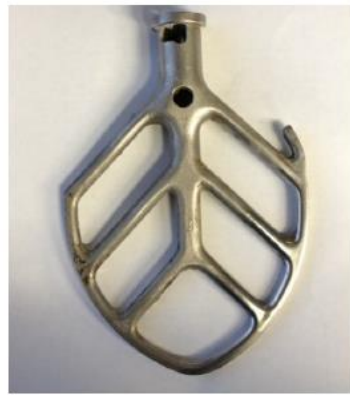
(b) Hobart mixer paddle and setup (for ASTM C305)
