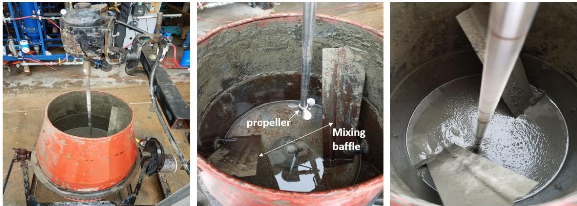
Figure 8.1 Drum baffled container and propeller used for mixing cement slurry
