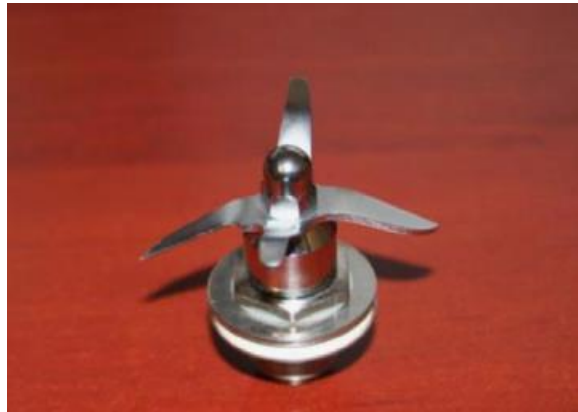
Figure 4.7 Impeller apparatus for Waring blender
