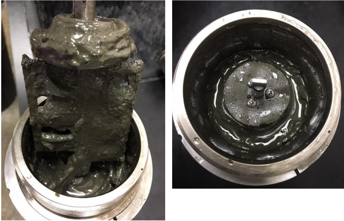
Figure 6.10 Cement slurry after thickening time tests. Slurry should be pumpable in downhole pressure and temperature conditions
