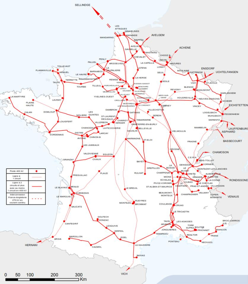
**Figure 2.1. 400-kV French power transmission network.**
