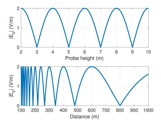
Figure 2.10: Normalized vertical electric field magnitude at the AUT versus probe height (distance of 400 m and AUT height of 10 m) and distance (probe height of 6 m and AUT height of 10 m), in the presence of ground reflections.
