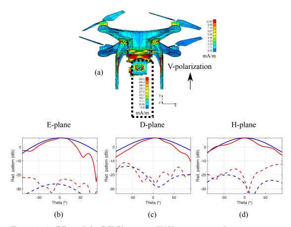
Figure 3.18: Effect of the DJI Phantom 3 UAV structure on the antenna pattern: single cell of a single layer FR4 microstrip array, vertically polarized. (a) Current density on the probe and the UAV structure. (b) E-Plane antenna patterns with and without the UAV (red and blue respectively). (c) D-Plane antenna patterns with and without the UAV (red and blue respectively). (d) H-Plane antenna patterns with and without the UAV (red and blue respectively).
