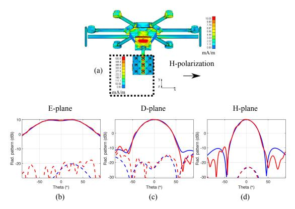
Figure 3.25: Effect of the UAV structure on the antenna pattern: central column of a  $3 \times 3$  S-Band single layer FR4 microstrip array, horizontally polarized. (a) Current density on the probe and the UAV structure. (b) E-Plane antenna patterns with and without the UAV (red and blue respectively). (c) D-Plane antenna patterns with and without the UAV (red and blue respectively). (d) H-Plane antenna patterns with and without the UAV (red and blue respectively).
