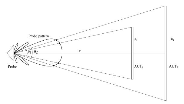
Figure 2.5: Illustration of the probe's antenna pattern projection onto the AUT's aperture.
