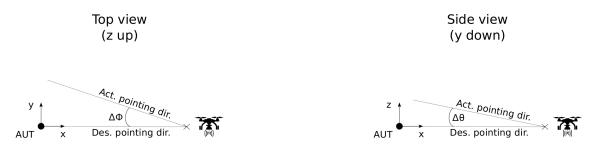
Figure 3.16: Illustration of the gimbal drift effect on the antenna pattern measurements. The probe mounted on the UAV excites the AUT—or receive its signal—at different angles in azimuth and elevation.  $\Delta \Phi$  and  $\Delta \theta$  correspond to these errors respectively.
