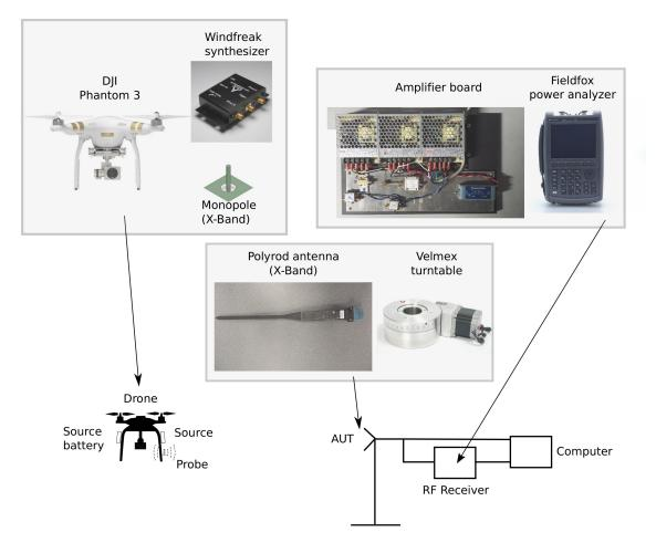
Figure 5.2: The setup used for the preliminary measurements. A DJI Phantom 3 was equipped with an X-Band monopole, fed by a Windfreak synthesizer. The AUT is an X-Band polyrod antenna, placed on a Velmex turntable, hooked up to an RF receiver, which is composed of an amplifier board and a Fieldfox power analyzer. The turntable and the power analyzer are controlled by the computer.
