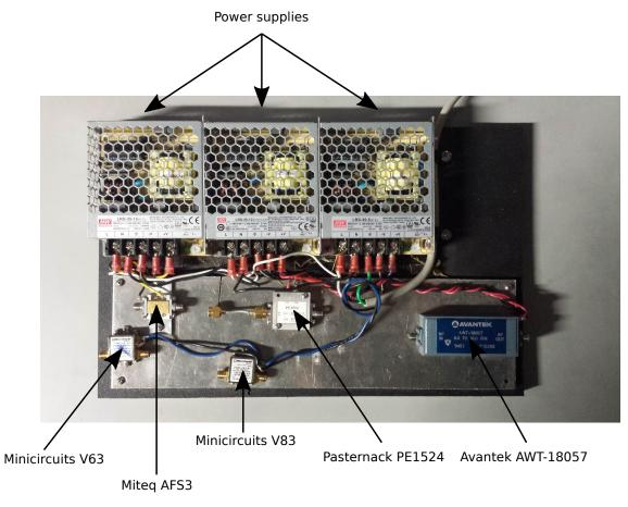
Figure 5.3: The amplifier board and its 5 amplifiers.
