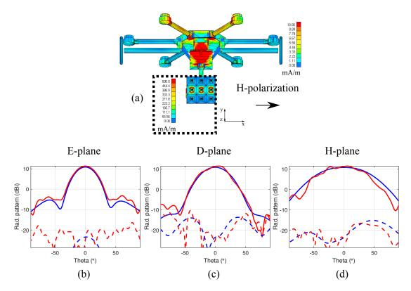
Figure 3.23: Effect of the UAV structure on the antenna pattern: central row of a  $3 \times 3$  S-Band single layer FR4 microstrip array, horizontally polarized. (a) Current density on the probe and the UAV structure. (b) E-Plane antenna patterns with and without the UAV (red and blue respectively). (c) D-Plane antenna patterns with and without the UAV (red and blue respectively). (d) H-Plane antenna patterns with and without the UAV (red and blue respectively).
