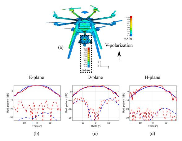
Figure 3.22: Effect of the octocopter UAV structure on the antenna pattern: central embedded element of a  $3\times3$  S-Band single layer FR4 microstrip array, vertically polarized. (a) Current density on the probe and the UAV structure. (b) E-Plane antenna patterns with and without the UAV (red and blue respectively). (c) D-Plane antenna patterns with and without the UAV (red and blue respectively). (d) H-Plane antenna patterns with and without the UAV (red and blue respectively).
