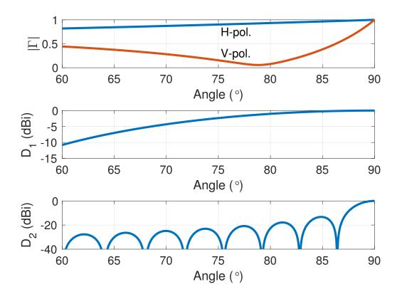
Figure 3.9: Parameters that influence the ground reflections for a 30 dB 5G antenna. The top plot is the reflection coefficient for H- and V-polarizations, the middle plot is the probe directivity, and the bottom plot is the radar directivity.
