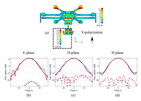
Figure 3.30: Effect of the UAV structure on the antenna pattern: all elements of a  $2 \times 2$  S-Band single layer FR4 microstrip array, vertically polarized. (a) Current density on the probe and the UAV structure. (b) E-Plane antenna patterns with and without the UAV (red and blue respectively). (c) D-Plane antenna patterns with and without the UAV (red and blue respectively). (d) H-Plane antenna patterns with and without the UAV (red and blue respectively).
