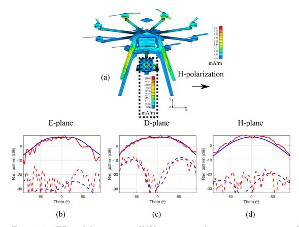
Figure 3.21: Effect of the octocopter UAV structure on the antenna pattern: central embedded element of a  $3\times3$  S-Band single layer FR4 microstrip array, horizontally polarized. (a) Current density on the probe and the UAV structure. (b) E-Plane antenna patterns with and without the UAV (red and blue respectively). (c) D-Plane antenna patterns with and without the UAV (red and blue respectively). (d) H-Plane antenna patterns with and without the UAV (red and blue respectively).
