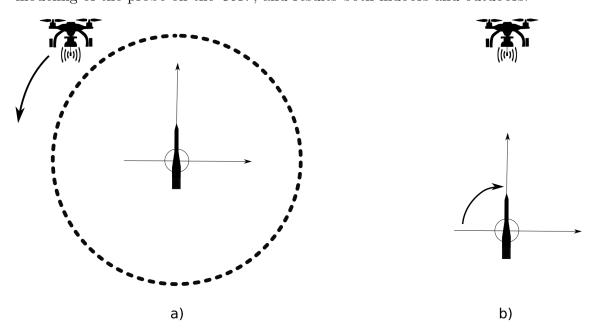
Figure 5.1: Top view of the scanning modes for the testings. a) The UAV flies around the AUT in a circle at 0-degree elevation. b) The UAV hovers in front of the AUT at 0-degree elevation while it spins on its turntable.
