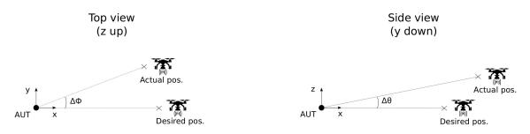
Figure 3.15: Illustration of the position drift effect on the antenna pattern measurements. The UAV measures the AUT radiation pattern at different angles in azimuth and elevation.  $\Delta \Phi$  and  $\Delta \theta$  correspond to these errors respectively.
