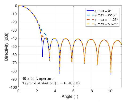
Figure 2.4: Effect of 3 different FF phase error requirements ( $\Delta \phi = 5.625$ , 11.25 and 22.5°) on the principal plane antenna pattern of a 40x40  $\lambda$  uniform square aperture with a Taylor  $\bar{n} = 6$ , -40 dB distribution.
