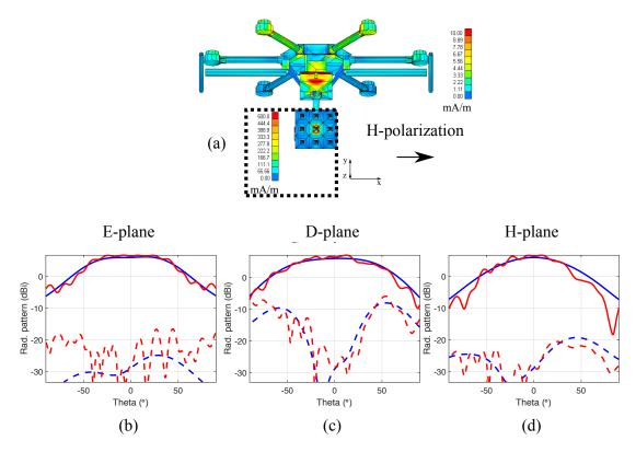
Figure 3.19: Effect of the hexacopter UAV structure on the antenna pattern: central embedded element of a  $3\times3$  S-Band single layer FR4 microstrip array, horizontally polarized. (a) Current density on the probe and the UAV structure. (b) E-Plane antenna patterns with and without the UAV (red and blue respectively). (c) D-Plane antenna patterns with and without the UAV (red and blue respectively). (d) H-Plane antenna patterns with and without the UAV (red and blue respectively).
