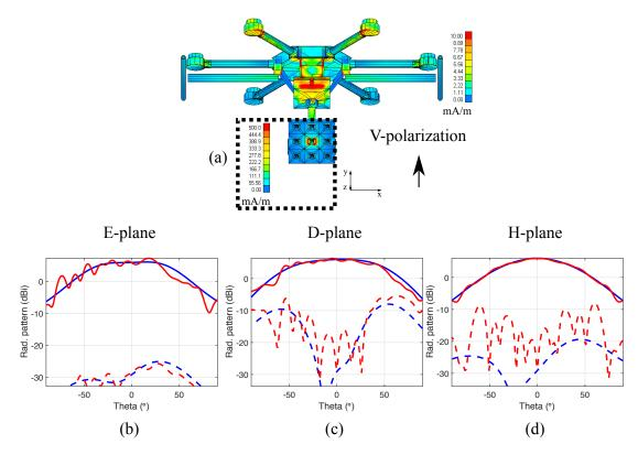
Figure 3.20: Effect of the hexacopter UAV structure on the antenna pattern: central embedded element of a  $3 \times 3$  S-Band single layer FR4 microstrip array, vertically polarized. (a) Current density on the probe and the UAV structure. (b) E-Plane antenna patterns with and without the UAV (red and blue respectively). (c) D-Plane antenna patterns with and without the UAV (red and blue respectively). (d) H-Plane antenna patterns with and without the UAV (red and blue respectively).
