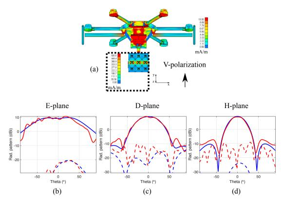
Figure 3.24: Effect of the UAV structure on the antenna pattern: central row of a  $3\times3$  S-Band single layer FR4 microstrip array, vertically polarized. (a) Current density on the probe and the UAV structure. (b) E-Plane antenna patterns with and without the UAV (red and blue respectively). (c) D-Plane antenna patterns with and without the UAV (red and blue respectively). (d) H-Plane antenna patterns with and without the UAV (red and blue respectively).
