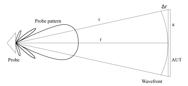
Figure 2.1: Illustration of the FF measurement configuration.
