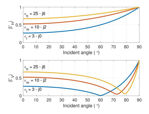
Figure 3.5: Reflection coefficient versus incident angle for 3 different permittivities, representative of soil properties, 3 - j0, 10 - j2, and 25 - j6.
