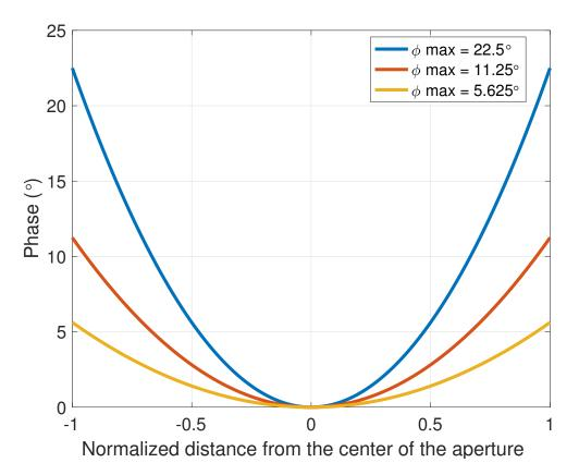
Figure 2.3: Aperture phase taper versus normalized aperture coordinates for a uniform square aperture, and 3 different FF phase error requirements ( $\Delta \phi = 5.625$ , 11.25 and 22.5°).
