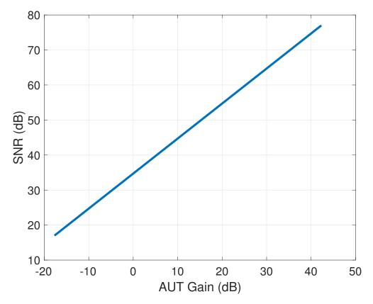
Figure B.1: Link budget (SNR) for the ATD versus its antenna gain. Parameters for these antennas are summed up in appendix B. The FF distance was chosen according to the  $8\frac{a^2}{\lambda}$  criterion for accurate sidelobe level measurements. A 12-dBi  $3\times3$  patch antenna array was used, and the noise floor is -80 dBW.
