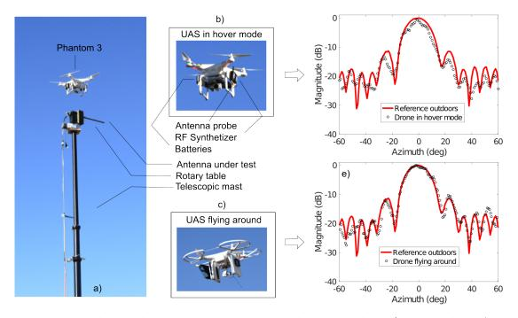
Figure 5.8: The outdoor arrangement alongside the results. a) shows the UAV in the sky in the background and the AUT on its turntable and telescopic mast in the foreground. b) shows the UAV in hover mode with the corresponding antenna pattern on the right. c) shows the UAV in flight mode—circular scan, with the corresponding antenna pattern on the right.
