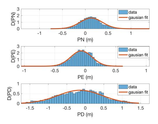
Figure 3.11: Position distributions during hover mode for the in-house ARRC hexacopter. The top plot shows the position along the North, the middle plot the position along the East, and the bottom plot the position along the axis pointing toward the center of the Earth. The blue histogram represents the actual data while the red plot is the gaussian fit applied to it.
