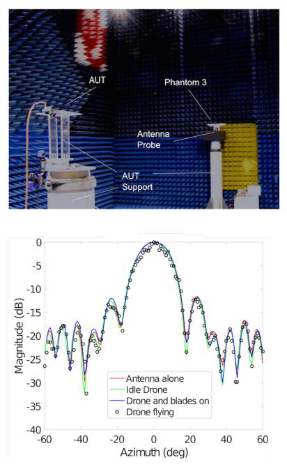
Figure 5.7: The indoor arrangement—top—and results—bottom. The testings were carried out inside a FF anechoic chamber at the ARRC, with the setup represented in figure 5.2. The results show 4 different patterns: the probe without the UAV, the probe with the UAV off, the probe with the UAV on and not flying, and the probe with the UAV hovering.
