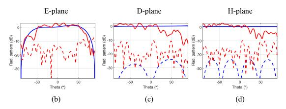
Figure 5.6: Effect of the UAV structure on the antenna pattern:  $\frac{\lambda}{4}$  monopole, vertically polarized. (a) Current density on the probe and the UAV structure. (b) E-Plane antenna patterns with and without the UAV (red and blue respectively). (c) D-Plane antenna patterns with and without the UAV (red and blue respectively). (d) H-Plane antenna patterns with and without the UAV (red and blue respectively).
