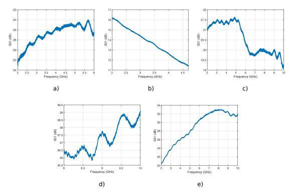
Figure 5.4: The gain for each amplifier in the frequency range of interest. a) Minicircuits V63, b) Minicircuits V83, c) Pasernack PE1524, d) Avantek AWT-18057, and e) Miteq AFS3.
