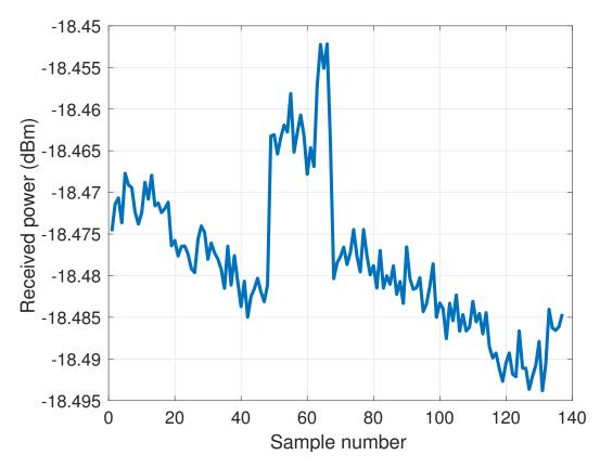
Figure 3.14: Received power at the MVG SH-2000 antenna terminals, when excited by the central embedded element of a S-Band single layer FR4 microstrip array at 3 GHz, mounted on the UAV's gimbal. The gimbal was controlled by the flight controller and its own controller (using feedback from its own IMUs and the GPS) and both antennas were aligned along their broadside directions.
