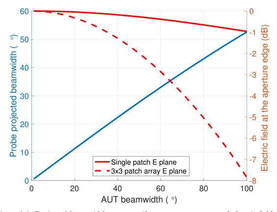
Figure 2.6: Projected beamwidth onto a uniform square aperture and electric field of a single patch antenna and a 3x3 uniform array of patch antennas  $(\frac{\lambda}{2} \text{ spacing})$  at its edge, versus its beamwidth.
