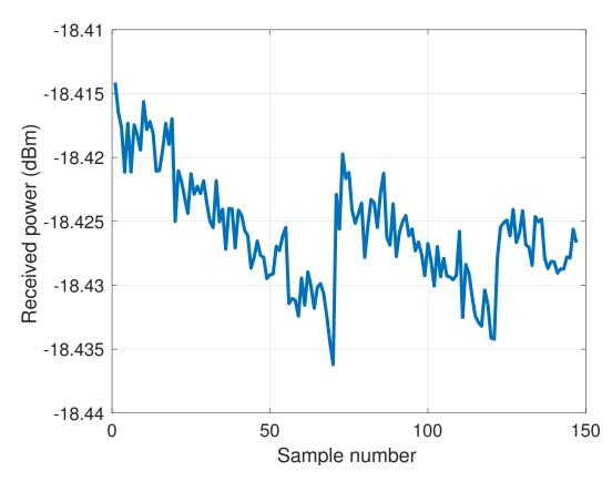
Figure 3.13: Received power at the MVG SH-2000 antenna terminals, when excited by the central embedded element of a S-Band single layer FR4 microstrip array at 3 GHz, mounted on the UAV's gimbal. The gimbal's motors were mechanically blocked and both antennas were aligned along their broadside directions.
