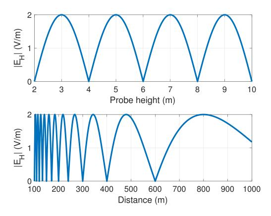
Figure 2.9: Normalized horizontal electric field magnitude at the AUT versus probe height (distance of 400 m and AUT height of 10 m) and distance (probe height of 6 m and AUT height of 10 m), in the presence of ground reflections.
