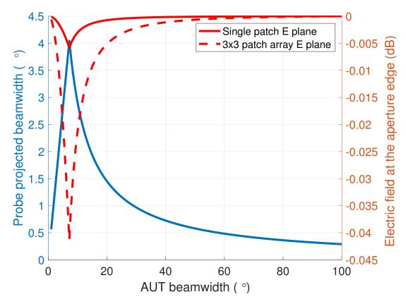
Figure 2.7: Projected beamwidth onto a uniform square aperture and electric field of a single patch antenna and a 3x3 uniform array of patch antennas ( $\frac{\lambda}{2}$  spacing) at its edge, versus its beamwidth. A minimum of 10 m for the FF distance was used.
