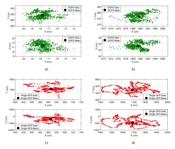
Figure 3.12: Comparison between RTK GPS position data and standard GPS position data for the Emlid Reach, for 2 datasets in static configuration. The top plot shows the x - y plane while the bottom plot shows the x - z plane. a) shows the RTK GPS dataset 1, b) shows the RTK GPS dataset 2, c) shows the GPS dataset 1, and d) shows the GPS dataset 2.
