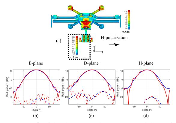
Figure 3.29: Effect of the UAV structure on the antenna pattern: all elements of a  $2 \times 2$  S-Band single layer FR4 microstrip array, horizontally polarized. (a) Current density on the probe and the UAV structure. (b) E-Plane antenna patterns with and without the UAV (red and blue respectively). (c) D-Plane antenna patterns with and without the UAV (red and blue respectively). (d) H-Plane antenna patterns with and without the UAV (red and blue respectively).
