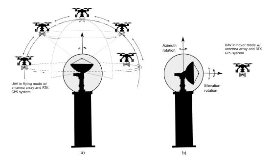
Figure 1.1: Illustration of the proposed system for in situ antenna characterization. a) The UAV flies around the radar system/antenna to carry out measurements. b) The drone hovers while the radar system/antenna rotates to carry out measurements.
