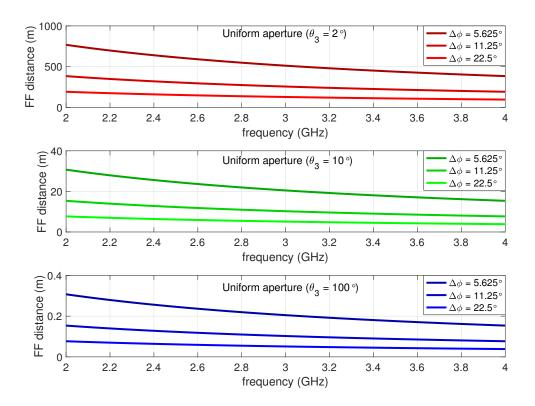
Figure 2.2: FF distance versus frequency for 3 given uniform square aperture antennas ( $\theta_3 = 2$ , 10 and 100°), and for 3 different phase error requirements ( $\Delta \phi = 5.625$ , 11.25 and 22.5°).
