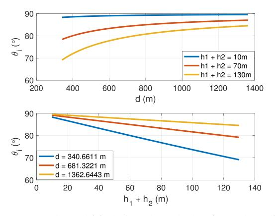
Figure B.3: Incident angle  $\theta_i$  for the ATD. The top plot shows  $\theta_i$  versus distance for 3 different values of  $h_1 + h_2$ , representing low, medium, and maximum. The bottom plot shows  $\theta_i$  versus  $h_1 + h_2$  for the 3 different values of the measurement distance, once the FF distance, twice the FF distance, and four times the FF distance.
