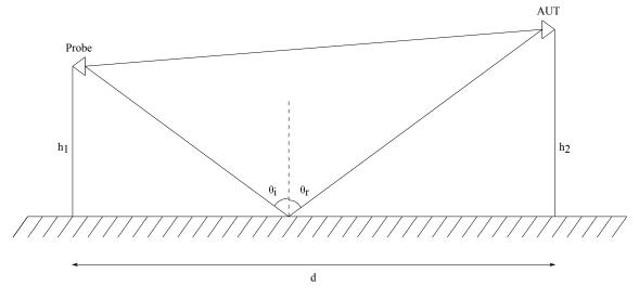
Figure 2.8: Propagation model between the probe and the AUT for FF measurements.
