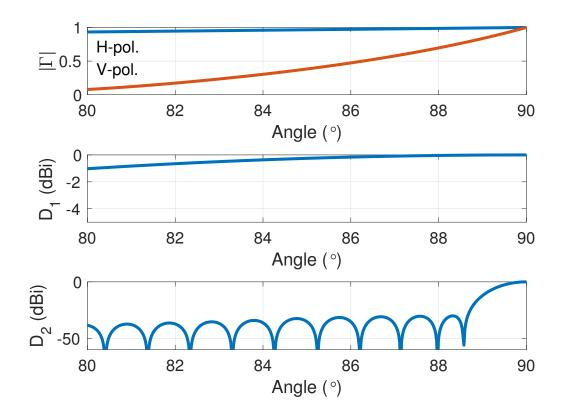
Figure 3.7: Parameters that influence the ground reflections for a 1° 3 dB beamwidth and 30 dB sidelobe-level weather radar versus a representative range of incident angles. The top plot is the reflection coefficient for H- and V-polarizations, the middle plot is the probe directivity, and the bottom plot is the radar directivity.
