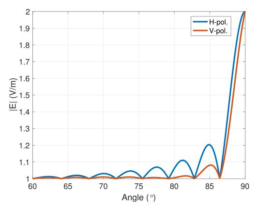
Figure 3.10: Maximum amplitude of the total electric field received at the 5G antenna versus a representative range of incident angles, for both H- and V-polarizations.
