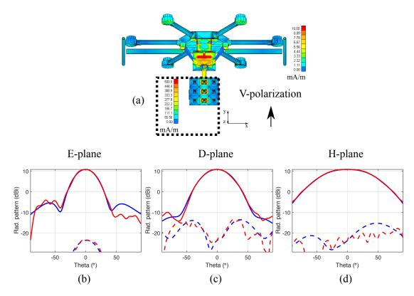
Figure 3.26: Effect of the UAV structure on the antenna pattern: central column of a  $3 \times 3$  S-Band single layer FR4 microstrip array, vertically polarized. (a) Current density on the probe and the UAV structure. (b) E-Plane antenna patterns with and without the UAV (red and blue respectively). (c) D-Plane antenna patterns with and without the UAV (red and blue respectively). (d) H-Plane antenna patterns with and without the UAV (red and blue respectively).
