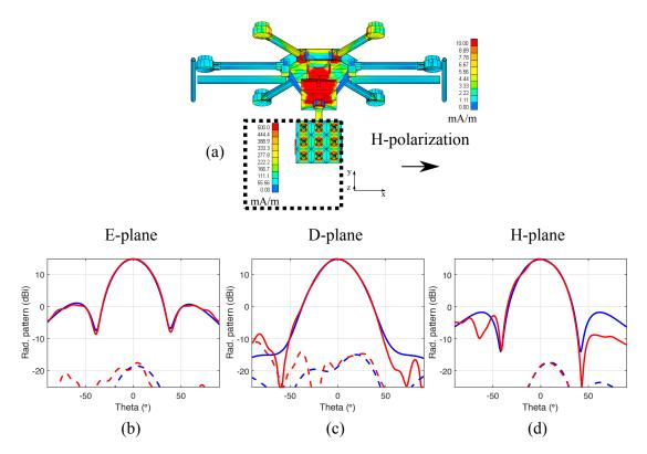
Figure 3.27: Effect of the UAV structure on the antenna pattern: all elements of a  $3 \times 3$  S-Band single layer FR4 microstrip array, horizontally polarized. (a) Current density on the probe and the UAV structure. (b) E-Plane antenna patterns with and without the UAV (red and blue respectively). (c) D-Plane antenna patterns with and without the UAV (red and blue respectively). (d) H-Plane antenna patterns with and without the UAV (red and blue respectively).
