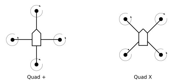
Figure 4.4: The two most popular frame types for the quadcopter: + and X frames. The direction of rotation for each motor is also indicated—Clockwise(CW) and Counter-Clockwise (CCW).
