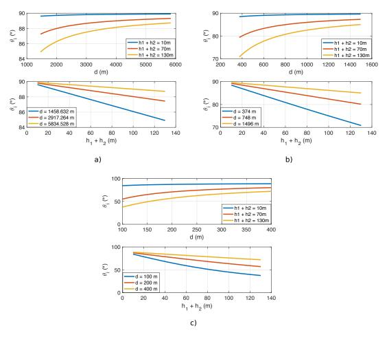
Figure 3.6: Incident angle  $\theta_i$  for the WSR88-D, a), RaXPol, b), and a 5G base station antenna, c). The top plot shows  $\theta_i$  versus distance for 3 different values of  $h_1 + h_2$ , representing low, medium, and maximum. The bottom plot shows  $\theta_i$  versus  $h_1 + h_2$  for the 3 different values of the measurement distance, once the FF distance, twice the FF distance, and four times the FF distance.
