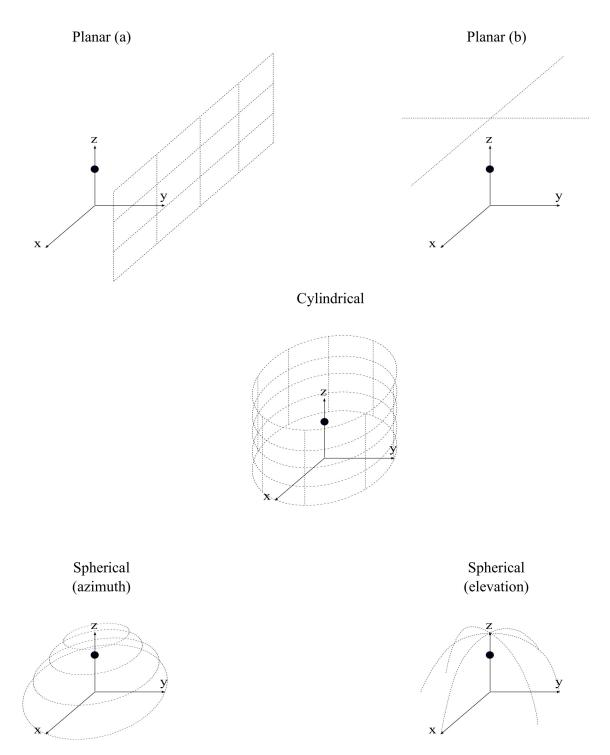
Figure 3.1: Illustration of the possible and common scan types with the UAV-based system. The first row illustrates planar scans, along x and z (a), and above the antenna in the x-y plane (b); the second cylindrical scans and the third spherical scans in both azimuth and elevation.
