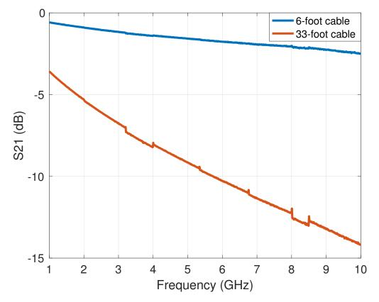
Figure 5.5: The losses versus frequency for both cables: 6-foot (blue) and 33-foot (red).
