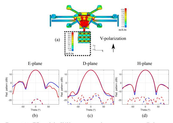
Figure 3.28: Effect of the UAV structure on the antenna pattern: all elements of a  $3\times3$  S-Band single layer FR4 microstrip array, vertically polarized. (a) Current density on the probe and the UAV structure. (b) E-Plane antenna patterns with and without the UAV (red and blue respectively). (c) D-Plane antenna patterns with and without the UAV (red and blue respectively). (d) H-Plane antenna patterns with and without the UAV (red and blue respectively).
