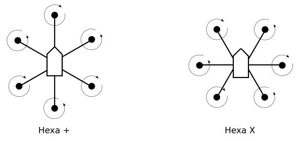
Figure 4.5: The two most popular frame types for the hexacopter: + and X frames. The direction of rotation for each motor is also indicated—Clockwise(CW) and Counter-Clockwise (CCW).
