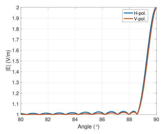
Figure 3.8: Maximum amplitude of the total electric field received at the radar versus a representative range of incident angles, for both H- and V-polarizations.
