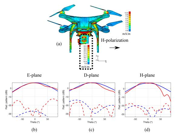
Figure 3.17: Effect of the DJI Phantom 3 structure on the antenna pattern: single cell of a single layer FR4 microstrip array, horizontally polarized. (a) Current density on the probe and the UAV structure. (b) E-Plane antenna patterns with and without the UAV (red and blue respectively). (c) D-Plane antenna patterns with and without the UAV (red and blue respectively). (d) H-Plane antenna patterns with and without the UAV (red and blue respectively).
