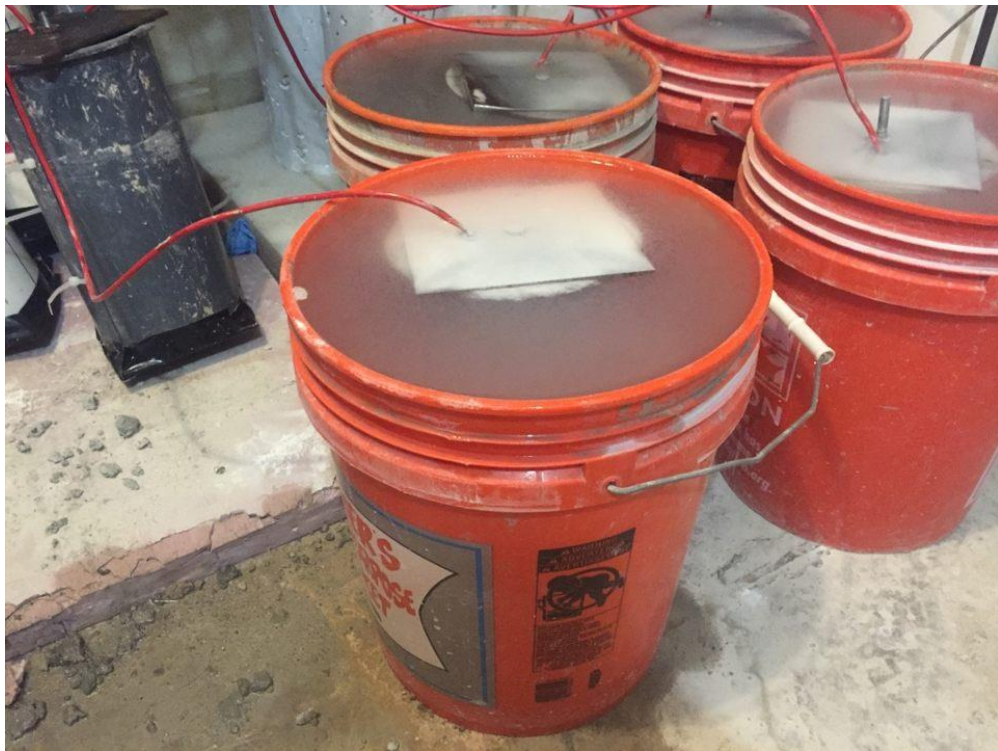
Figure 25, Wet Curing of 6"x12"
