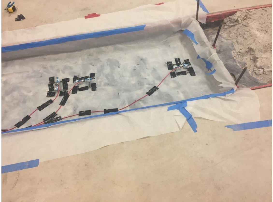
Figure 18, Setup for Slab with Fibers or Control Slab
