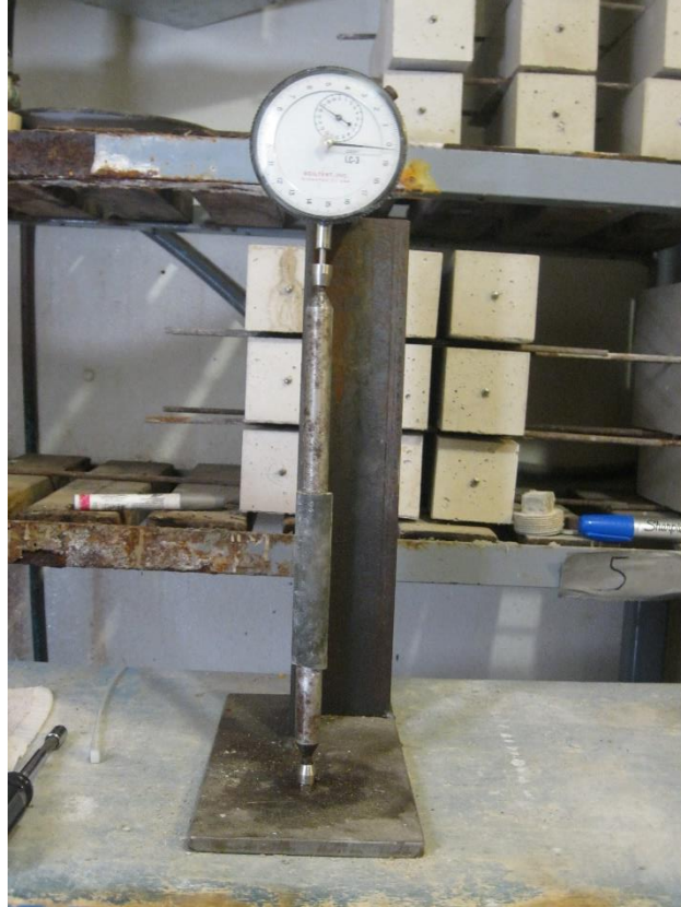
Figure 22, C-878 Length Comparator
