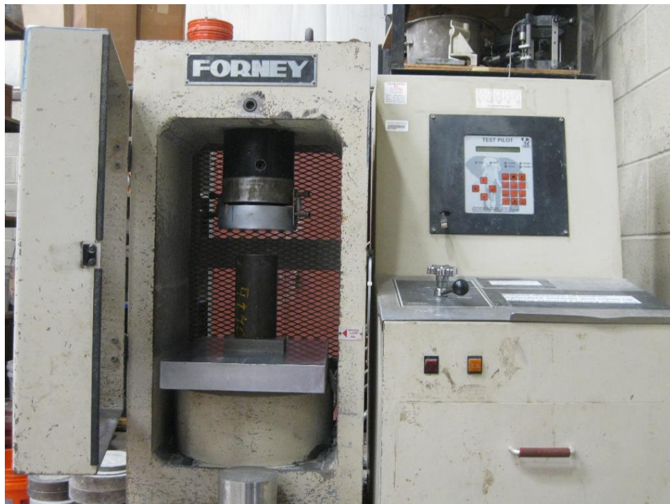
Figure 19, Setup for C-39 Test
