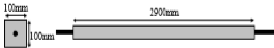
Figure 3, Setup of Tension Stiffening Experiment (Hosoda and Kishi 2003)
