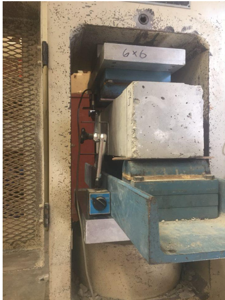
Figure 26, Load Deflection Test Setup for the Modified MOR Test
