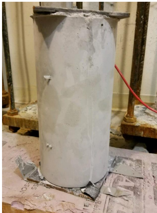
Figure 24, 6"x12" Restrained Cylinder
