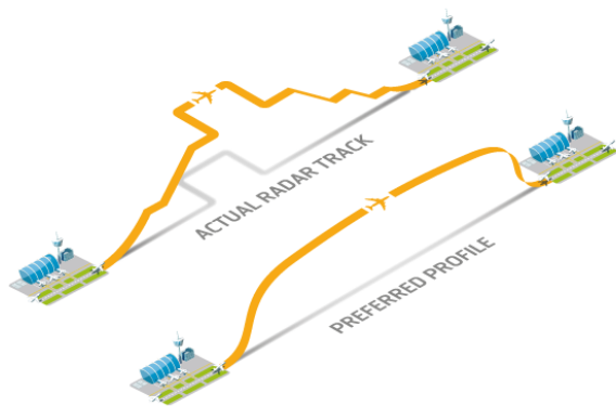
Figure XXVI. RADAR vs. Trajectory Based Operations (TBO) Adapted from "Managing Real Time Fuel Efficiency" by National Air Traffic Systems (2016b) published by FloSys - Flight Optimization System.
