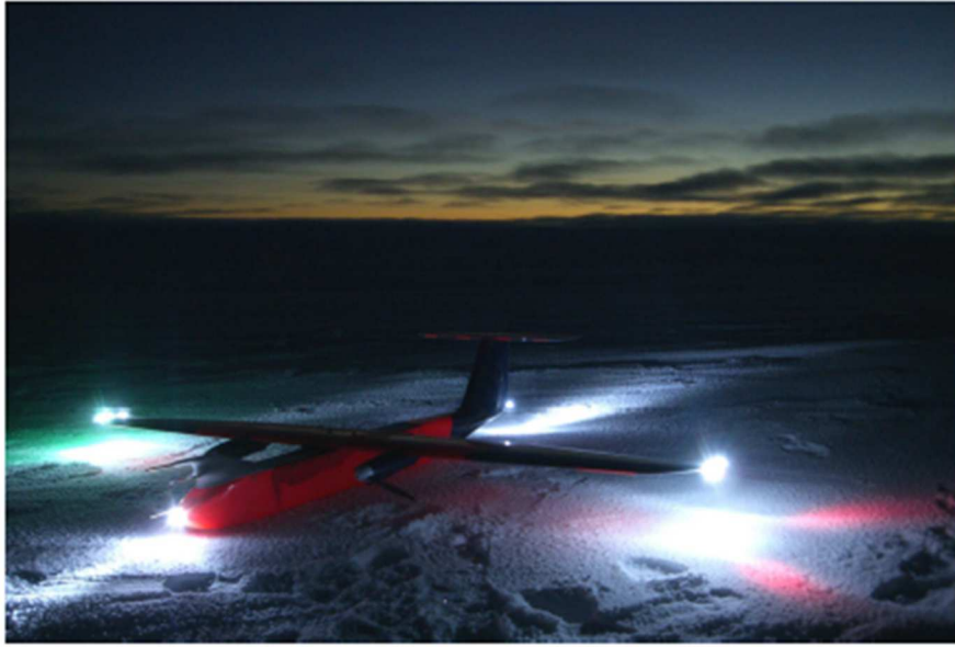
Figure 3-11 : M2AV taking turbulence data in Antarctica [1].
