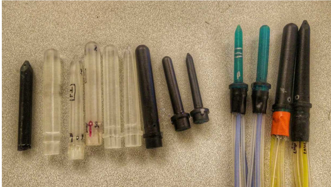
Figure 4-1 : Progression of 3D printed probes. Old-to-new from left to right. 3D printing of left 6 probes in the FDM method, and the 7 probes to the right are manufactured by SLA tough resin.
