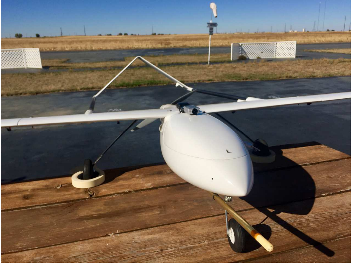
Figure 1-2 : 3D printed 5-hole probe mounted on NCAR's Albatross platform [5].
