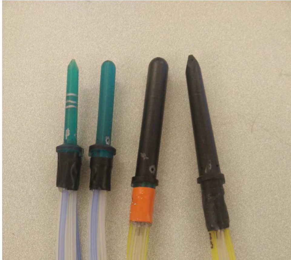
Figure 4-2 : Scaled down pyramid and hemisphere probes (left) compared to the large hemisphere and pyramid probes (right).
