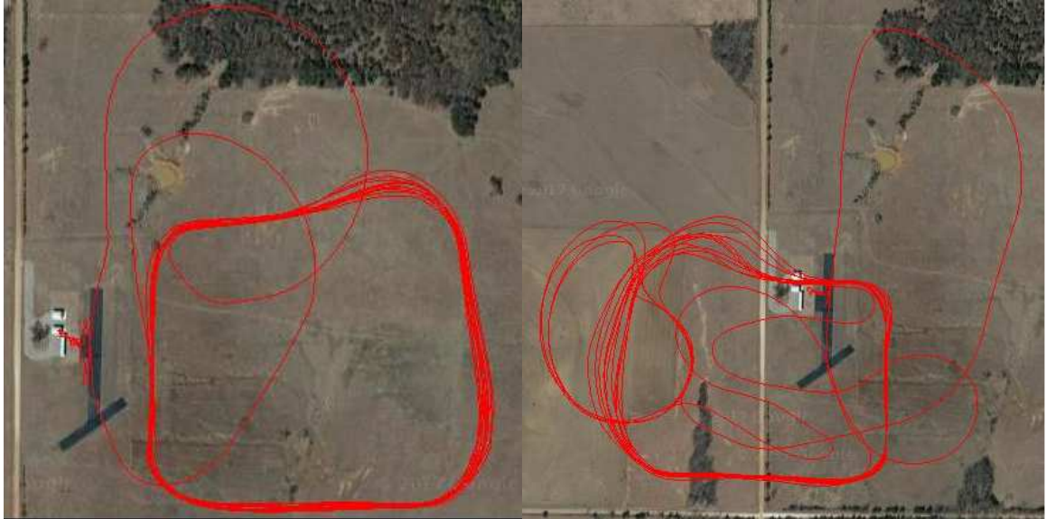
Figure 6-2 : Flight Paths for 2 flight days with varying wind conditions. Left image shows minimal overshoot. Overshoots in waypoints (right) resulting from greater wind conditions and autopilot gain tuning.
