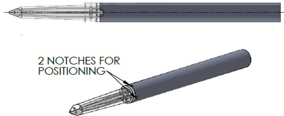
Figure 4-10 : Boom and Probe notch mating.
