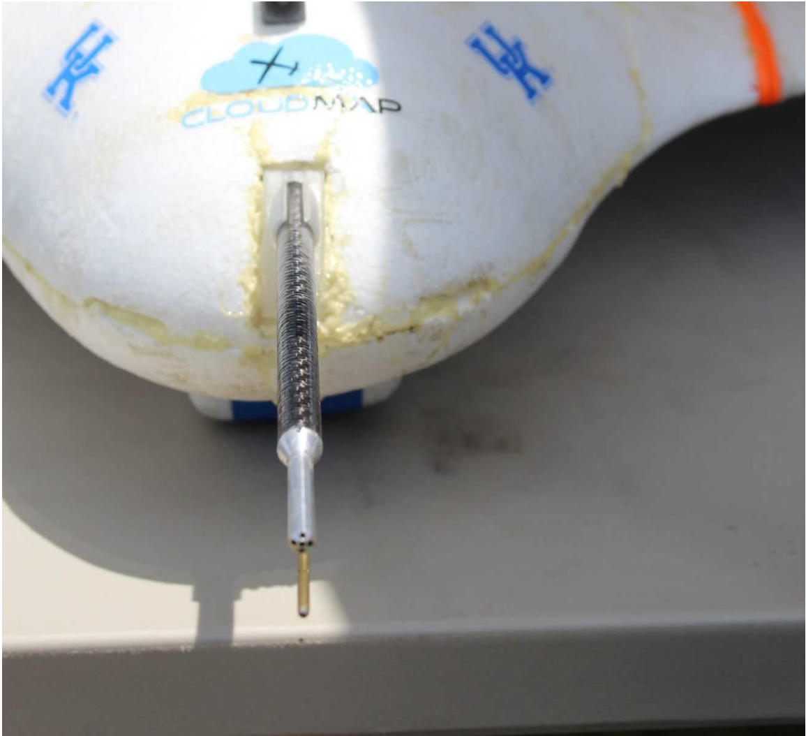
Figure 1-3 : Machined 5-hole probe mounted on University of Kentucky's X-8 platform.
