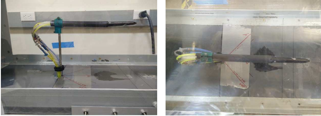
Figure 4-8 : Pyramid 5-hole probe side and top views
