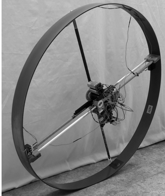
Figure 1.1: The OSU rolling robot has a mass of 0.950 kg with a perimeter of 2.095 m.
