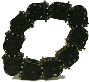
Figure 2.3: The CKBot roller developed by Sastra et al. had ten individually motorized modules connected end-to-end in a loop. Image is from [6].
