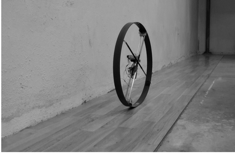
Figure 4.1: Roll track for the robot is a rectangular strip of laminate flooring, measuring 0.82 m by 9.70 m, that's installed on concrete.
