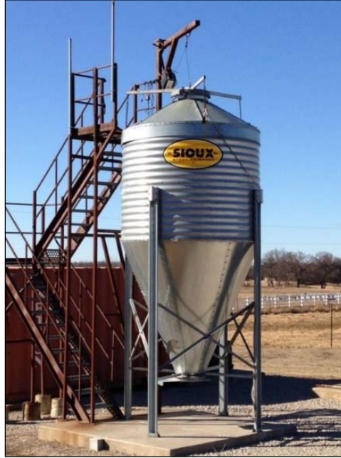
Figure 4.1. The 1.83 m (6 ft) diameter steel bin used during measurement of entrapment pressures.
