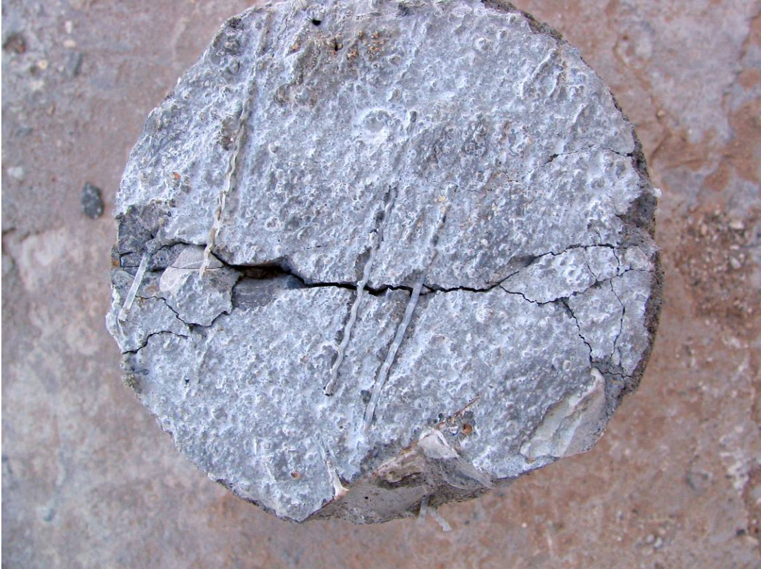
Figure 31: Fiber-reinforced concrete splitting tensile failure: ductile
