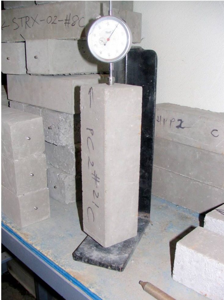
Figure 19: Unrestrained shrinkage test
