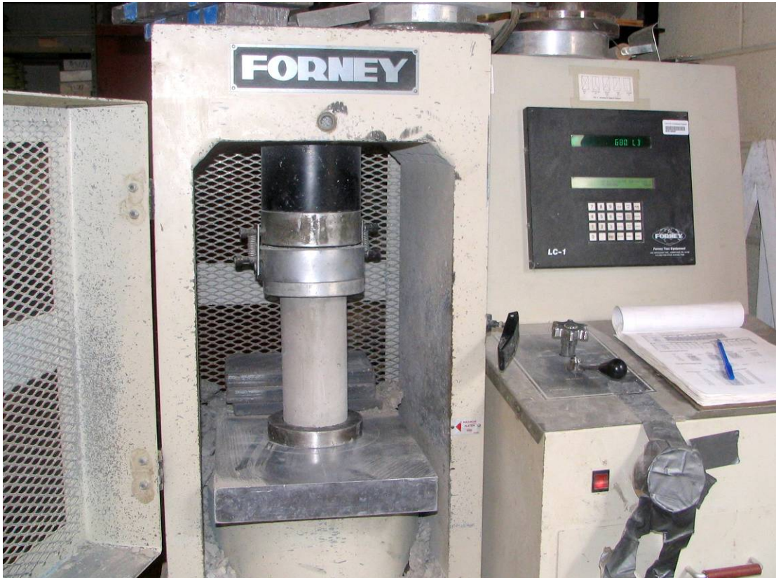
Figure 17: Compression test with Forney compression testing machine
