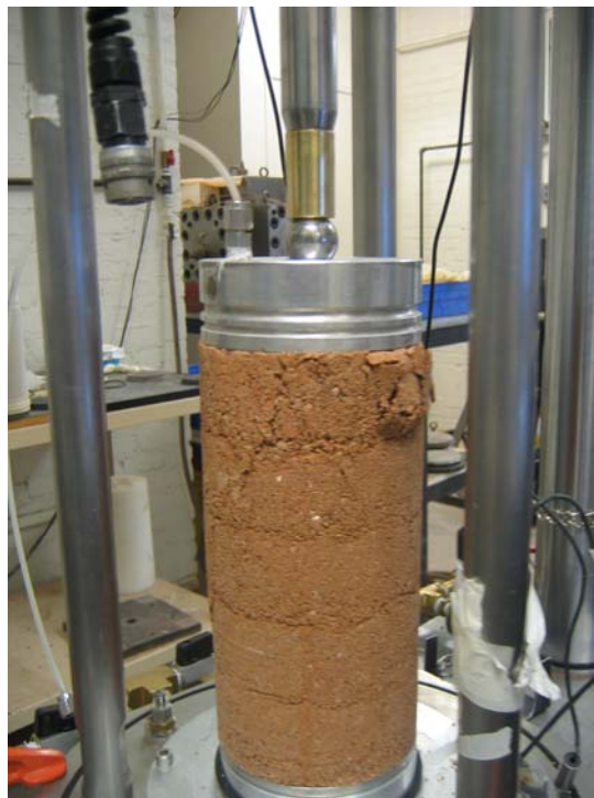
Figure 3.6 Specimen in MTS Frame for UCS Test
