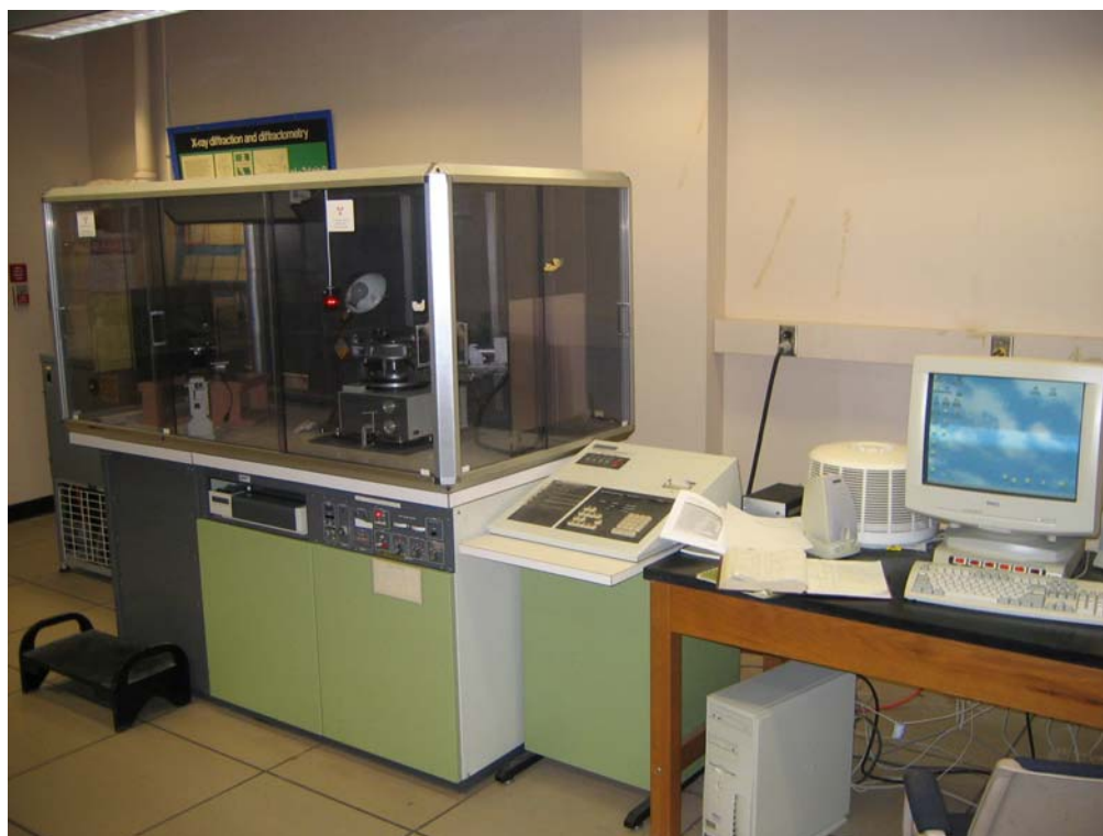
Figure 5.5 Rigaku D/Max X-ray Diffractometer
