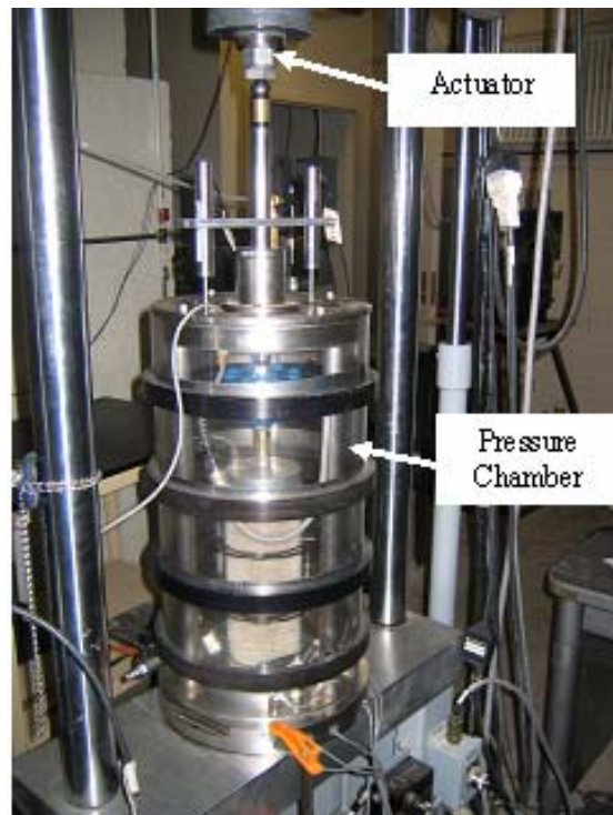
Figure 3.4 Setup for Resilient Modulus Test (with pressure chamber)
