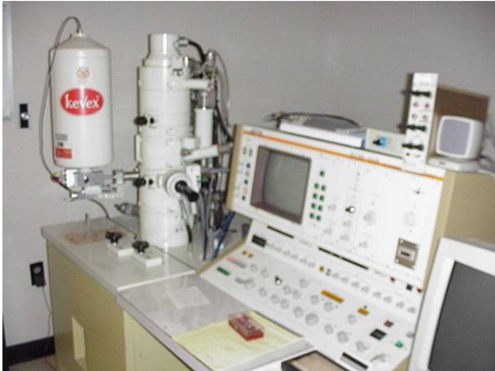
Figure 5.3 JEOL JSM 880 used for Scanning Electron Microscopy
