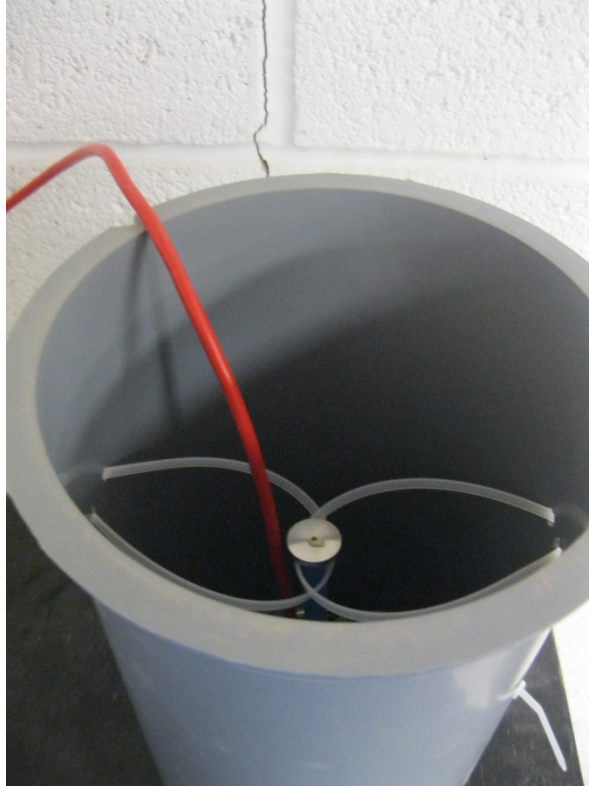
Figure 25: 6"x 12" Cylinder Equipped with VWSG for Unrestrained Expansion
