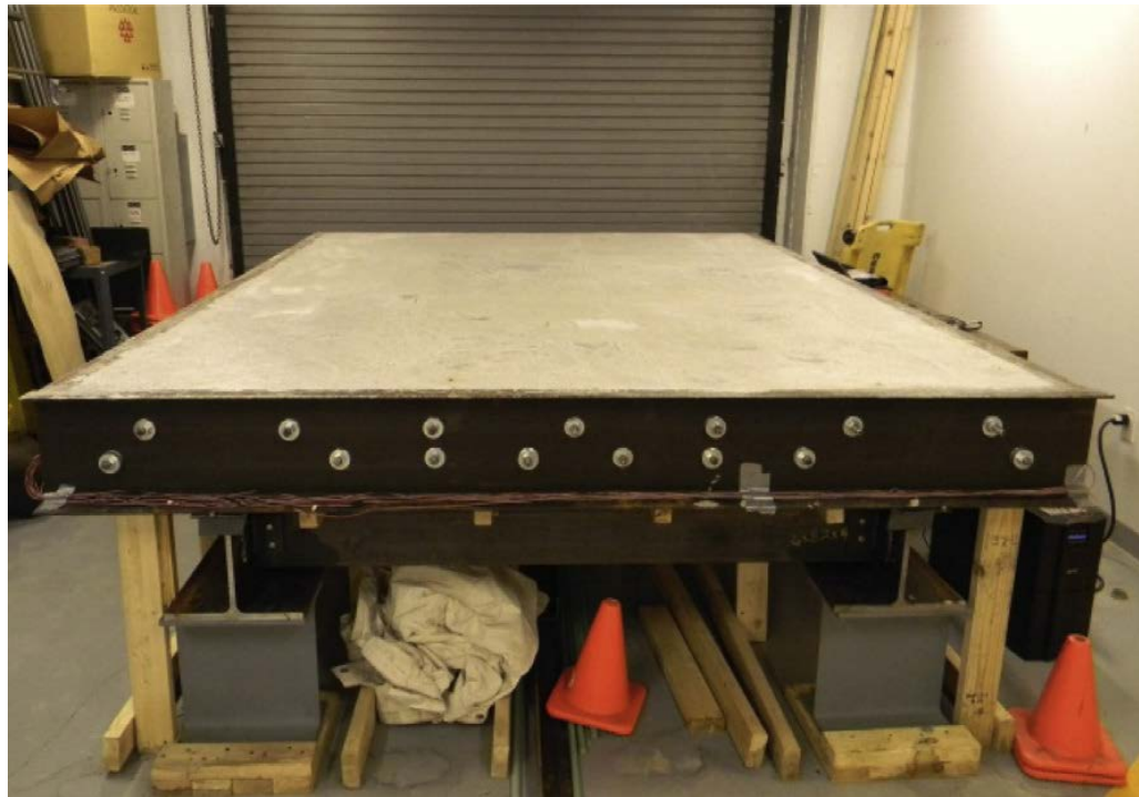
Figure 7: Experimental Bridge Deck with Concrete (Richardson et al., 2014)
