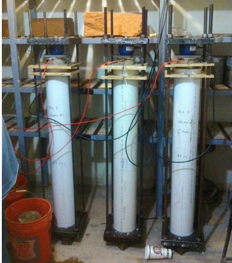
Figure 30: Curing Alternative 1, PVC Jackets with Cardboard Forms at Water Cure Stage (Seth Roswurm, 2013)
