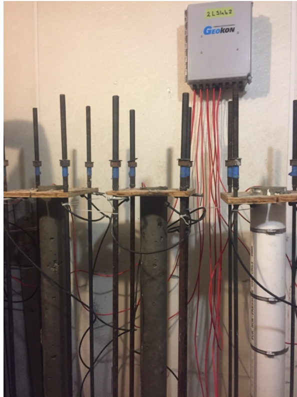
Figure 33: Curing Alternative 2, PVC Form with Hose Clamps at Form Stripping Stage
