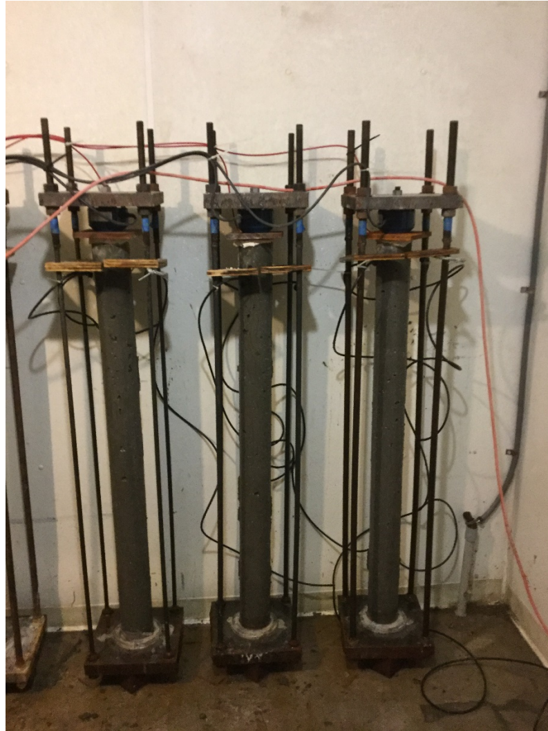
Figure 34: Restrained Columns Equipped with Sprinkler System for Wet Cure
