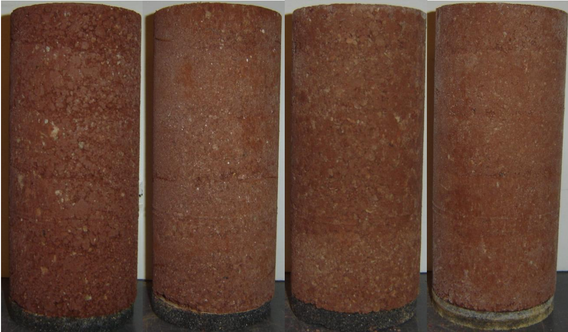
Figure C 5: Kingfisher Specimens Tested for M_r at the end of 0 Freeze-Thaw Cycles (From Left to Right: Raw, Lime, CFA, CKD)
