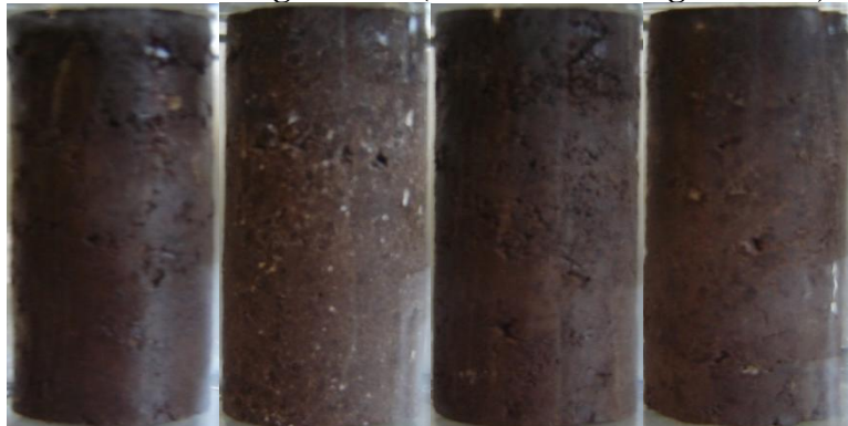
Figure B 15: Harvard Miniature Lomill Specimens Before 1 Wet-Dry Cycle. (From Left to Right: Raw, Lime, CFA, CKD)
