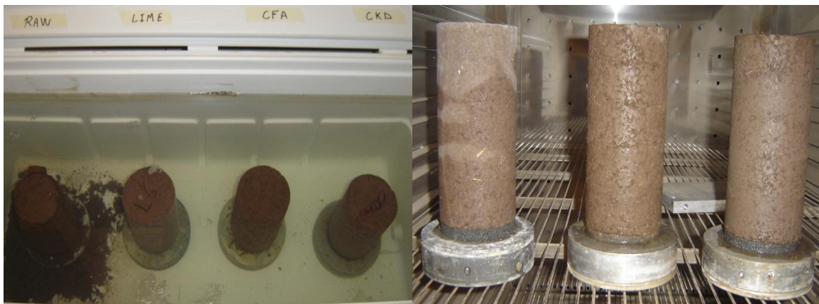
(a) (b) Figure 3.14: Specimens under Wetting Cycle at 0 hours (a) and During 42 hours Oven Drying (b)
