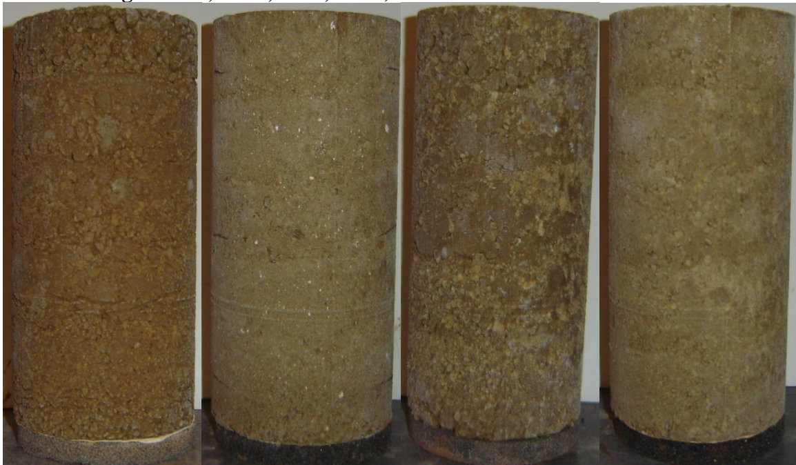
Figure D 10: Dennis Specimens Tested for M_r after 0 Wet-Dry Cycles (From Left to Right: Raw, Lime, CFA, CKD)
