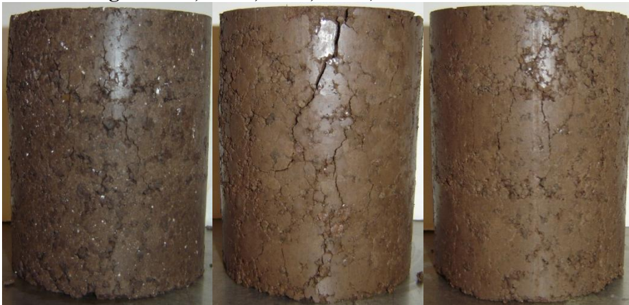
Figure F 8: Lomill Specimens After Vacuum Saturation at the End of UCS Test (From Left to Right: Lime, CFA, CKD)
