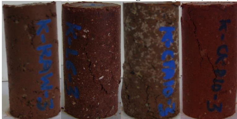
Figure A 9: Harvard Miniature Kingfisher Specimens at the End of 1 Freeze-Thaw Cycle After UCS. (From Left to Right: Raw, Lime, CFA, CKD)
