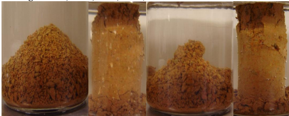
Figure 4.44: Carnasaw Specimens at the End of 5-Hour Soaking Period (From Left to Right: Raw, Lime, CFA, CKD)
