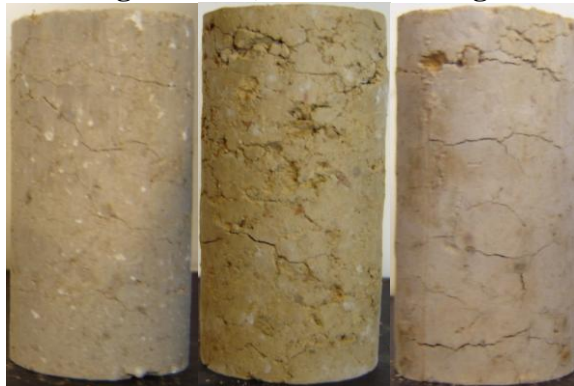
Figure B 11: Harvard Miniature Dennis Specimens After 1 Wet-Dry Cycle at the End of 42 Hours of Drying Period. (From Left to Right: Lime, CFA, CKD)
