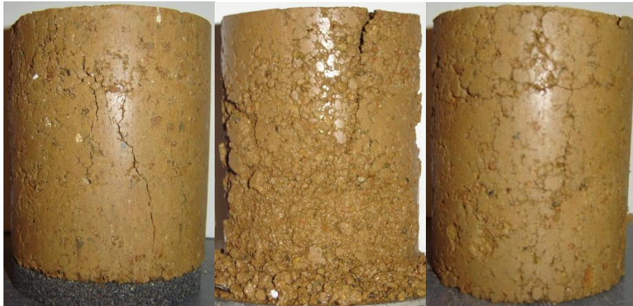
Figure F 4: Carnasaw Specimens After Vacuum Saturation at the End of UCS Test (From Left to Right: Lime, CFA, CKD)
