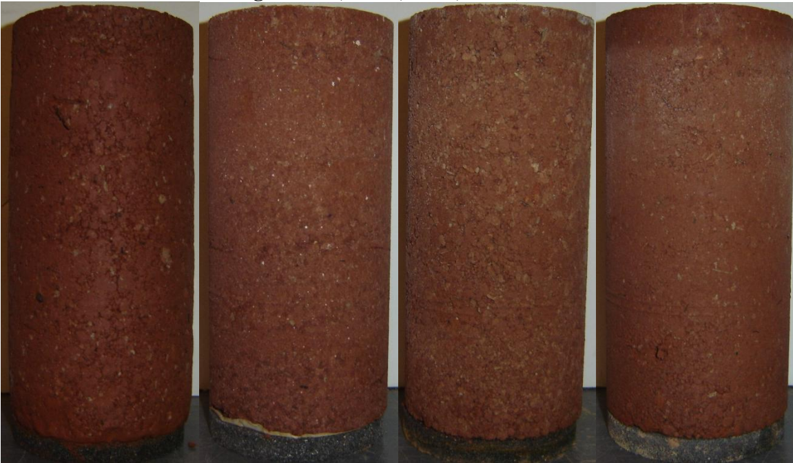
Figure C 6: Kingfisher Specimens Tested for M_r at the end of 1 Freeze-Thaw Cycle (From Left to Right: Raw, Lime, CFA, CKD)
