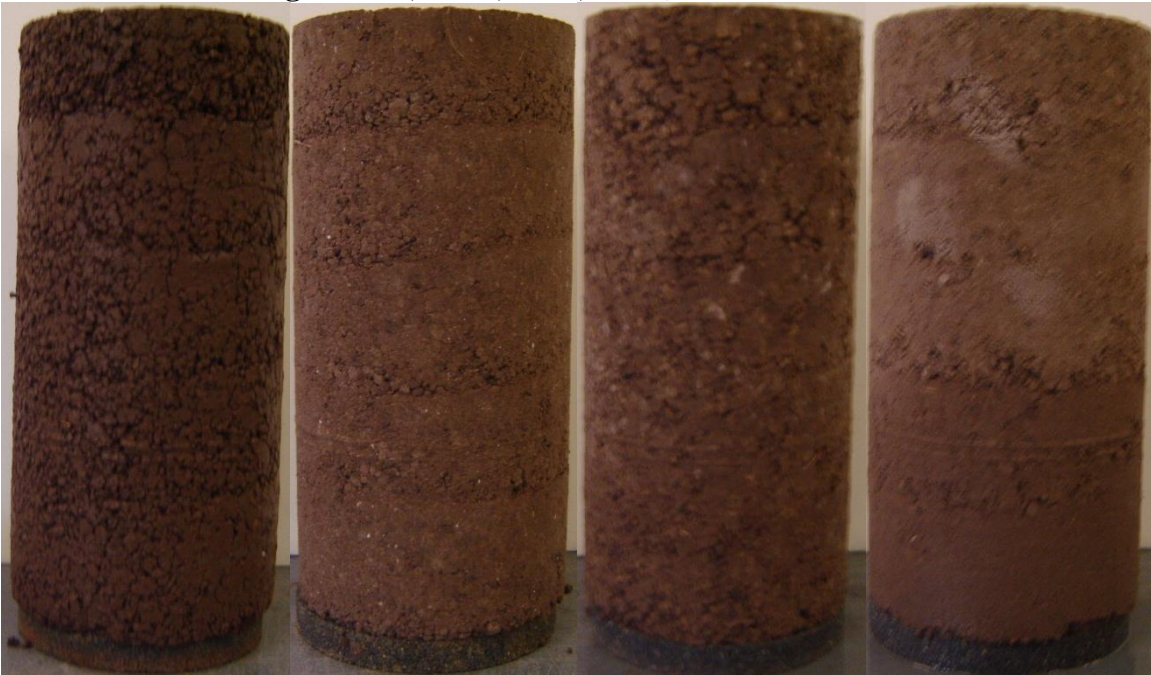
Figure C 12: Dennis Specimens Tested for M_r at the End of 1 Freeze-Thaw Cycle (From Left to Right: Raw, Lime, CFA, CKD)
