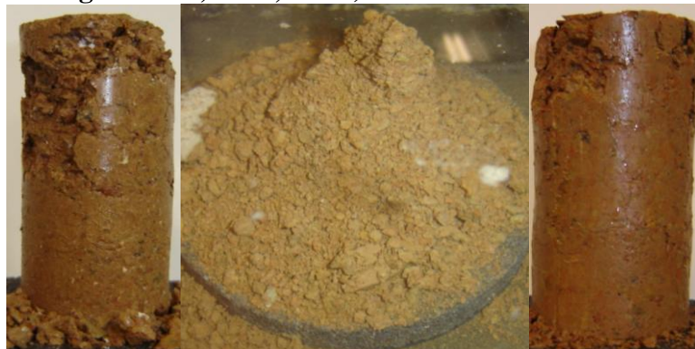
Figure B 8: Harvard Miniature Carnasaw Specimens After 1 Wet-Dry Cycle at the End of 5 Hours of Soaking Period. (From Left to Right: Lime, CFA, CKD)
