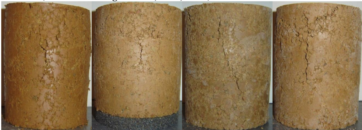
Figure F 3: Carnasaw Specimens Before Vacuum Saturation at the End of UCS test (From Left to Right: Raw, Lime, CFA, CKD)
