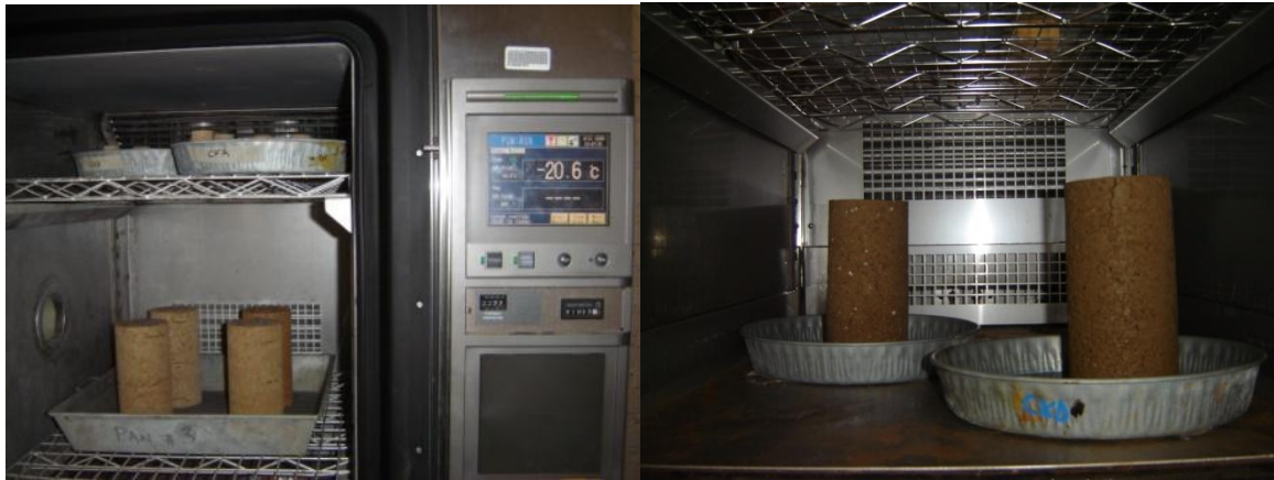
(a) (b) Figure 3.13: Resilient Modulus Specimens under (a) Freezing and (b) Thawing
