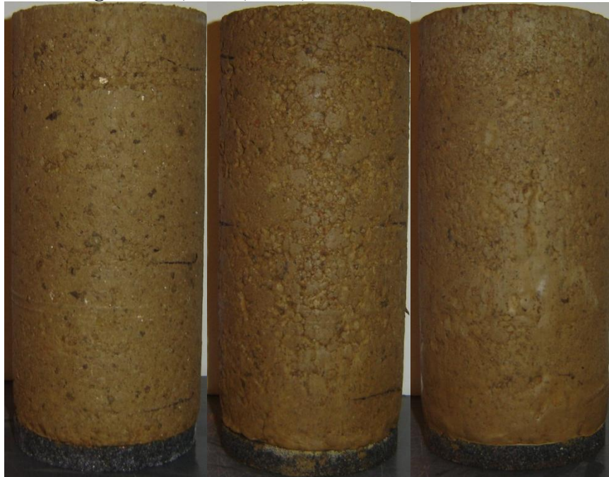
Figure C 10: Dennis Specimens Tested for M_r at the End of 4 Freeze-Thaw Cycles (From Left to Right: Lime, CFA, CKD)
