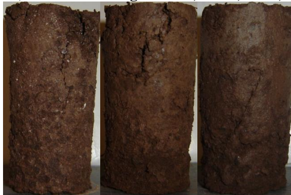
Figure A 30: Harvard Miniature Lomill Specimens at the End of 12 Freeze-Thaw Cycles After UCS. (From Left to Right: Raw, Lime, CFA, CKD)
