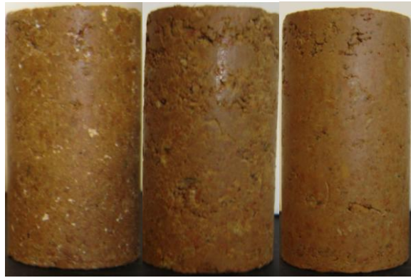
Figure B 7: Harvard Miniature Carnasaw Specimens Before 1 Wet-Dry Cycle. (From Left to Right: Lime, CFA, CKD)
