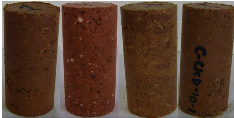
Figure A 13: Harvard Miniature Carnasaw Specimens at the End of 0 Freeze-Thaw Cycles Before UCS. (From Left to Right: Raw, Lime, CFA, CKD)
