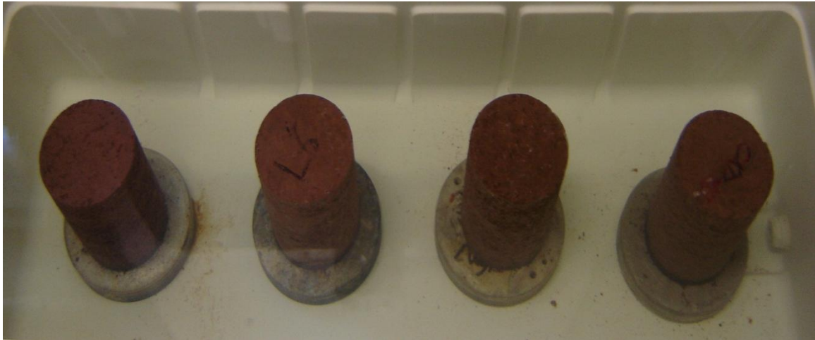
Figure D 15: Lomill Specimens in Water during 1 Wet-Dry Cycle (From Left to Right: Raw, Lime, CFA, CKD)
