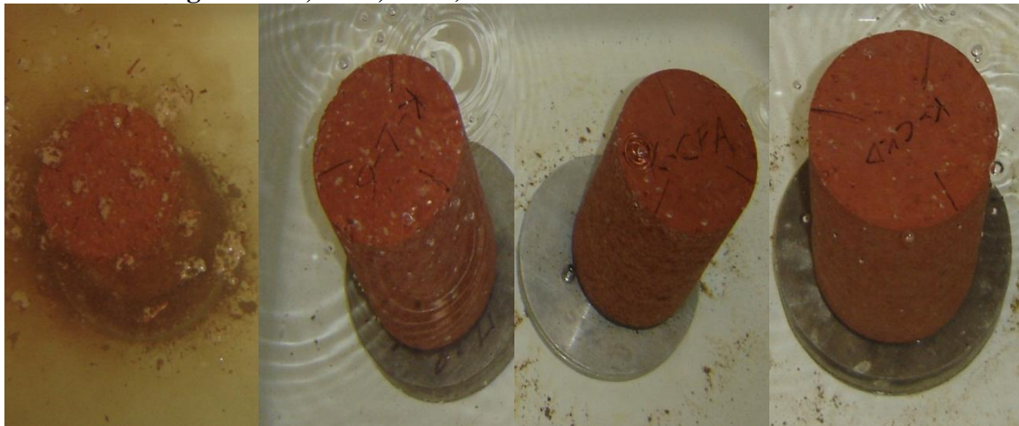
Figure D 4: Kingfisher Specimens in Water During 1 Wet-Dry Cycle (From Left to Right: Raw, Lime, CFA, CKD)
