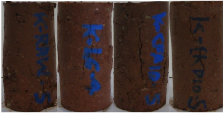
Figure A 10: Harvard Miniature Kingfisher Specimens at the End of 4 Freeze-Thaw Cycles After UCS. (From Left to Right: Raw, Lime, CFA, CKD)
