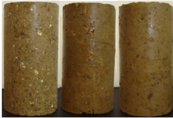
Figure B 10: Harvard Miniature Dennis Specimens After 1 Wet-Dry Cycle at the End of 5 Hours of Soaking Period. (From Left to Right: Lime, CFA, CKD)
