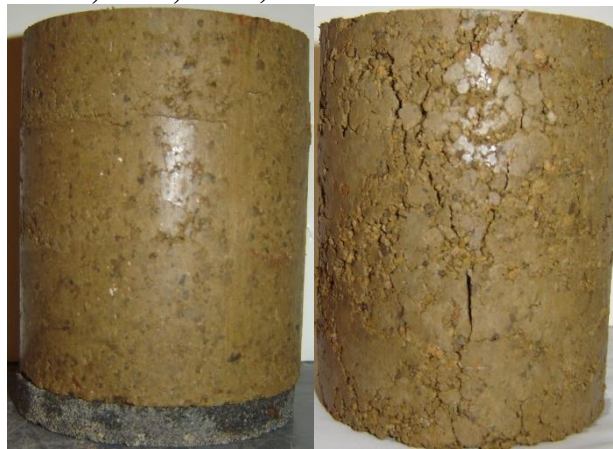
Figure 4.55: Dennis Specimens after Vacuum Saturation after UCS Test (From Left to Right: Lime, CFA)
