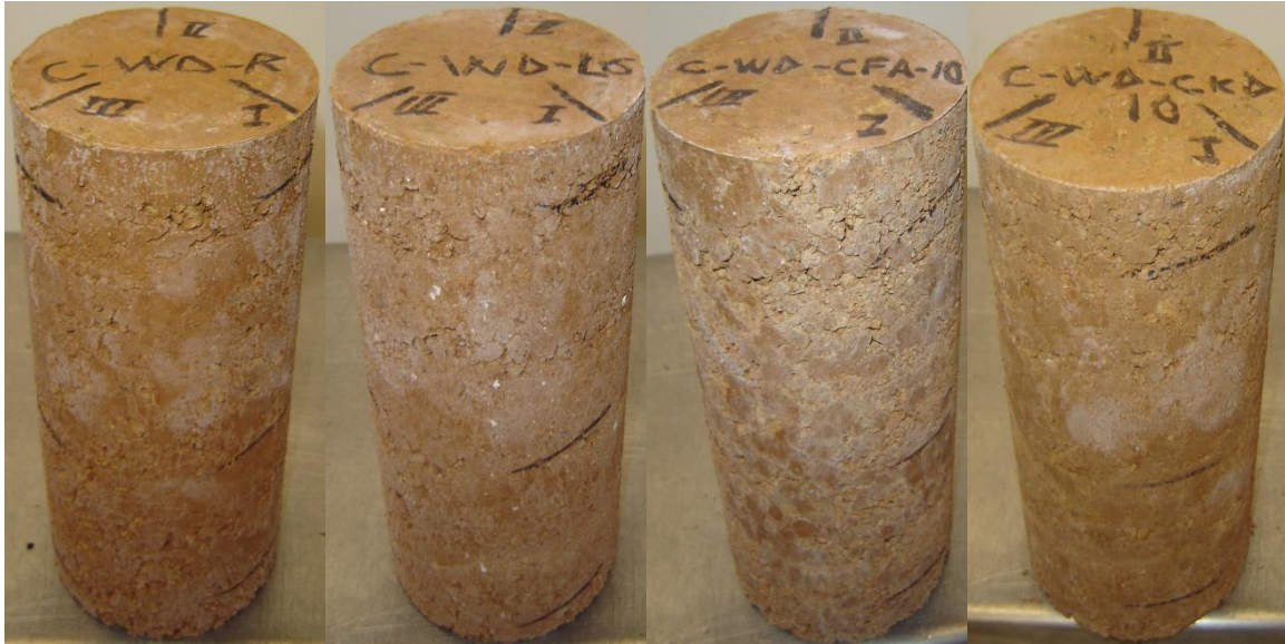
Figure D 7: Carnasaw Specimens Tested for M_r at the End of 0 Wet-Dry Cycles (From Left to Right: Raw, Lime, CFA, CKD)
