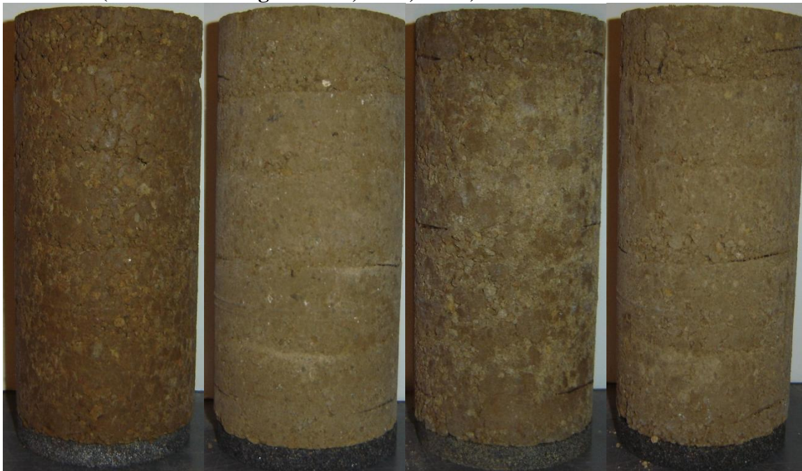
Figure C 8: Dennis Specimens Tested for M_r at the end of 0 Freeze-Thaw Cycles (From Left to Right: Raw, Lime, CFA, CKD)
