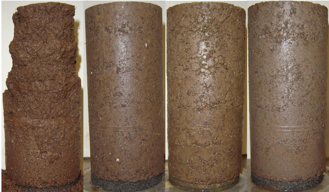
Figure D 16: Lomill Specimens After 5 Hour Soaking During 1 Wet-Dry Cycle (From Left to Right: Raw, Lime, CFA, CKD)
