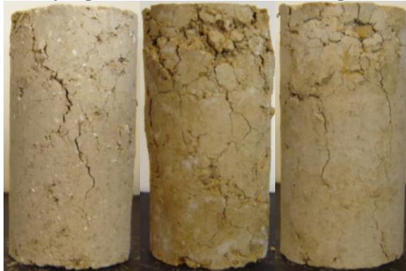
Figure B 12: Harvard Miniature Dennis Specimens After 1 Wet-Dry Cycle After UCS. (From Left to Right: Lime, CFA, CKD)
