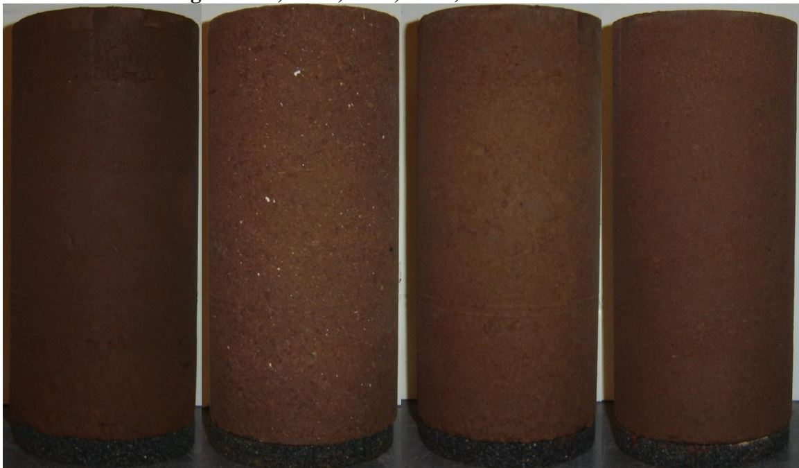
Figure C 2: Port Specimens Tested for M_r at the End of 1 Freeze-Thaw Cycle (From Left to Right: Raw, Lime, CFA, CKD)
