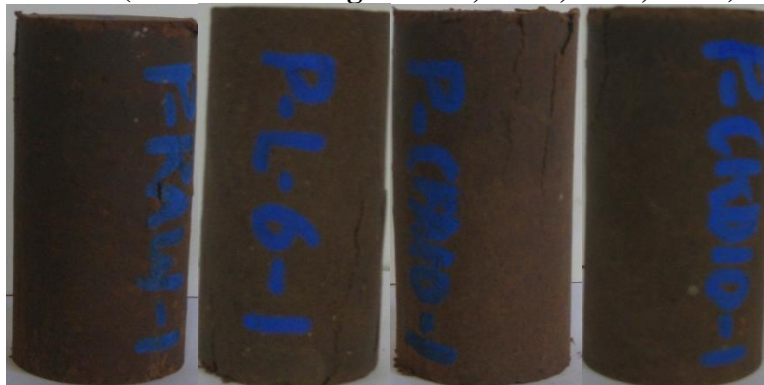
Figure A 2: Harvard Miniature Port Specimens at the End of 0 Freeze-Thaw Cycles After UCS (From Left to Right: Raw, Lime, CFA, CKD)
