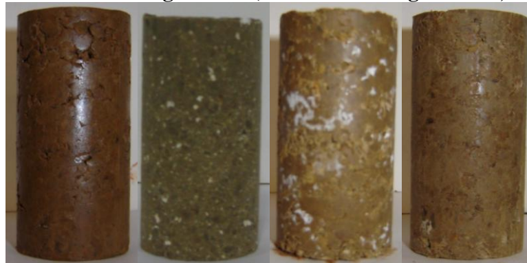
Figure B 9: Harvard Miniature Dennis Specimens Before 1 Wet-Dry Cycle. (From Left to Right: Raw, Lime, CFA, CKD)
