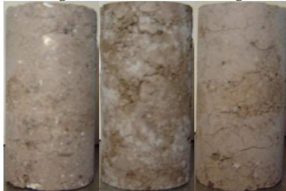
Figure B 17: Harvard Miniature Lomill Specimens After 1 Wet-Dry Cycle at the End of 42 Hours of Drying Period. (From Left to Right: Lime, CFA, CKD)
