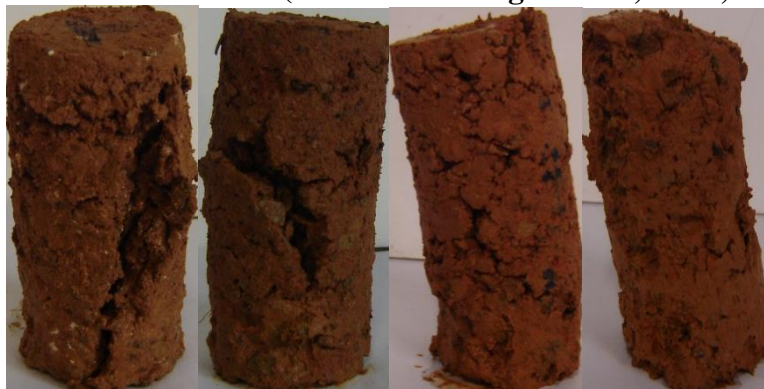
Figure 4.13: Harvard Miniature Carnasaw Specimens at the End of 12 Freeze-Thaw Cycles After UCS Test (From Left to Right: Raw, Lime, CFA, CKD)
