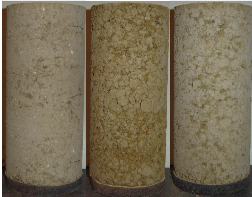
Figure D 12: Dennis Specimens Tested for M_r after 1 Wet-Dry Cycle (From Left to Right: Lime, CFA, CKD)
