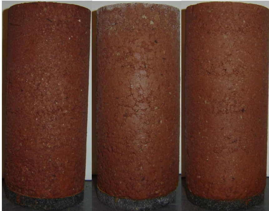
Figure C 7: Kingfisher Specimens Tested for M_r at the end of 4 Freeze-Thaw Cycles (From Left to Right: Lime, CFA, CKD)
