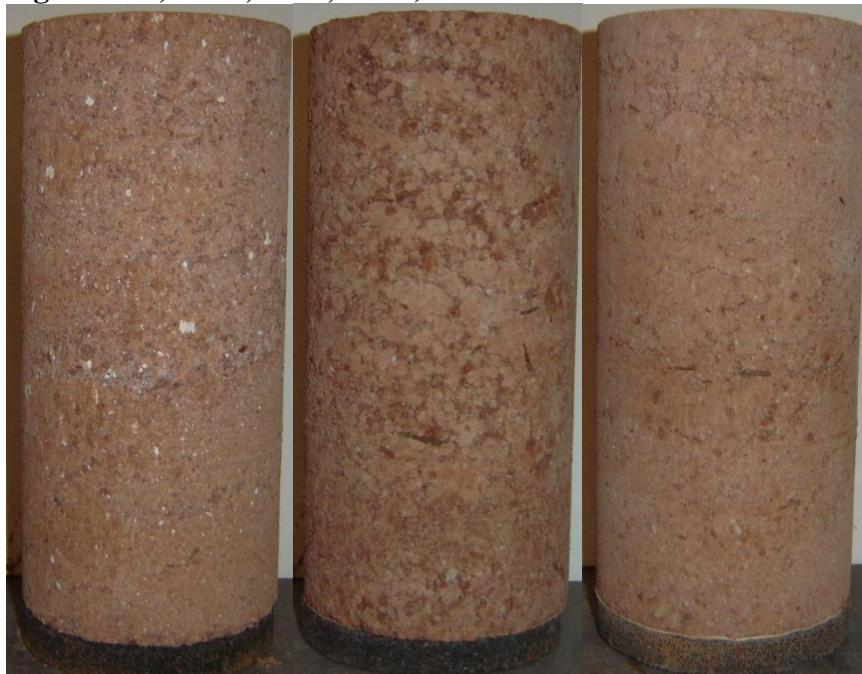
Figure D 2: Kingfisher Specimens Tested for M_r After 1 Wet-Dry Cycle (From Left to Right: Lime, CFA, CKD)
