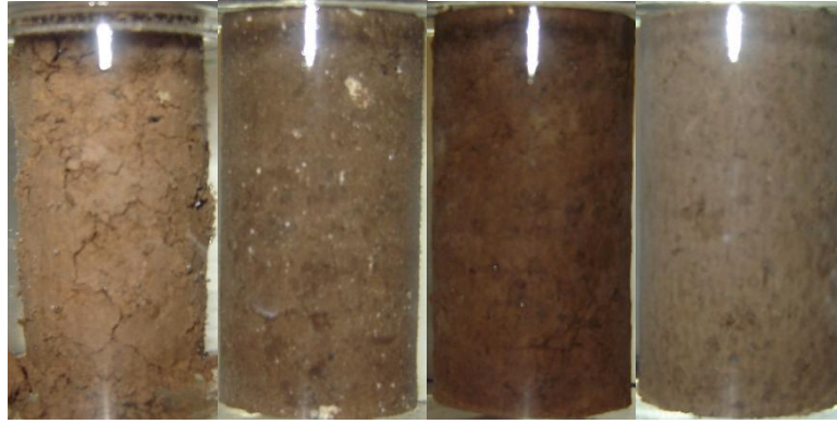
Figure B 16: Harvard Miniature Lomill Specimens After 1 Wet-Dry Cycle at the End of 5 Hours of Soaking Period. (From Left to Right: Raw, Lime, CFA, CKD)
