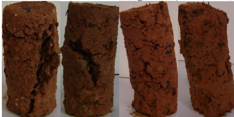
Figure A 18: Harvard Miniature Carnasaw Specimens at the End of 12 Freeze-Thaw Cycles After UCS. (From Left to Right: Raw, Lime, CFA, CKD)
