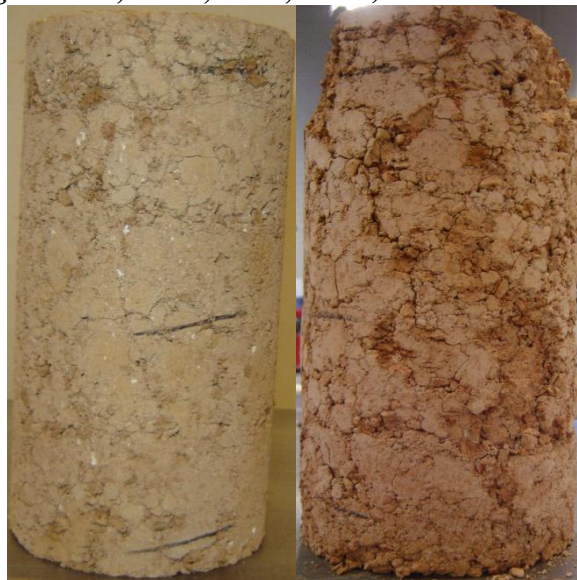
Figure D 8: Carnasaw Specimens Tested for M_r After 1 Wet-Dry Cycle (From Left to Right: Lime, CKD)
