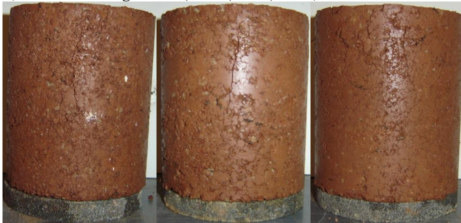
Figure F 2: Kingfisher Specimens After Vacuum Saturation at the End of UCS Test (From Left to Right: Lime, CFA, CKD)
