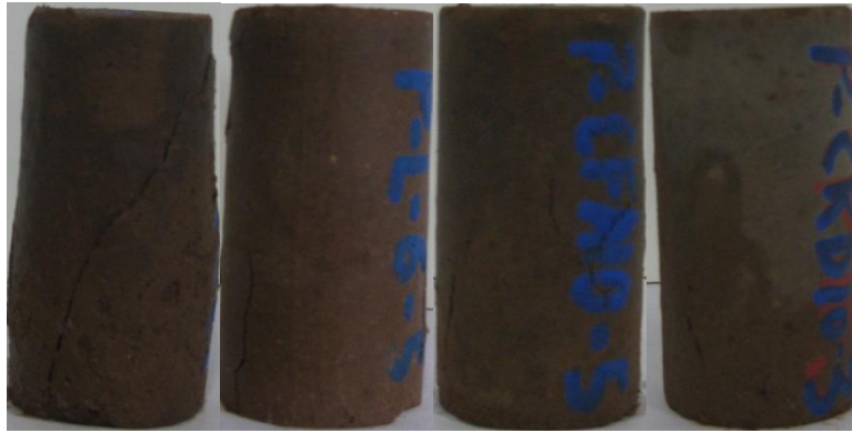
Figure A 4: Harvard Miniature Port Specimens at the End of 4 Freeze-Thaw Cycles After UCS (From Left to Right: Raw, Lime, CFA, CKD)
