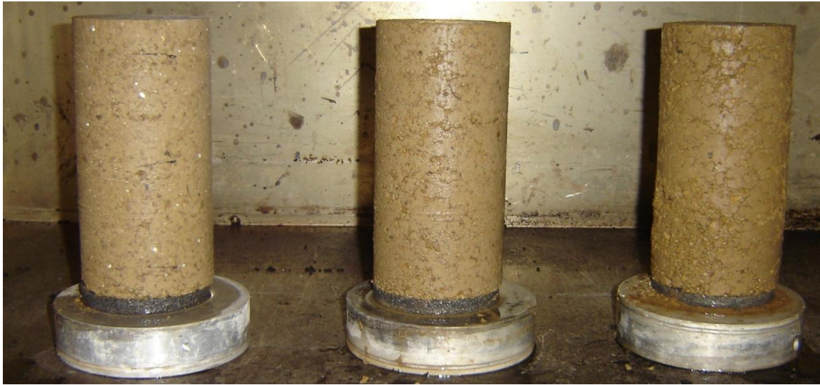
Figure D 13: Dennis Specimens in Oven during 1 Wet-Dry Cycle (From Left to Right: Lime, CFA, CKD)
