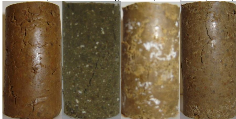
Figure A 20: Harvard Miniature Dennis Specimens at the End of 0 Freeze-Thaw Cycles After UCS. (From Left to Right: Raw, Lime, CFA, CKD)
