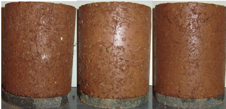
Figure 4.53: Kingfisher Specimens After Vacuum Saturation After UCS Test (From Left to Right: Lime, CFA, CKD)
