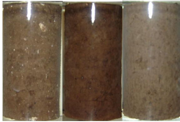
Figure 4.23: Harvard Miniature Lomill Specimens After 1 Wet-Dry Cycle at the End of 5- Hour Soaking Period (From Left to Right: Lime, CFA, CKD)
