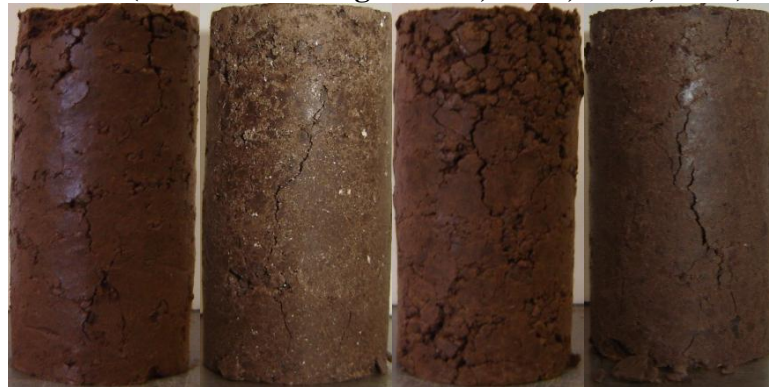
Figure A 27: Harvard Miniature Lomill Specimens at the End of 1 Freeze-Thaw Cycle After UCS. (From Left to Right: Raw, Lime, CFA, CKD)
