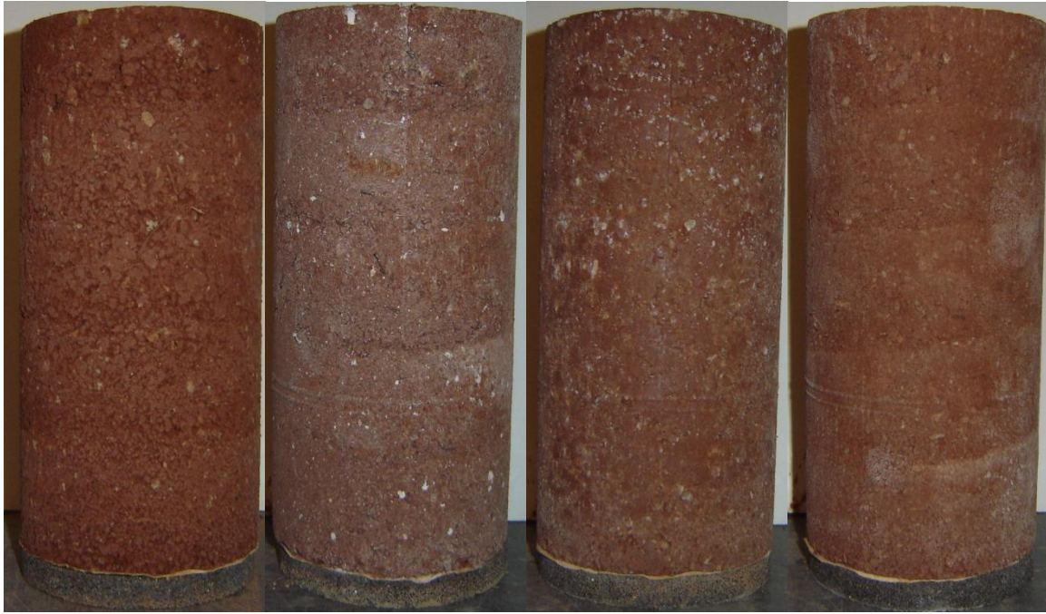
Figure D 1: Kingfisher Specimens Tested for M_r after 0 Wet-Dry Cycles (From Left to Right: Raw, Lime, CFA, CKD)
