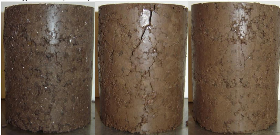
Figure 4.56: Lomill Specimens After Vacuum Saturation After UCS Test (From Left to Right: Lime, CFA, CKD)
