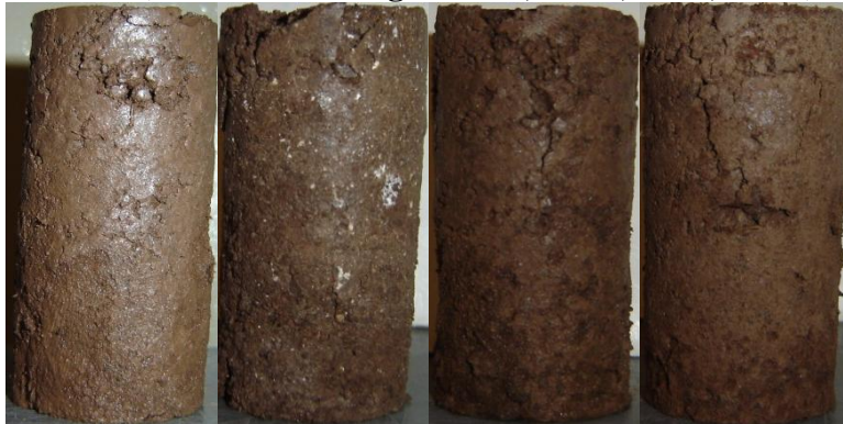
Figure A 29: Harvard Miniature Lomill Specimens at the End of 8 Freeze-Thaw Cycles After UCS. (From Left to Right: Raw, Lime, CFA, CKD)
