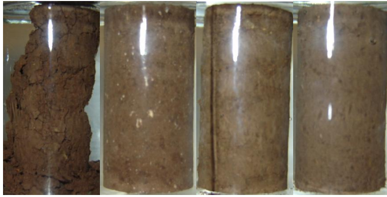
Figure E 10: Lomill Specimens at the End of 5 Hours of Soaking Period (From Left to Right: Raw, Lime, CFA, CKD)
