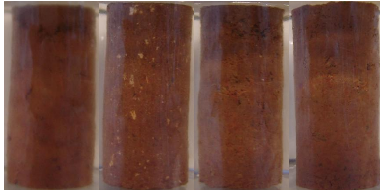
Figure E 5: Carnasaw Specimens at the Beginning of 5 Hours of Soaking Period (From Left to Right: Raw, Lime, CFA, CKD)
