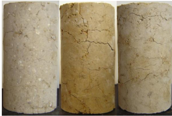
Figure B 13: Harvard Miniature Dennis Specimens Before 2 Wet-Dry Cycles. (From Left to Right: Lime, CFA, CKD)
