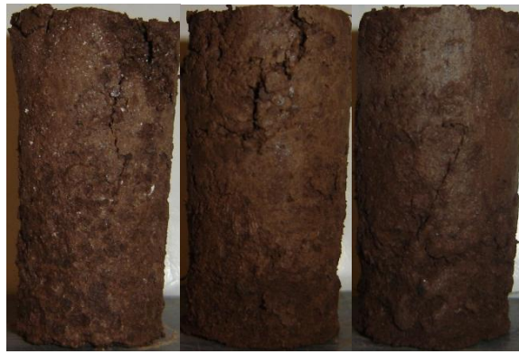
Figure 4.15: Harvard Miniature Lomill Specimens at the End of 12 Freeze-Thaw Cycles After UCS Test (From Left to Right: Lime, CFA, CKD)
