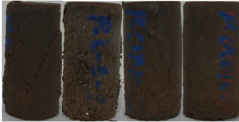
Figure 4.11: Harvard Miniature Port Specimens at the End of 12 Freeze-Thaw Cycles After UCS Test (From Left to Right: Raw, Lime, CFA, CKD)
