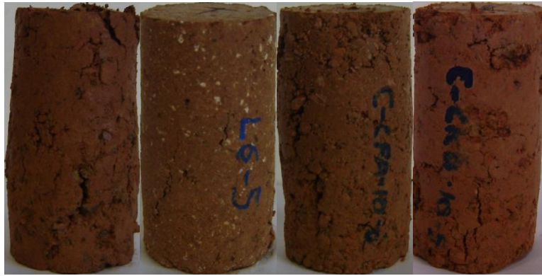
Figure A 16: Harvard Miniature Carnasaw Specimens at the End of 4 Freeze-Thaw Cycles After UCS. (From Left to Right: Raw, Lime, CFA, CKD)
