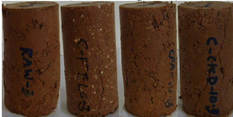
Figure A 15: Harvard Miniature Carnasaw Specimens at the End of 1 Freeze-Thaw Cycle After UCS. (From Left to Right: Raw, Lime, CFA, CKD)
