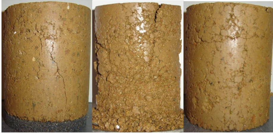
Figure 4.54: Carnasaw Specimens After Vacuum Saturation After UCS Test (From Left to Right: Lime, CFA, CKD)
