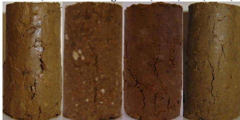
Figure A 21: Harvard Miniature Dennis Specimens at the End of 1 Freeze-Thaw Cycle After UCS. (From Left to Right: Raw, Lime, CFA, CKD)
