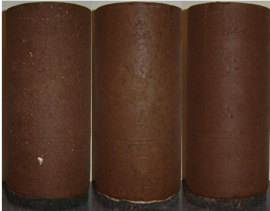
Figure C 3: Port Specimens Tested for M_r at the End of 4 Freeze-Thaw Cycles (From Left to Right: Lime, CFA, CKD)
