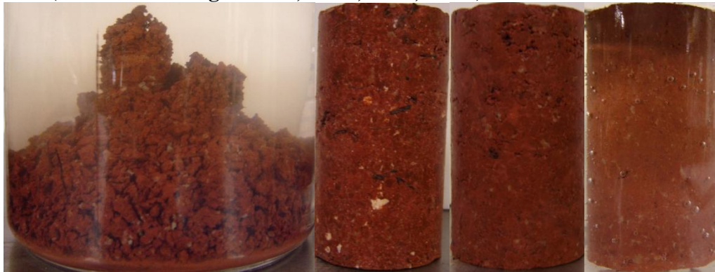
Figure B 2: Harvard Miniature Kingfisher Specimens After 1 Wet-Dry cycle at the End of 5 Hours of Soaking Period. (From Left to Right: Raw, Lime, CFA, CKD)
