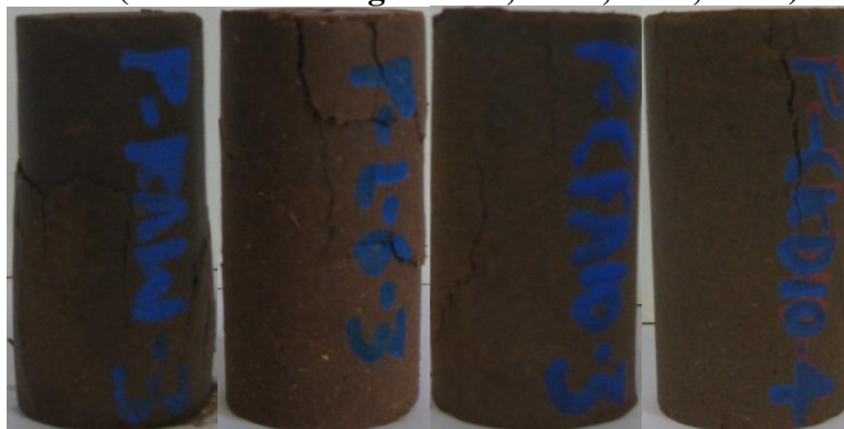
Figure A 3: Harvard Miniature Port Specimens at the End of 1 Freeze-Thaw Cycle After UCS (From Left to Right: Raw, Lime, CFA, CKD)
