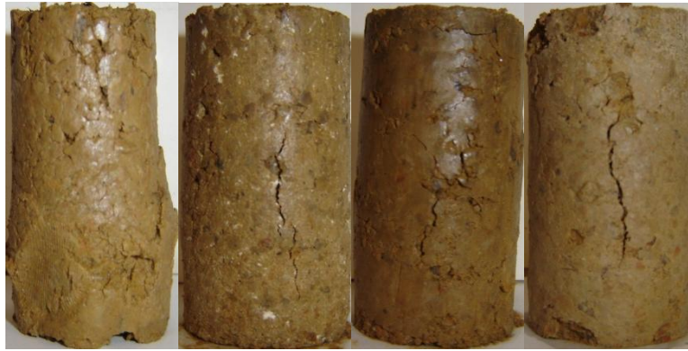
Figure A 22: Harvard Miniature Dennis Specimens at the End of 4 Freeze-Thaw Cycles After UCS. (From Left to Right: Raw, Lime, CFA, CKD)
