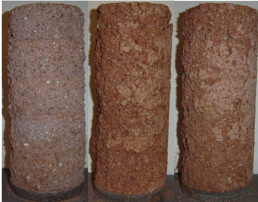
Figure D 3: Kingfisher Specimens Failed Before M_r After 2 Wet-Dry Cycles (From Left to Right: Lime, CFA, CKD)
