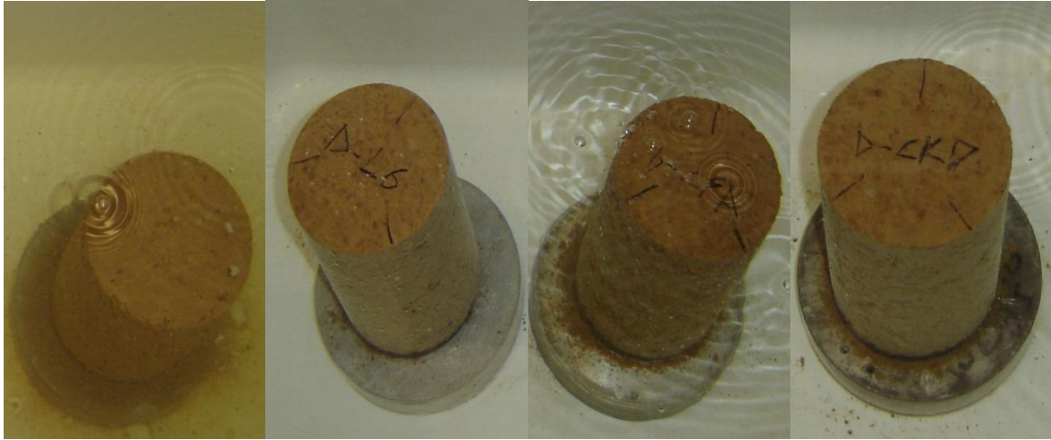
Figure D 11: Dennis Specimens in Water during 1 Wet-Dry Cycle (From Left to Right: Raw, Lime, CFA, CKD)
