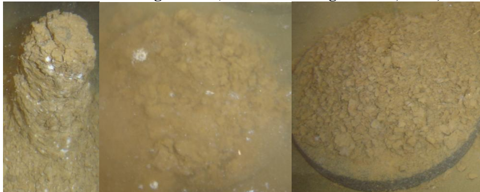
Figure 4.22: Harvard Miniature Dennis Specimens After 2 Wet-Dry Cycles at the End of 5- Hour Soaking Period (From Left to Right: Lime, CFA, CKD)
