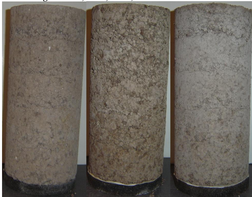
Figure D 18: Lomill Specimens after 42 Hour Oven Drying During 1 Wet-Dry Cycle (From Left to Right: Lime, CFA, CKD)
