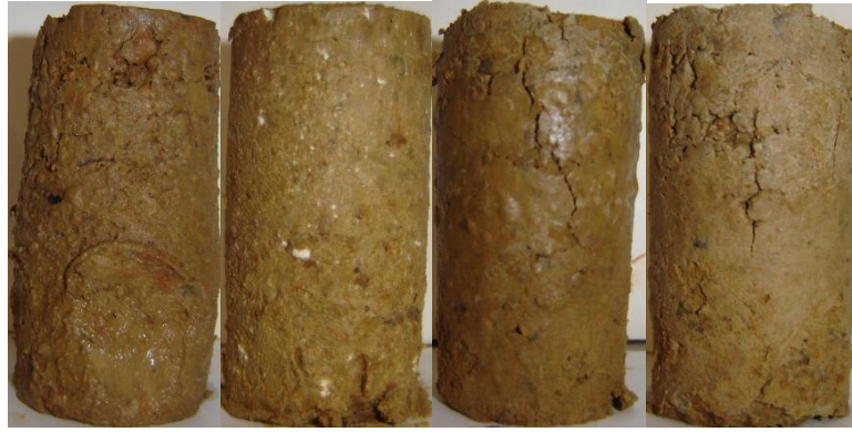
Figure 4.14: Harvard Miniature Dennis Specimens at the End of 12 Freeze-Thaw Cycles After UCS Test (From Left to Right: Raw, Lime, CFA, CKD)
