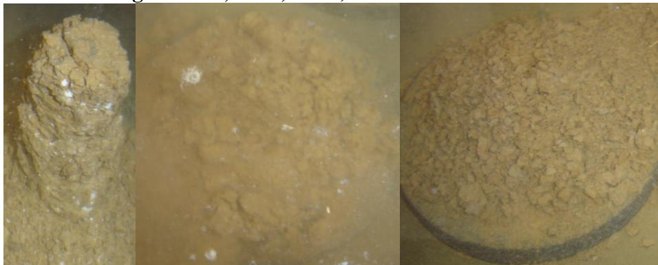
Figure B 14: Harvard Miniature Dennis Specimens After 2 Wet-Dry Cycles at the End of 5 Hours of Soaking Period. (From Left to Right: Lime, CFA, CKD)
