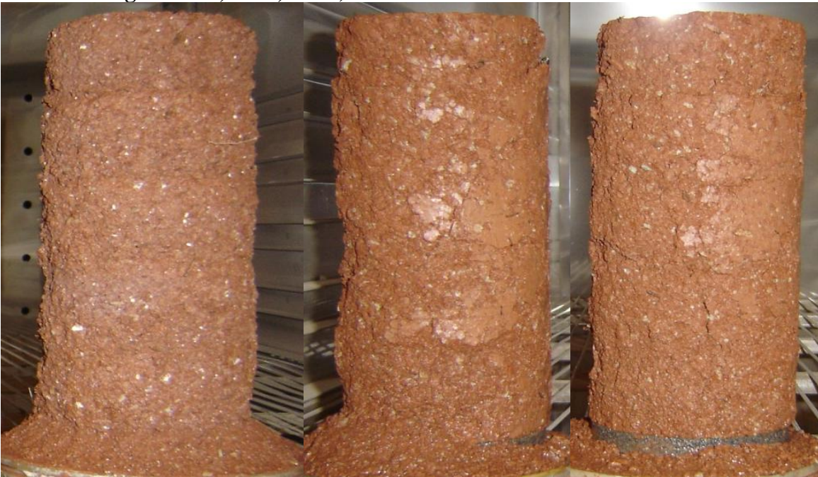
Figure D 6: Kingfisher Specimens in Oven during 2 Wet-Dry Cycles (From Left to Right: Lime, CFA, CKD)
