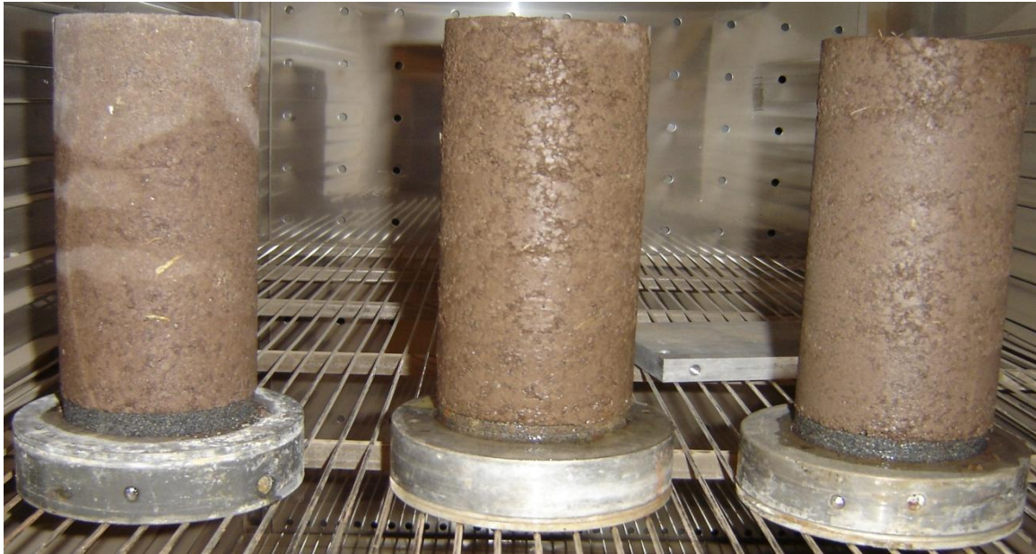
Figure D 17: Lomill Specimens During 1 Wet-Dry Cycle During Oven Drying (From Left to Right: Lime, CFA, CKD)
