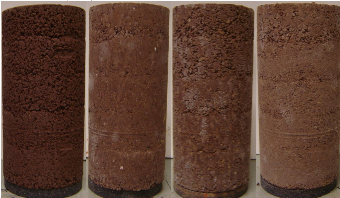
Figure D 14: Lomill Specimens Tested for M_r After 0 Wet-Dry Cycles (From Left to Right: Raw, Lime, CFA, CKD)
