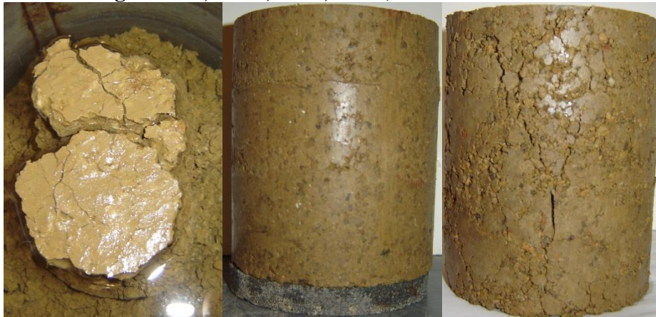
Figure F 6: Dennis Specimens After Vacuum Saturation After UCS Test (Raw (Left) and CKD failed before UCS)
