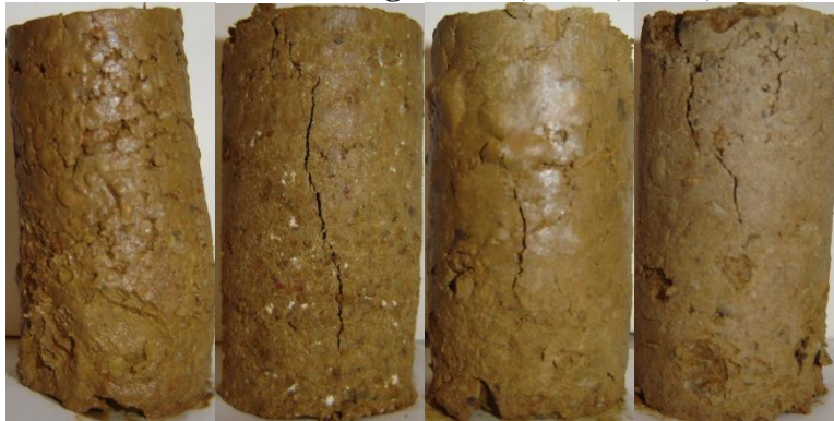
Figure A 23: Harvard Miniature Dennis Specimens at the End of 8 Freeze-Thaw Cycles After UCS. (From Left to Right: Raw, Lime, CFA, CKD)
