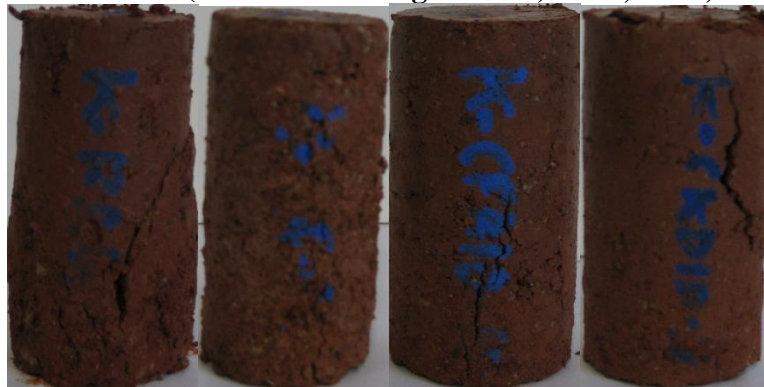
Figure 4.12: Harvard Miniature Kingfisher Specimens at the End of 12 Freeze-Thaw Cycles After UCS Test (From Left to Right: Raw, Lime, CFA, CKD)
