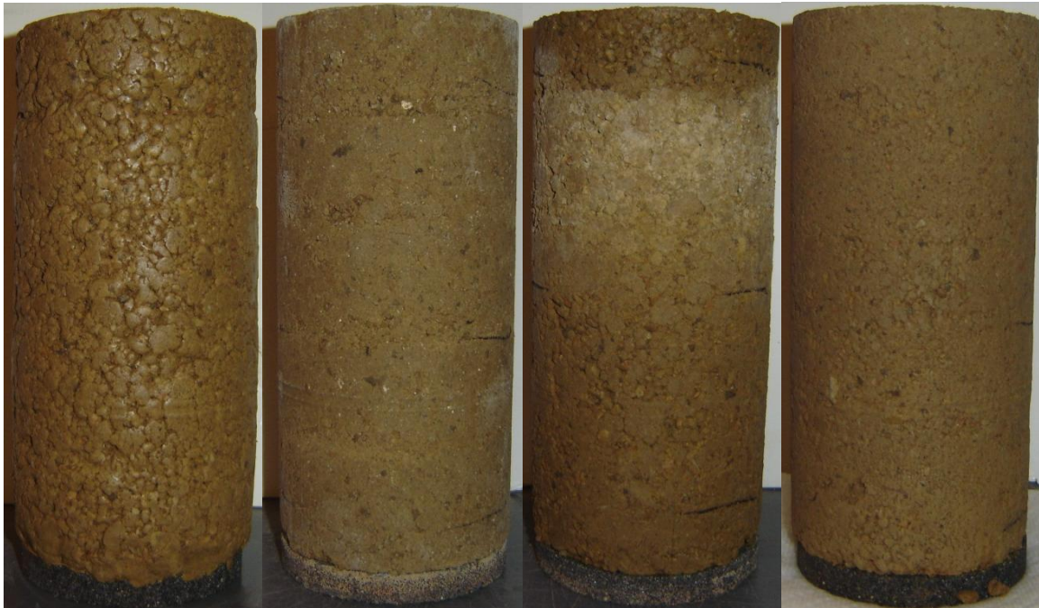
Figure C 9: Dennis Specimens Tested for M_r at the End of 1 Freeze-Thaw Cycle (From Left to Right: Raw, Lime, CFA, CKD)
