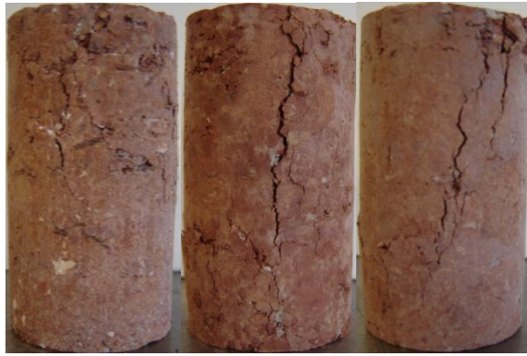
Figure B 4: Harvard Miniature Kingfisher Specimens After 1 Wet-Dry Cycle After UCS. (From Left to Right: Lime, CFA, CKD)
