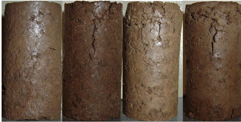
Figure A 28: Harvard Miniature Lomill Specimens at the End of 4 Freeze-Thaw Cycles After UCS. (From Left to Right: Raw, Lime, CFA, CKD)
