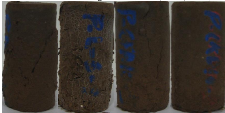
Figure A 6: Harvard Miniature Port Specimens at the End of 12 Freeze-Thaw Cycles After UCS (From Left to Right: Raw, Lime, CFA, CKD)
