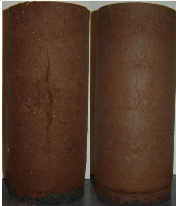
Figure C 4: Port Specimens Tested for M_r at the end of 8 Freeze-Thaw Cycles (From Left to Right: Lime, CKD; CFA Failed Before Test in Cycle 8)
