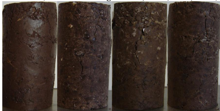
Figure A 26: Harvard Miniature Lomill Specimens at the End of 0 Freeze-Thaw Cycles After UCS. (From Left to Right: Raw, Lime, CFA, CKD)
