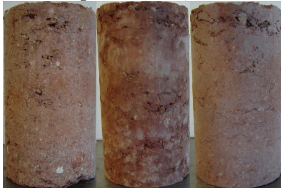
Figure B 5: Harvard Miniature Kingfisher Specimens Before 2 Wet-Dry Cycles. (From Left to Right: Lime, CFA, CKD)
