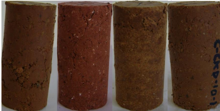
Figure A 14: Harvard Miniature Carnasaw Specimens at the End of 0 Freeze-Thaw Cycles After UCS. (From Left to Right: Raw, Lime, CFA, CKD)
