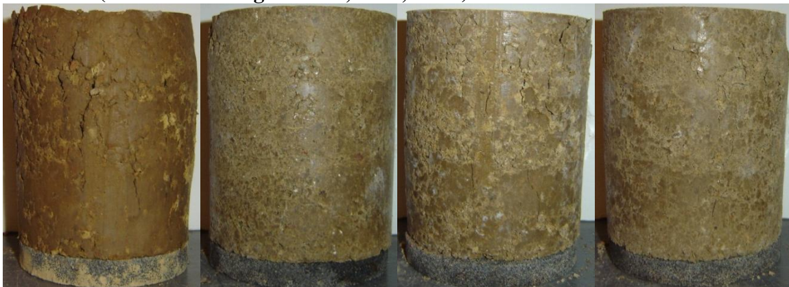
Figure F 5: Dennis Specimens Before Vacuum Saturation at the End of UCS test (From Left to Right: Raw, Lime, CFA, CKD)
