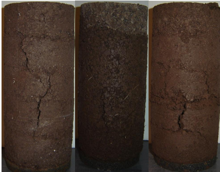
Figure C 13: Dennis Specimens Tested for M_r at the End of 4 Freeze-Thaw Cycles (From Left to Right: Lime, CFA, CKD)
