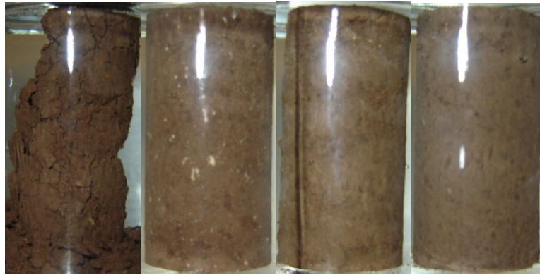
Figure 4.46: Lomill Specimens at the End of 5-Hour Soaking Period (From Left to Right: Raw, Lime, CFA, CKD)
