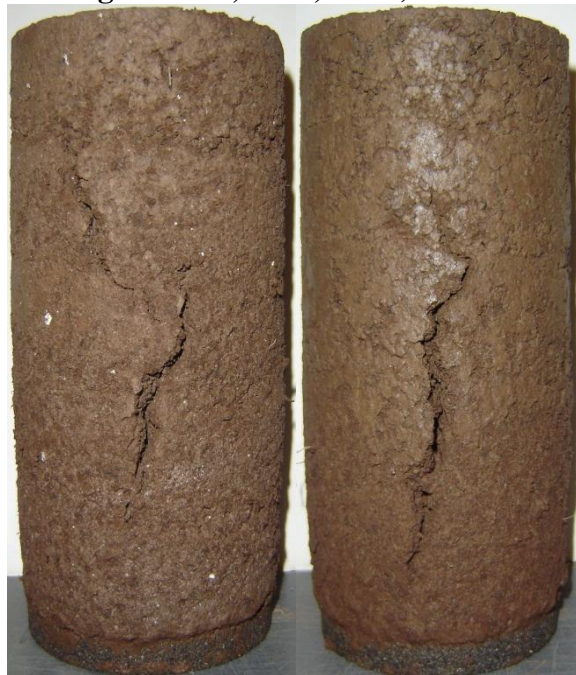
Figure C 14: Dennis Specimens Tested for M_r at the End of 8 Freeze-Thaw Cycles (From Left to Right: Lime, CFA)
