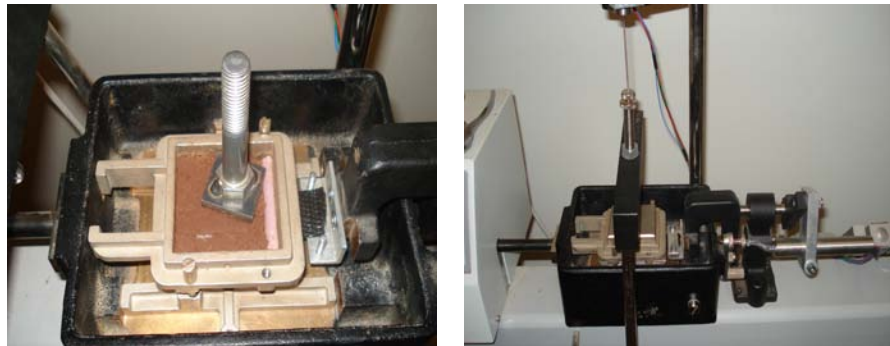
Figure 32. Small-scale pullout tests in Chickasha soil using a DST machine
