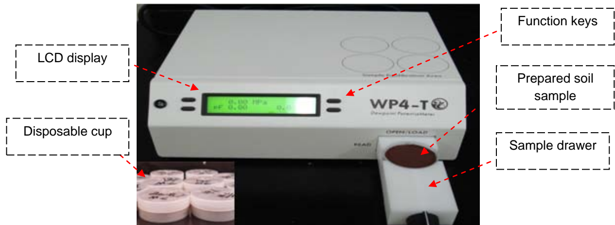
Figure 11. WP4 Water Potentiometer equipment (soil samples in sealed cups are shown in the inset)
