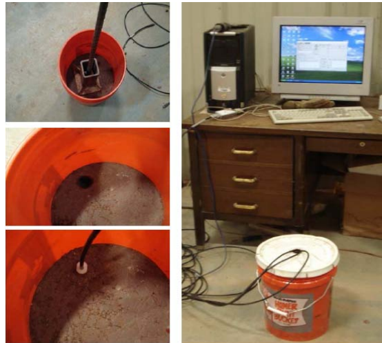
Figure 5. Fredlund sensors placed in a calibration bucket to measure matric suction of the Chickasha soil
