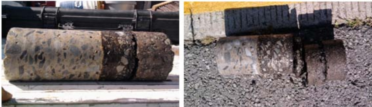
Figure 2.26 - Cores extracted on the oldest McAlester Overlay.
