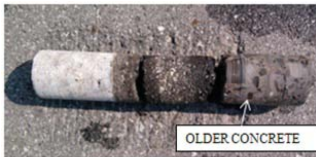
Figure 2.4 – A typical core from an Oklahoma whitetopping.
