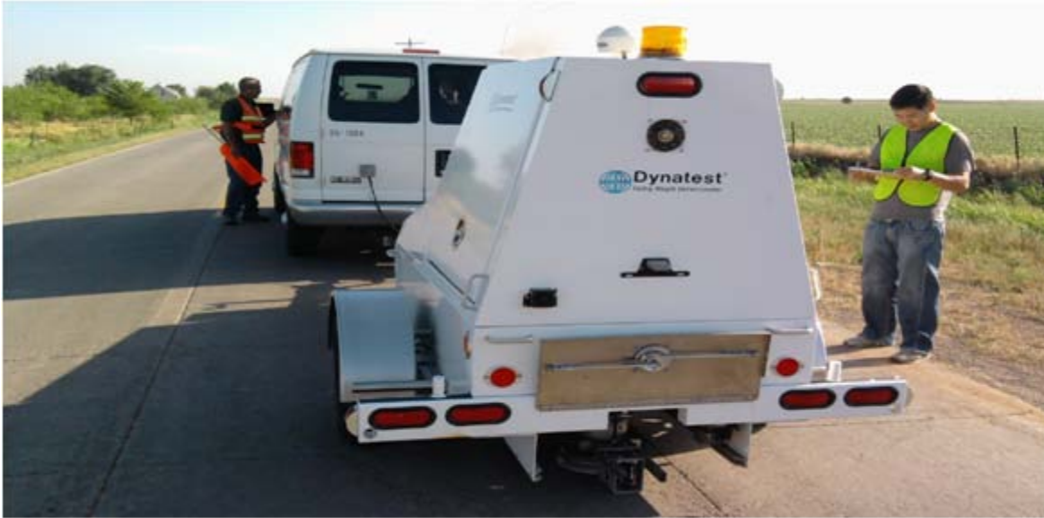
Figure 2.1 - The FWD behind the truck had a computer and camera assembly.
