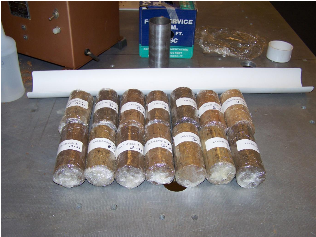
Figure 2 – Selected Specimens Trimmed in Length and Diameter
