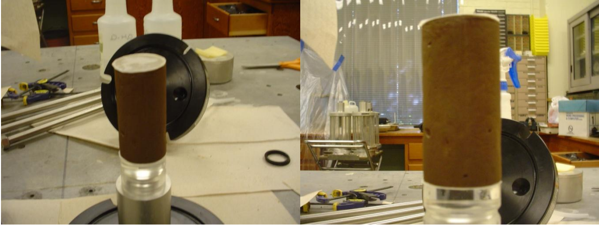
Figure 11 – Specimens on Triaxial Base
