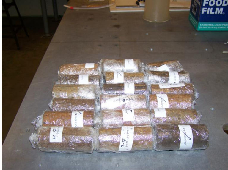
Figure 5 – All 18 In-Situ Specimens after Shear Testing
