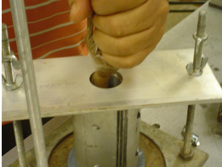
Figure 8 – Placing Slurry Specimen into Mold
