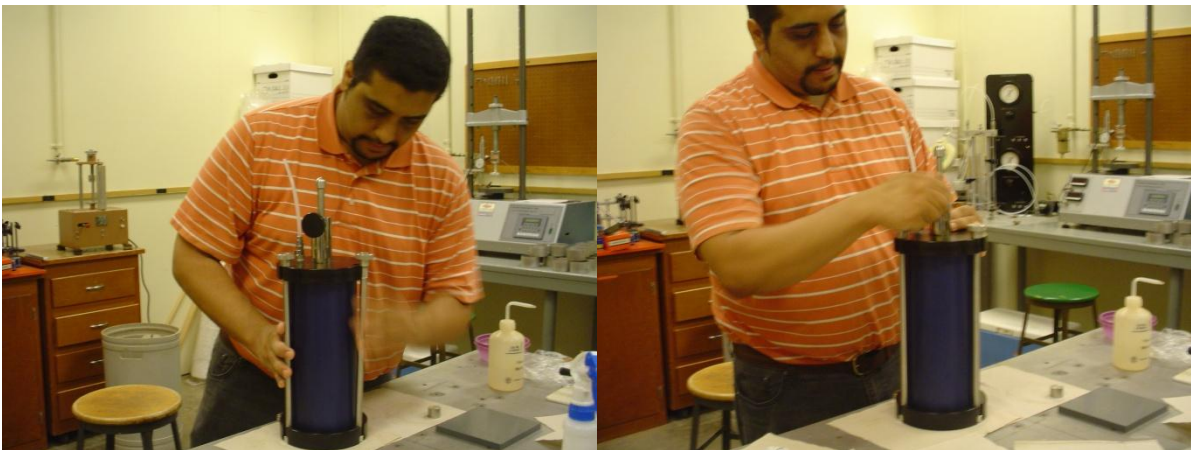
Figure 14 – Assembly of the Triaxial Cell
