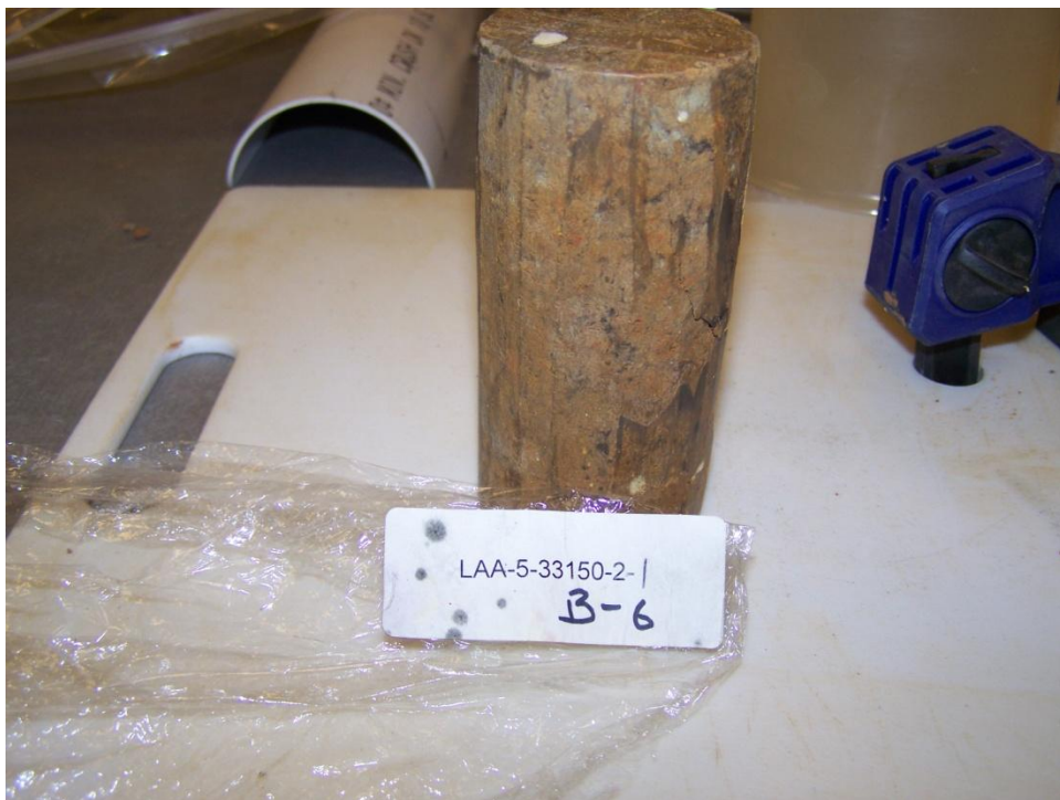
Figure 4 – In-Situ Specimen after Shear Testing
