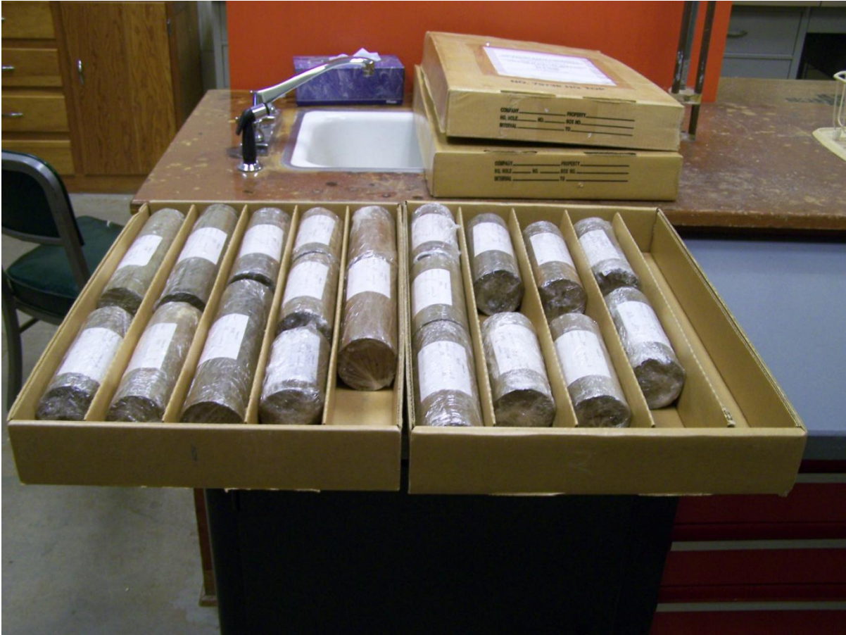
Figure 1 – Soil Samples Prior to Trimming
