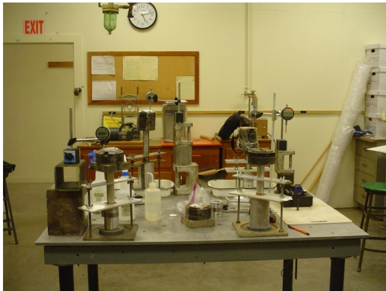
Figure 9 – SPNC Devices During Consolidation
