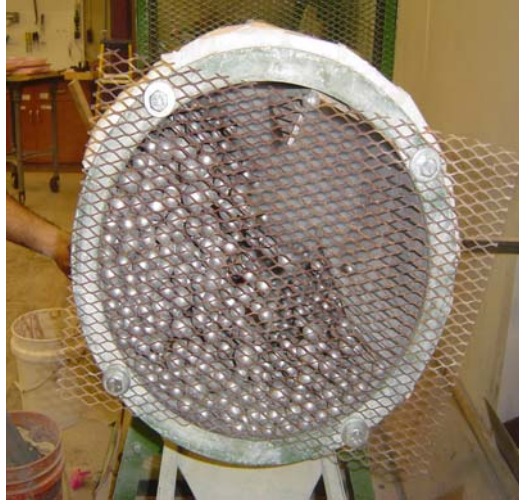
Figure 3.3 Balls motion in the grinding system
