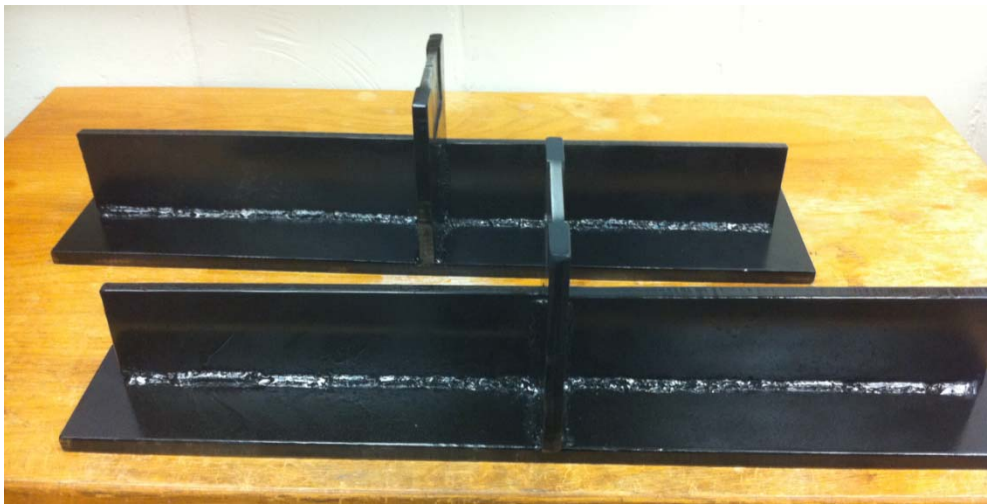
Figure 5: Bearing Compression Test Fixtures
