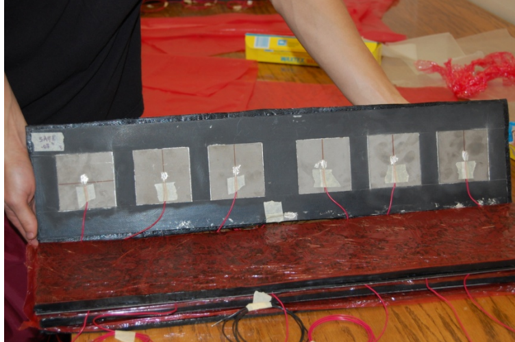
Figure 8: Six 0.080-Inch Thick Wafers on a Bearing Plate
