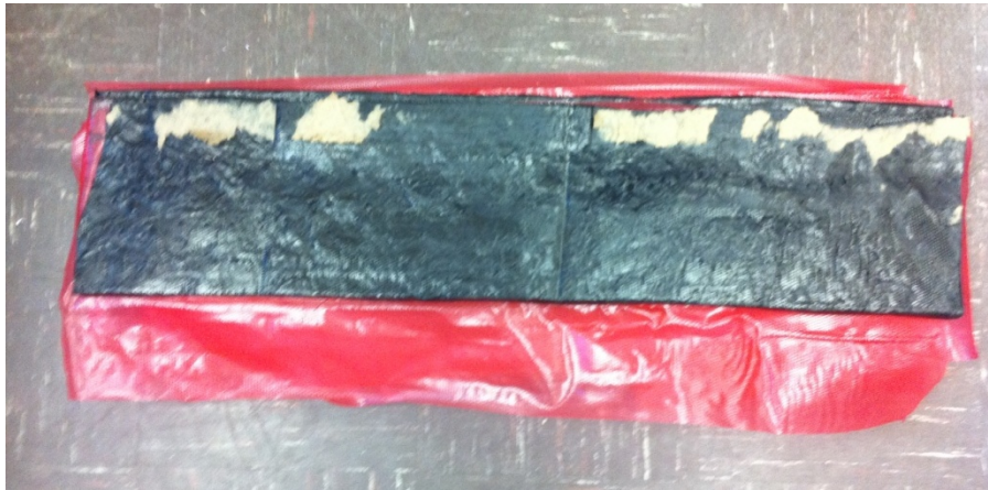
Figure 4: Elastomeric rubber layers for the bridge bearing
