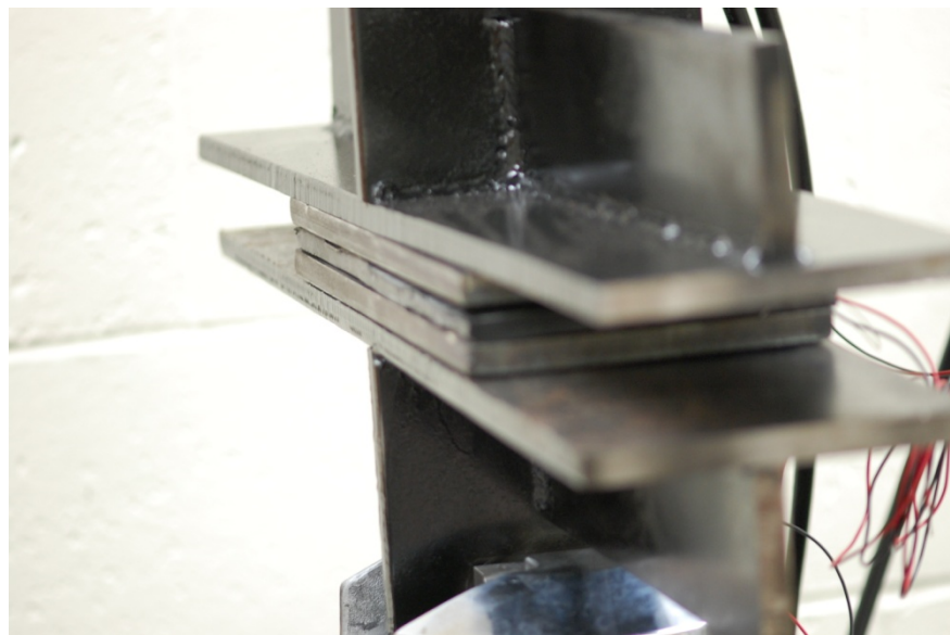
Figure 7: "Pre-Prototype Bearing" in the Test Machine
