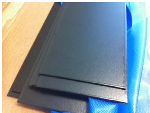
Figure 3: Steel shim layers for the bridge bearing
