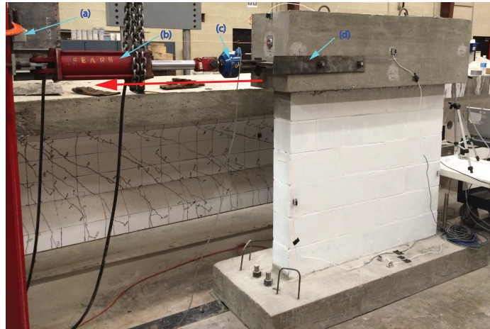
Figure 61: The masonry wall lateral test setup: (a) string potentiometer for measuring deflection; (b) hydraulic loading piston for applying lateral force; (c) load cell for measuring the applied lateral force, and (d) shear loading plate for transferring the shear load to the specimen
