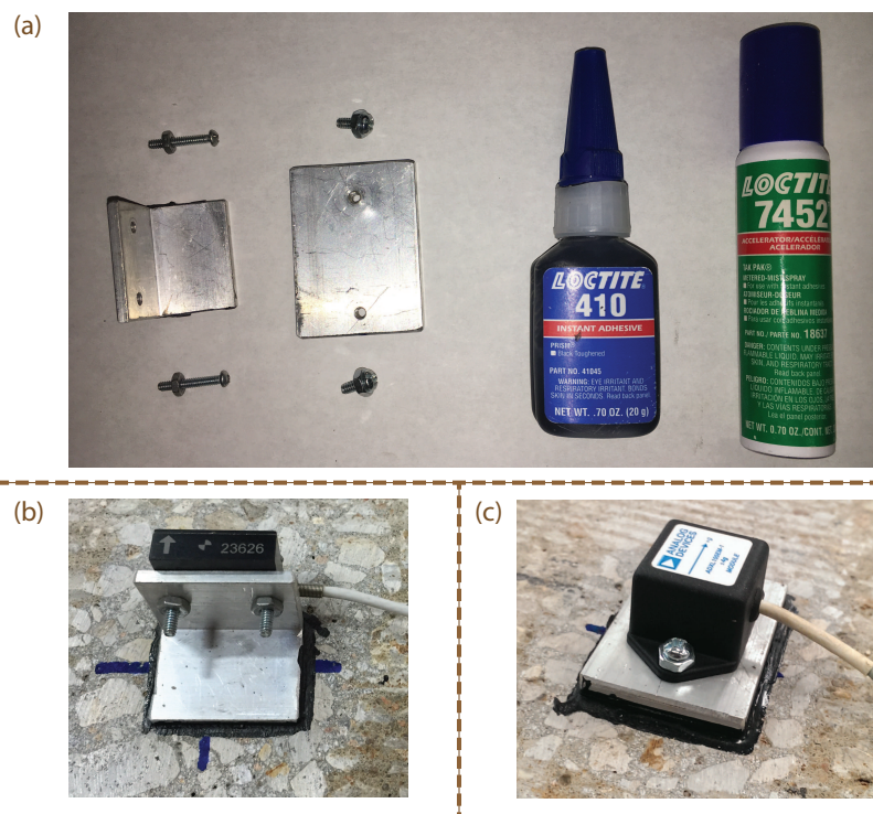
Figure 14: Accelerometer mounting accessories: (a) L-bracket for SD sensors, flat bracket for mounting ADXL sensors on the prestressed concrete girder only, Loctite 410 instant adhesive to be applied on bracket before mounting and for mounting, and Loctite 7452 accelerator for accelerating the adhesive bonding power, (b) a mounted SD sensor and (c) a mounted ADXL sensor
