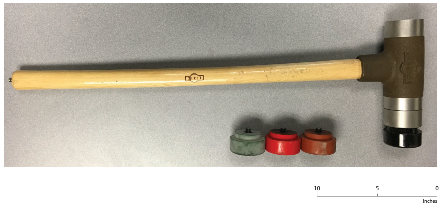
Figure 11: Dytran modal hammer
