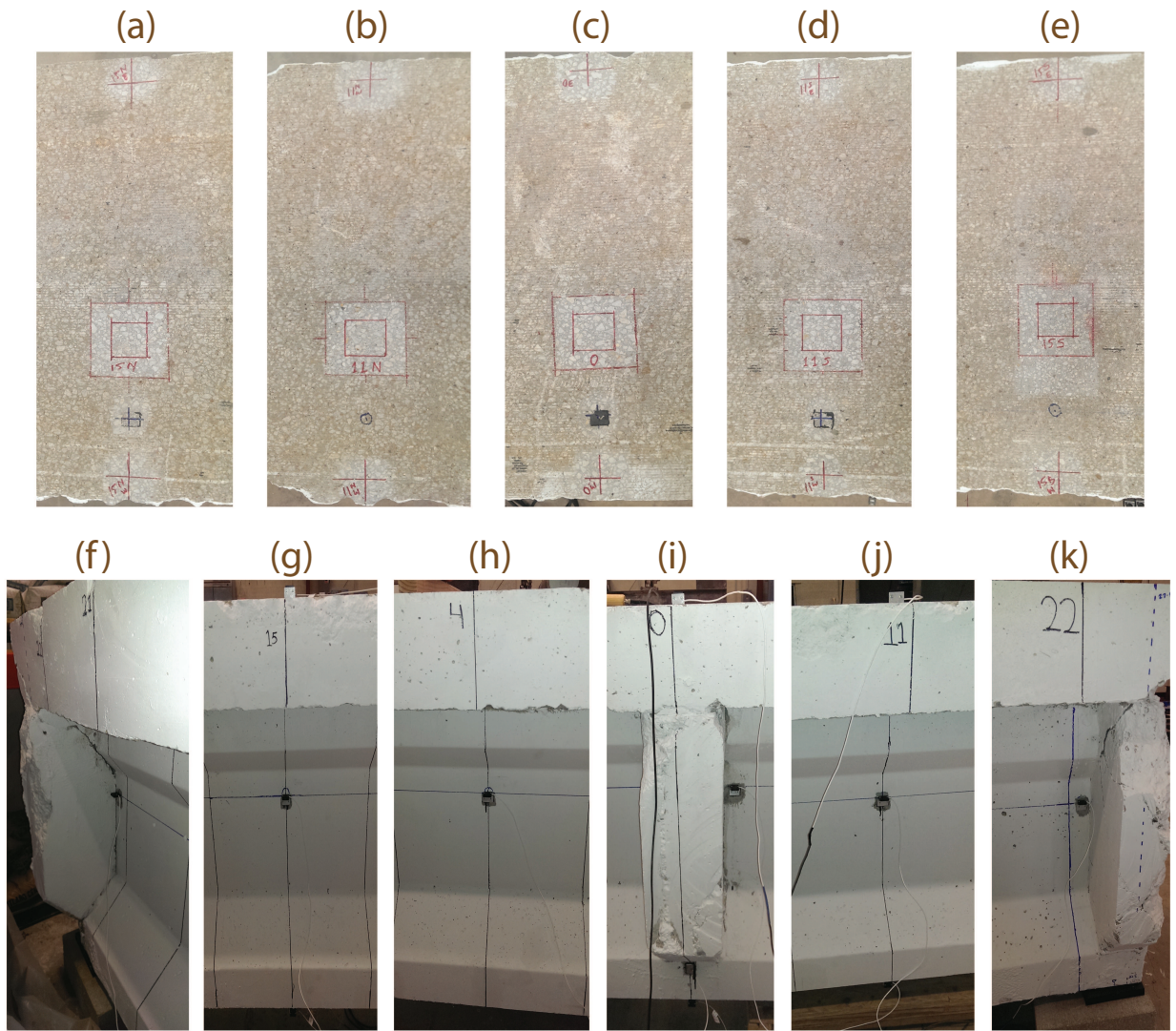
Figure 25: Top view of the prestressed concrete surface sanded and labeled with impact locations and side view of sensor layout: (a) Impact 15N, (b) Impact 11N, (c) Impact 0, (d) Impact 11S, (e) Impact 15S, (f) Sensor at 22.5N, (g) Sensors at 15N, (h) Sensors at 4N, (i) Sensors at 0, (j) Sensors at 11S, (k) Sensor at 22.5S
