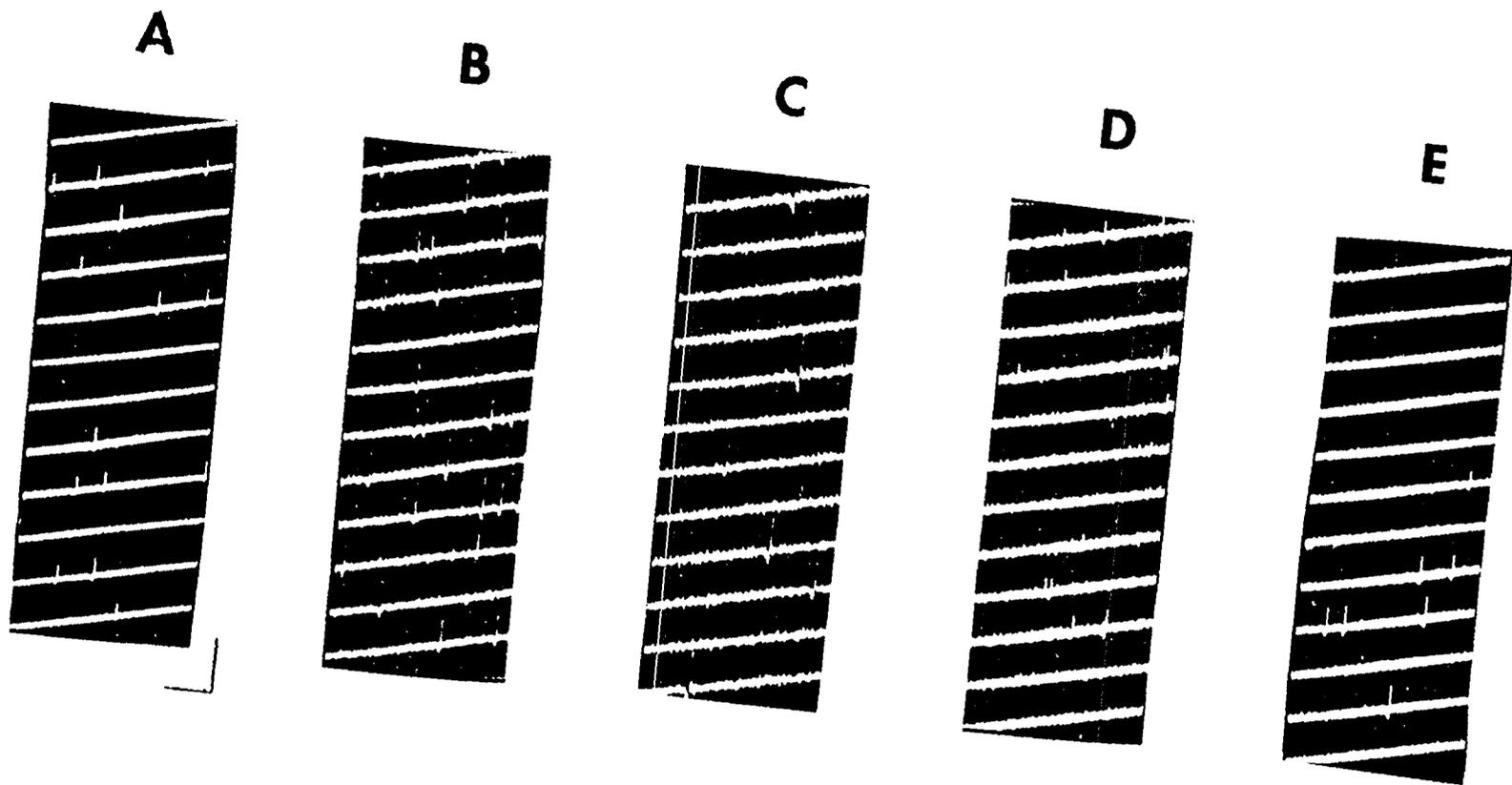
Figure 12. Film records indicating MEPP's recorded at five different end-plates. Each record represents one of the five intervals shown in Figure 11. Calibrations: vertical 1.0 mV, horizontal 50 msec, the same for all records. A. initial 1.25 mM Ca control, 5.6 MEPP's/sec; B. 10 mM Ca, 11 MEPP's/sec; C. intermediate 1.25 mM Ca control, 2.5 MEPP's/sec; D. 10 mM Ca + 1.25 mM Ba, 6.2 MEPP's/sec; E. final 1.25 mM Ca control, 3.7 MEPP's/sec.
