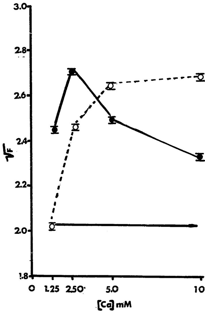
Figure 16. Means of square roots of MEPP frequency in four concentrations of Ca with and without Ba. Ordinate: square root of MEPP frequency. Abscissa: Ca concentration. Open circles (○) indicate Ca alone. Filled circles (●) indicate Ca plus 1.25 mM Ba. Bars above and below each point represent  $\pm 1$  S.E. of the mean. All MEPP frequencies based upon increases from preceding control.
