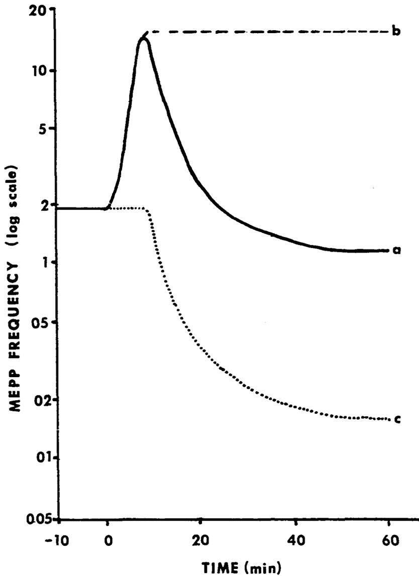
Figure 21. Separation of Ba-induced MEPP frequency curve into its components. Ordinate: MEPP frequency, log scale. Abscissa: time in minutes. Zero time indicates introduction of 0.5 mM Ba. Solid line (a) represents observed MEPP frequency, data same as Figure 9. Dashed line (b) represents plateau of increased MEPP frequency due to membrane depolarization. Dotted line (c) represents the total decline in MEPP frequency from the fast rates expected from line (b).
