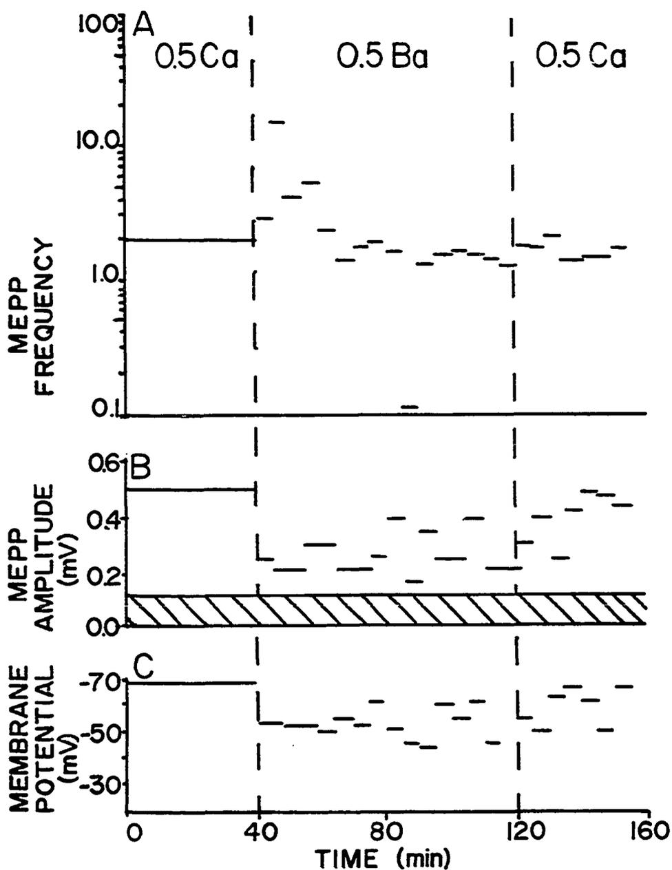
Figure 5. The effects of barium on MEPP frequency, MEPP amplitude and membrane potential in a single diaphragm. Ordinates: A. geometric mean MEPP frequency, logarithmic scale; B. mean MEPP amplitude in mV; C. muscle cell membrane potential in mV. Abscissa is time in minutes. Vertical dashed lines indicate changes in solution. Plotted horizontal lines represent interval of measurement (5 min except for control). Crossmarked bar in B indicates baseline noise.
