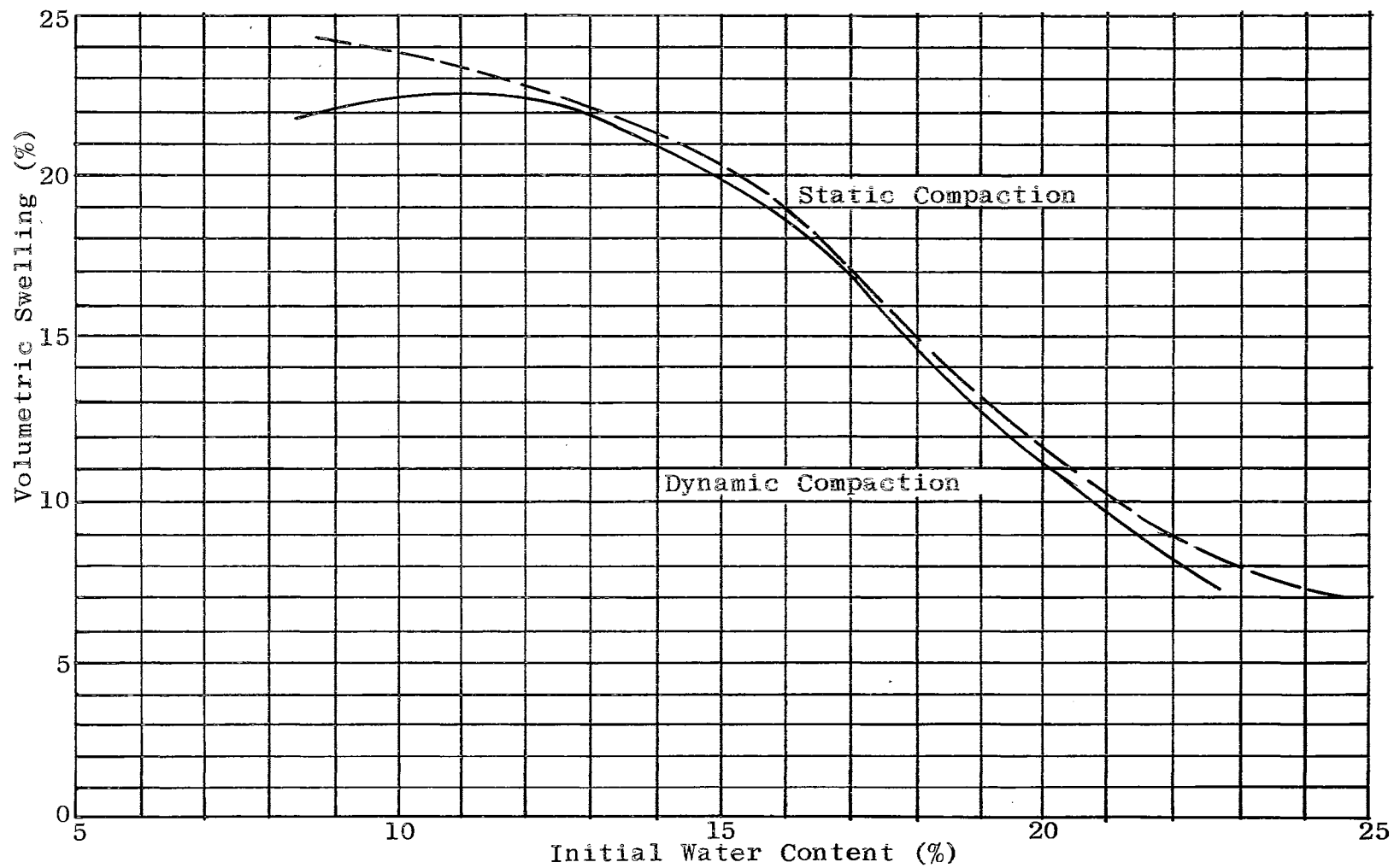
FIGURE 18. EFFECT OF COMPACTION METHOD ON VOLUMETRIC SWELLING Comparison of Dynamic and Static Compaction. (After Liu, 38.)
