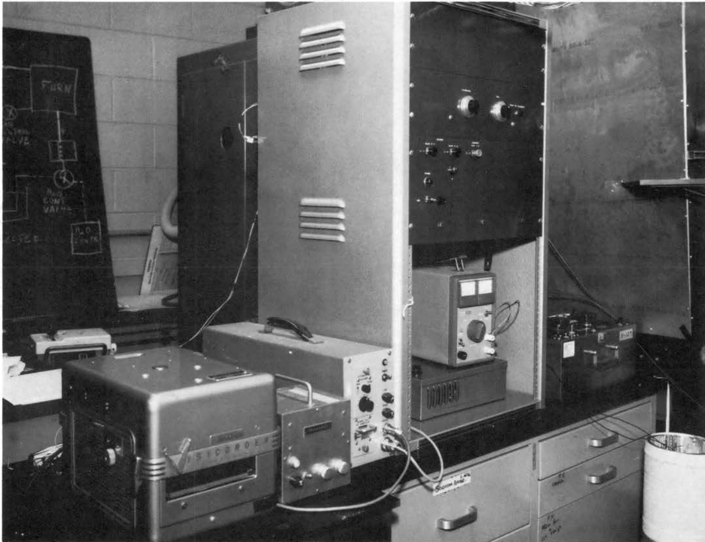
Figure 15. Control Panel, Power Supply, Amplifier, Timing Unit, and Visicorder for Sodium Heat Transfer Apparatus.
