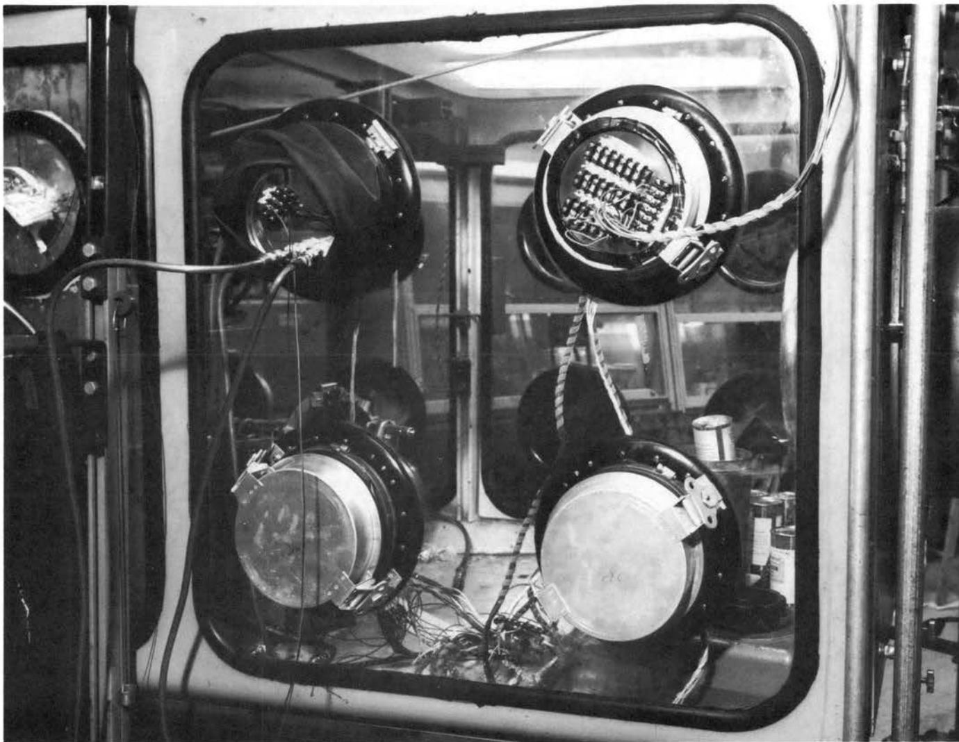
Figure 19. Argon Atmosphere Glovebox Modifications.
