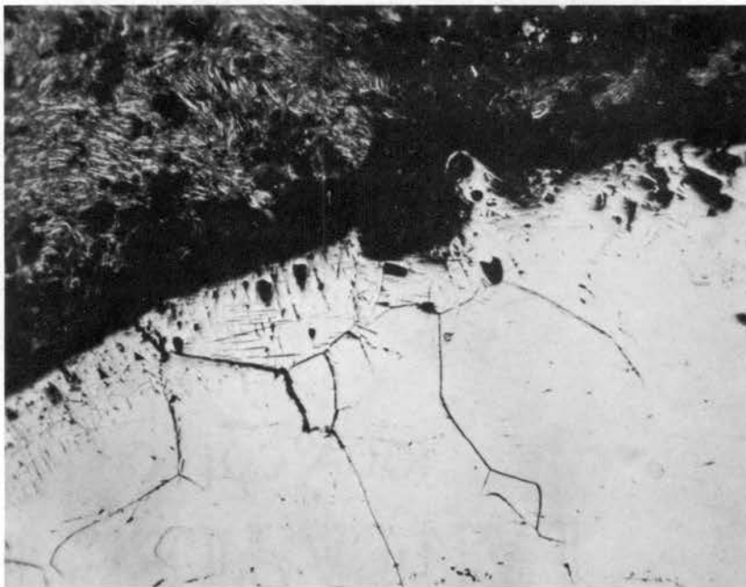
Figure 26. Photomicrograph of Tantalum Sphere: (a) As-Fabricated, (b) After Several Data Runs (90X).
