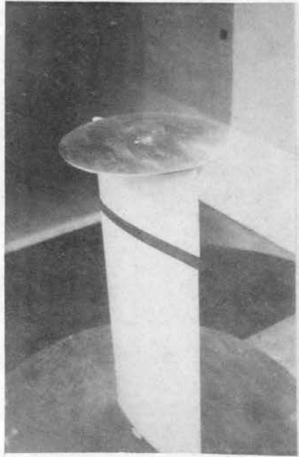
Figure 4. Supplementary Model With End-Plates Being Tested in the Wind Tunnel
