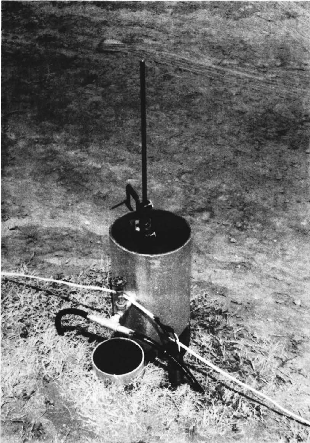
Figure 23. The Gauge Well at Station 0 + 90 With a 2 ft. Point Gauge. The Gauge Well Is Typical of the Wells at the Other 9 Stations Along the Test Channel
