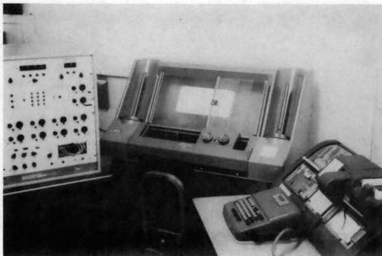
Figure 15. Analog to digital chart reader system was used to process rainfall data. The three components of the system are shown left to right: Digital converter, reader head, and keypunch.
