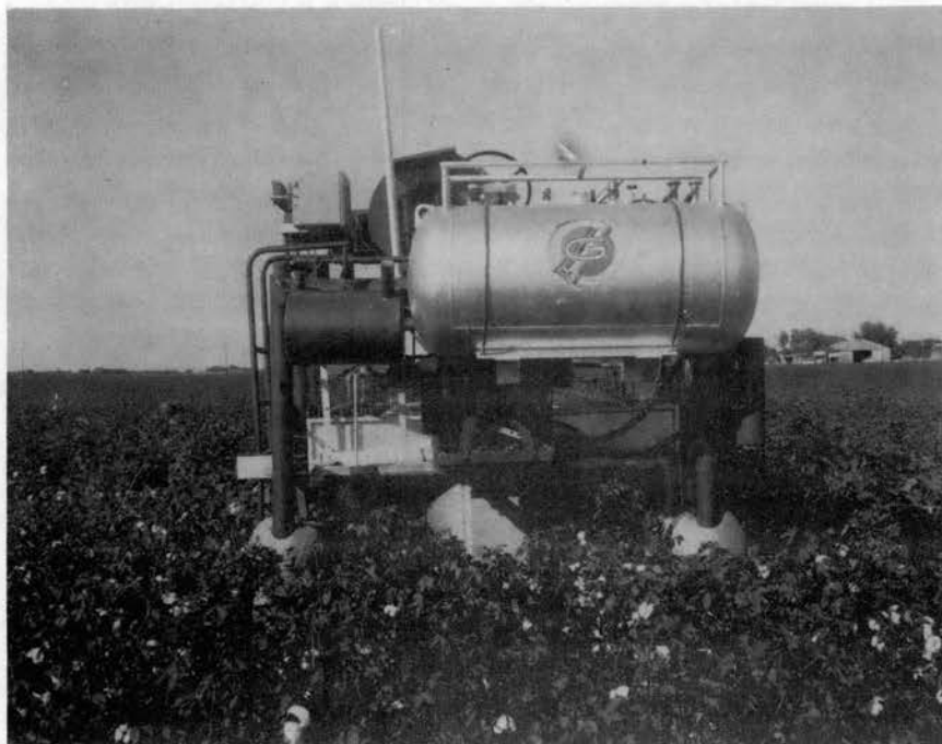
Figure 9. Front View of the Field Defoliation Unit
