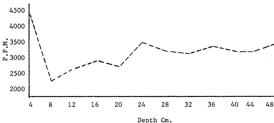
Figure 12. P.P.M. of Chloride in Different Depths of Soil Irrigated from the Surface
