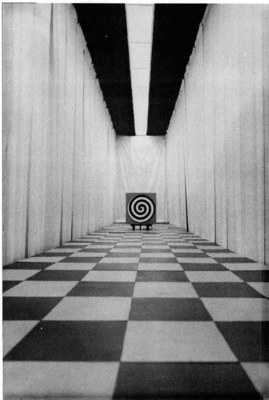
Figure 3. A 4-Inch Spiral set at a Distance of 9.5 Feet in the Visual Alley, Subtending a Visual Angle of 2^{\circ}
