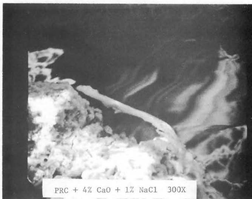
(a) 300X Photomicrograph of Salt-Lime Modified PRC
