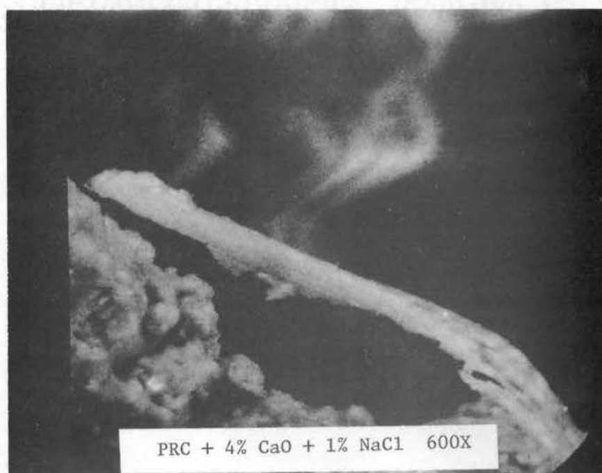
(b) 600X Photomicrograph of Salt-Lime Modified PRC
