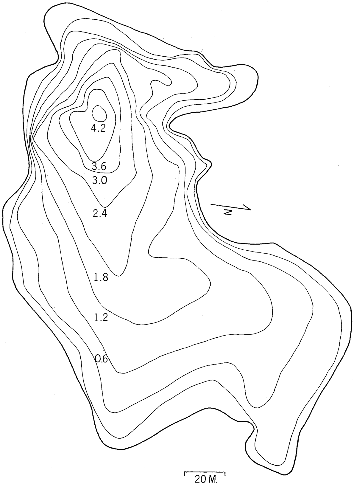
Figure 2. Contour Map of Big Clear Pond. Depth Contours in Meters Below Normal Water Level.
