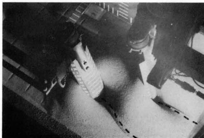
Figure 40. Effects of d = 4'' at High Interference. The Superimposed Dashed Lines are Used to Represent the Flow Pattern From Figure 32, Control Condition for High Interference ( V = 3 fps, w = 4'' , \alpha = 105^\circ , \beta_d = 75^\circ , \beta_i = 105^\circ , x = 5.5'' , y = +8'' , d = 6'' ).
