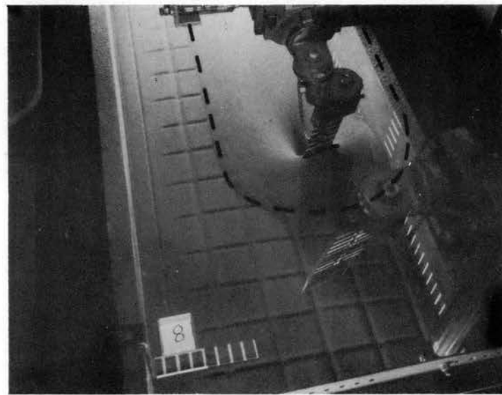
Figure 42b. Edge of Tool 5 Inches From Bin Side. Draft Force Affected to the Extent of 2 Pounds. No Measurable Effects on Other Tool Forces
