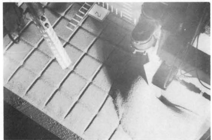
Figure 29. Reference Condition Without Interference ( V = 3 fps, \alpha = 105^\circ , \beta_d = 75^\circ )
