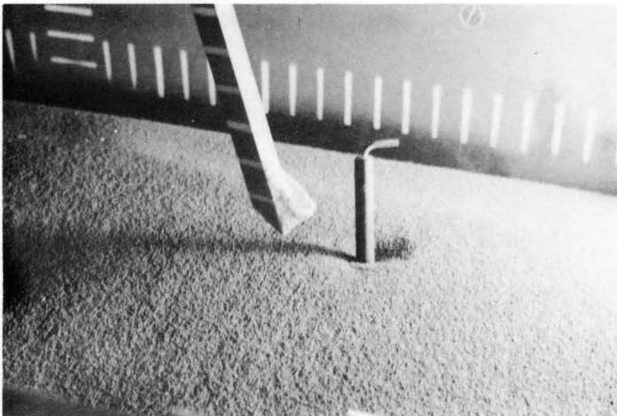
Figure 43. Views of Soil Body Formed on Tillage Tool ( V = 3 fps, w = 2'' , \alpha = 75^\circ , \beta_1 = 75^\circ , d \approx 6'' )
