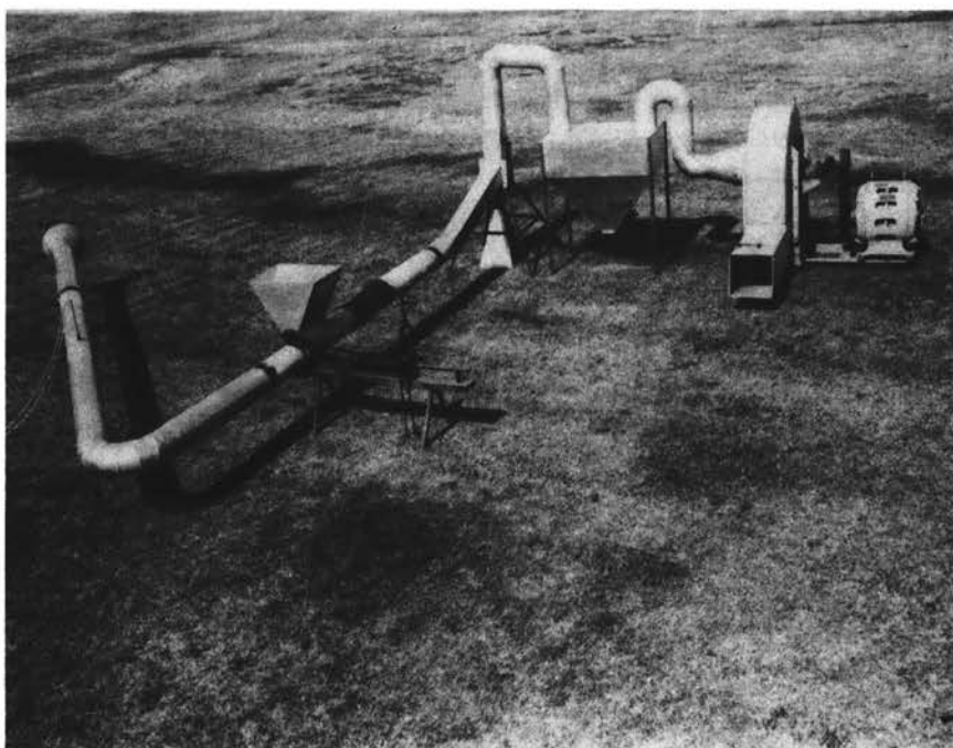
Figure 39. Complete Separating System Showing the Collection Tank
