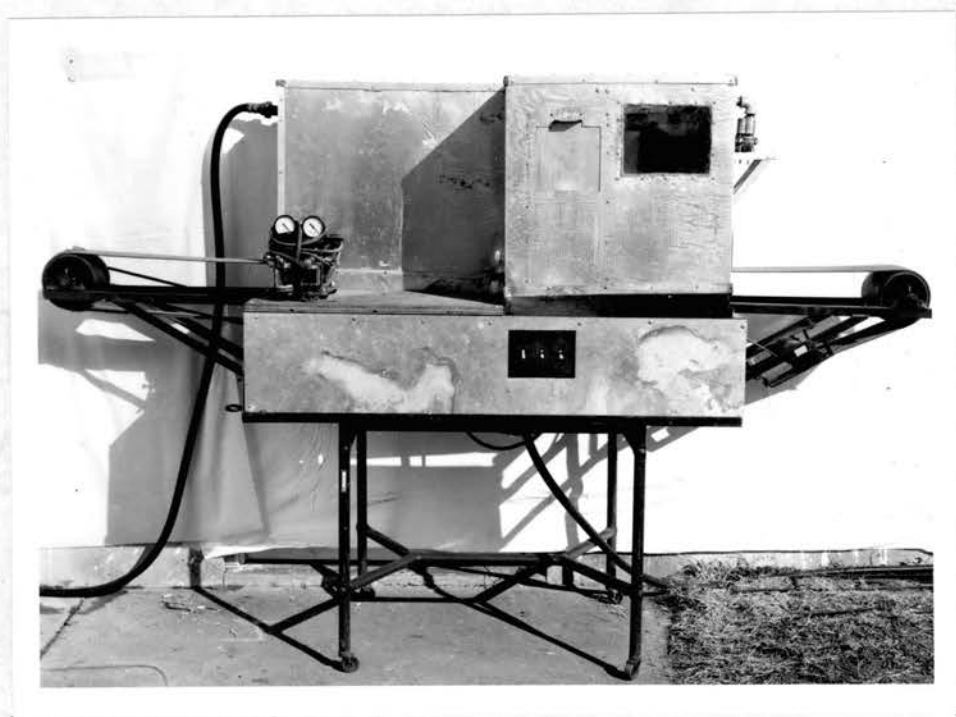
Figure 4. A machine used to inoculate differential wheat varieties for leaf rust race identification
