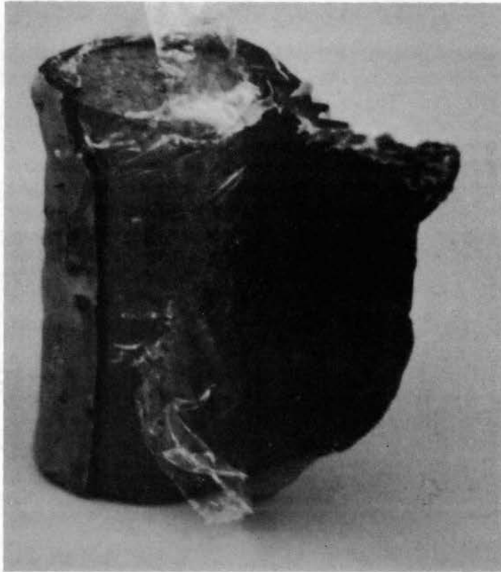
Figure 4. Waxed Coating Partially Stripped from Specimen
