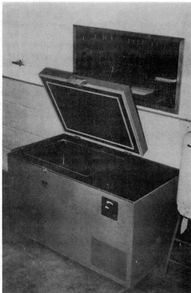
Figure 7. Controlled Temperature Cabinet
