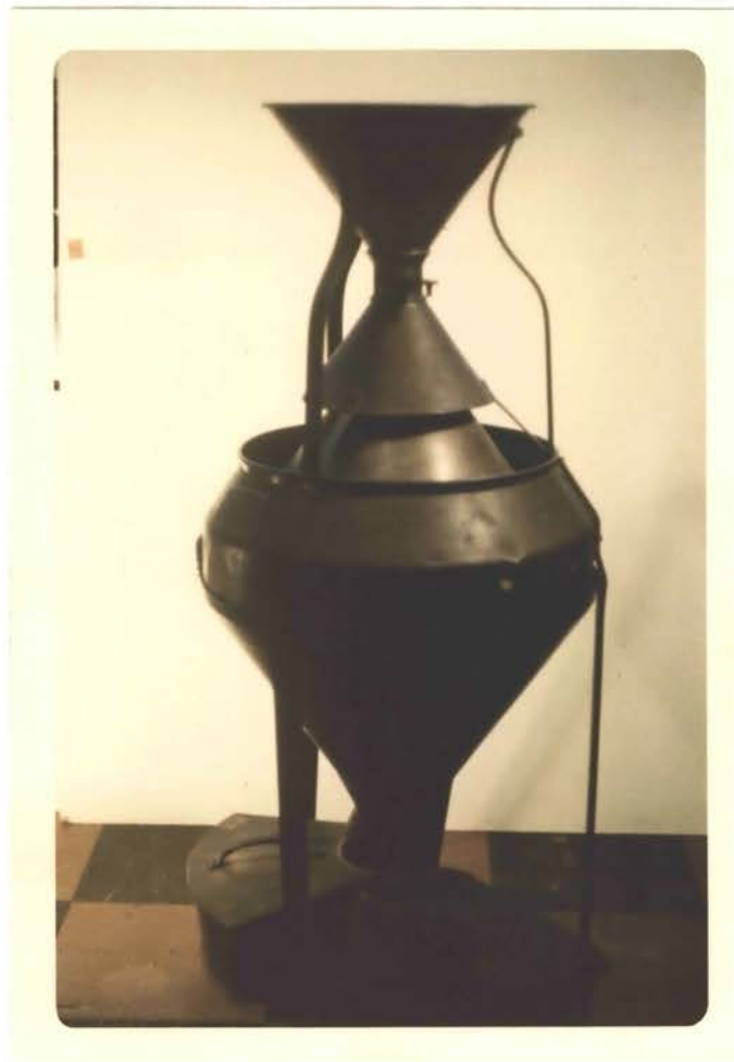
Figure 8. Boerner Aliquot Sampler used in obtaining a random sample of alfalfa seed
