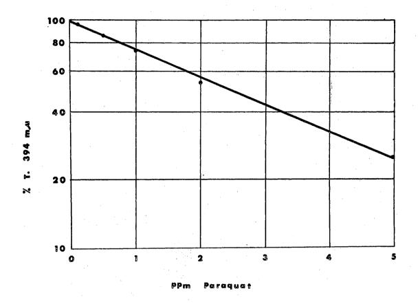
Figure 3. Standard Curve for Dithionite Chemical Quantitation at 394 mµ of Paraquat Levels.
