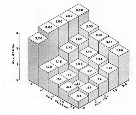
Figure 10. Effect of Differential Cu<sup>++</sup> and Paraquat Levels on Extractable Chlorophyll Absorbance in <u>C</u>. pyrenoidosa at 434 mµ.
