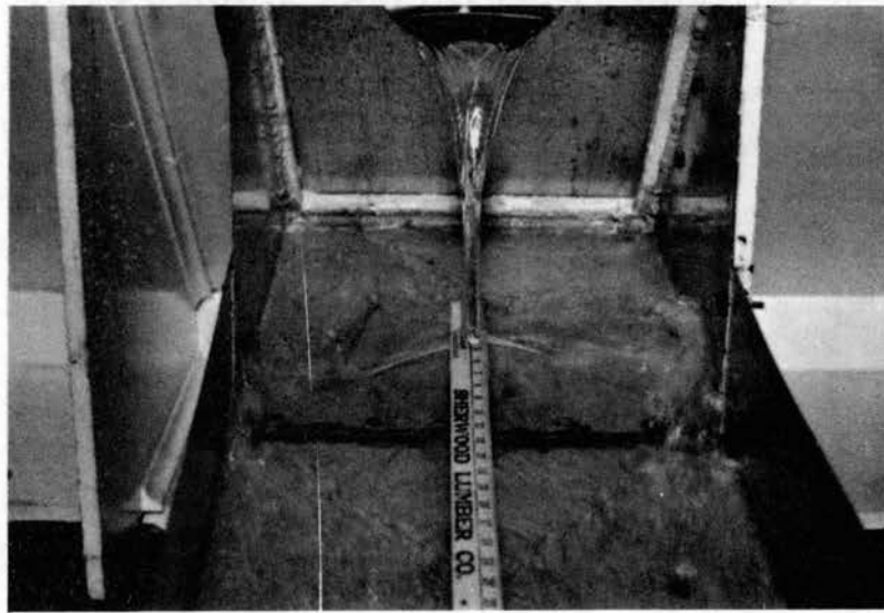
Figure 4. Circular Weir Discharge From the 8-Inch Diameter Plate.
