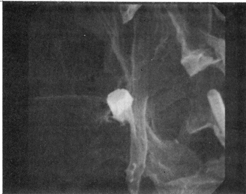
Photomicrograph 22. Union Clay 33000X-5% Lime-30 Day Cure-Group O→W
