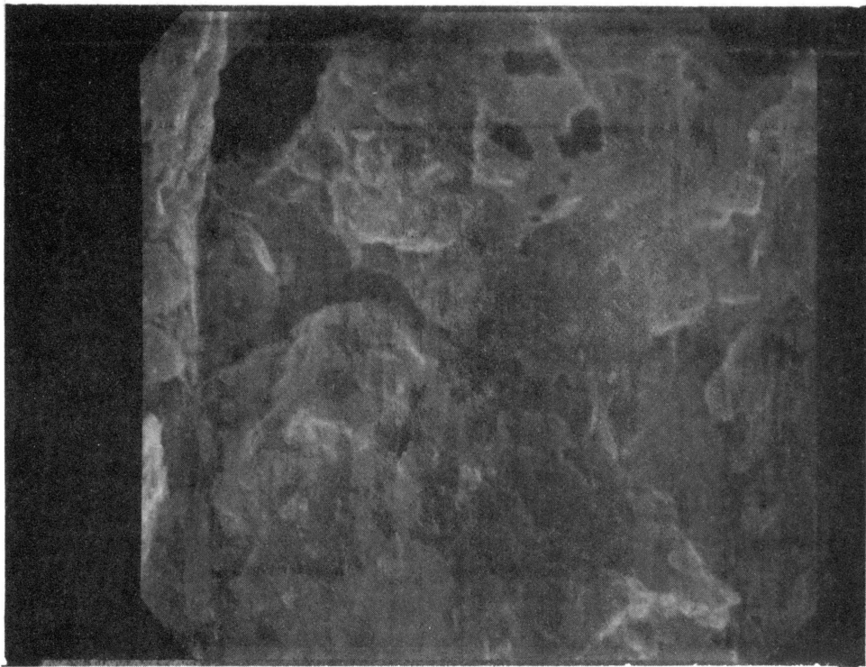
Photomicrograph 27. Summit Soil 11000X-7% Lime-2 Day Cure-Group W
