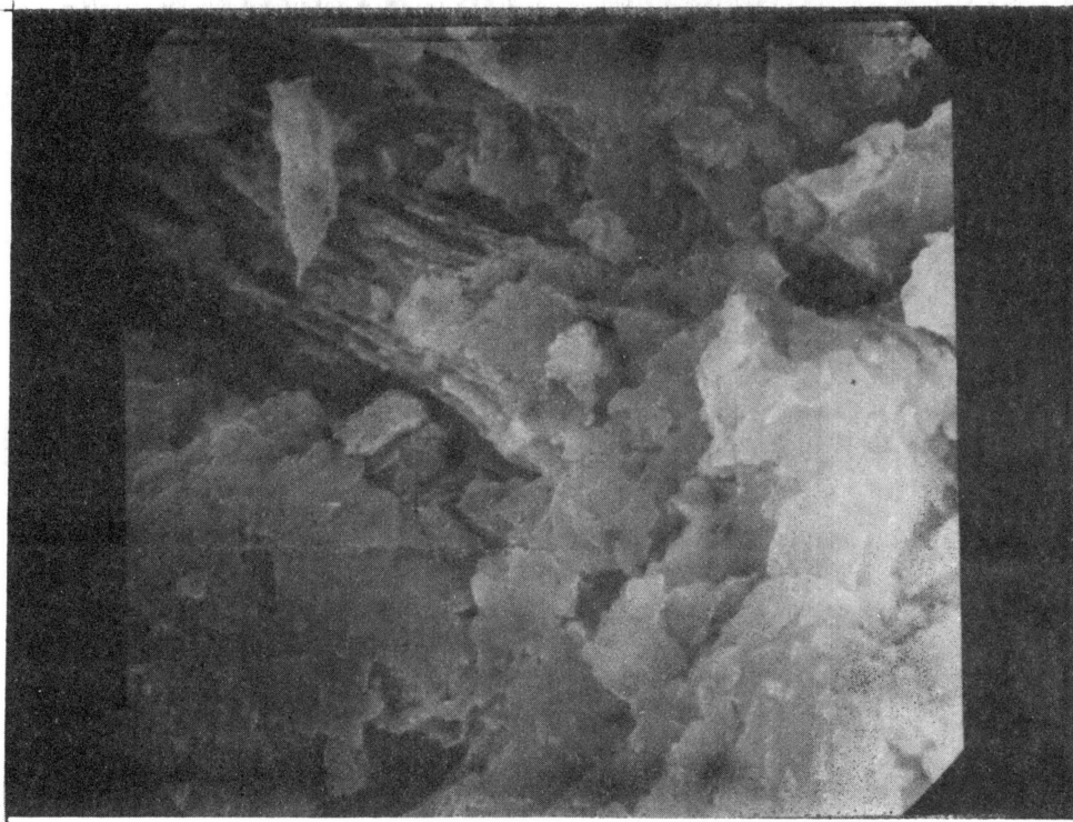
Photomicrograph 30. Summit Soil 4400X-7% Lime-90 Day Cure-Group D
