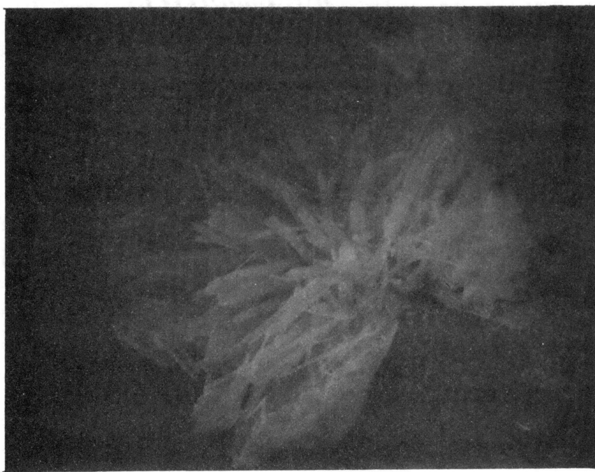
Photomicrograph 24. Union Clay 2420X-5% Lime-90 Day Cure-Group O→W
