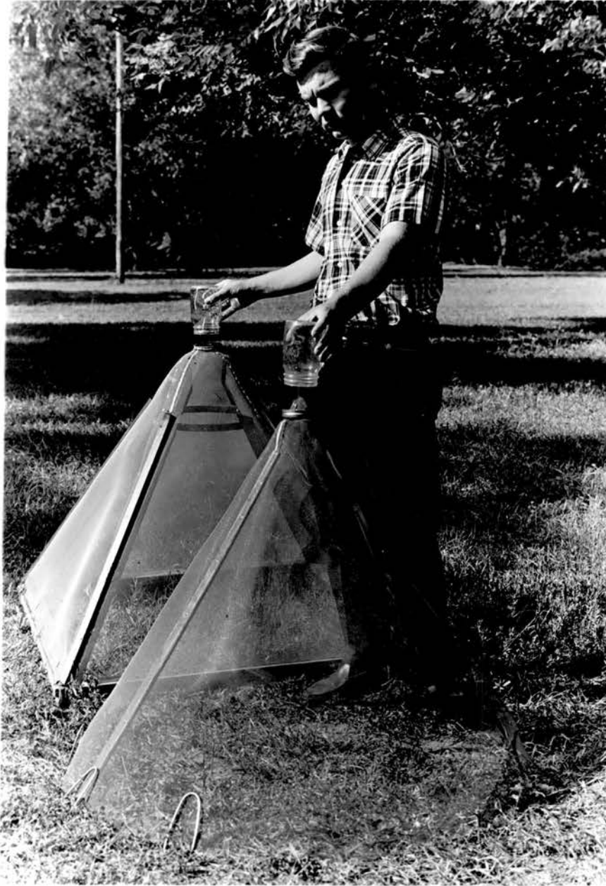
Figure 1. Comparison of pyramid trap to simplified cone trap used in flight habit studies.
