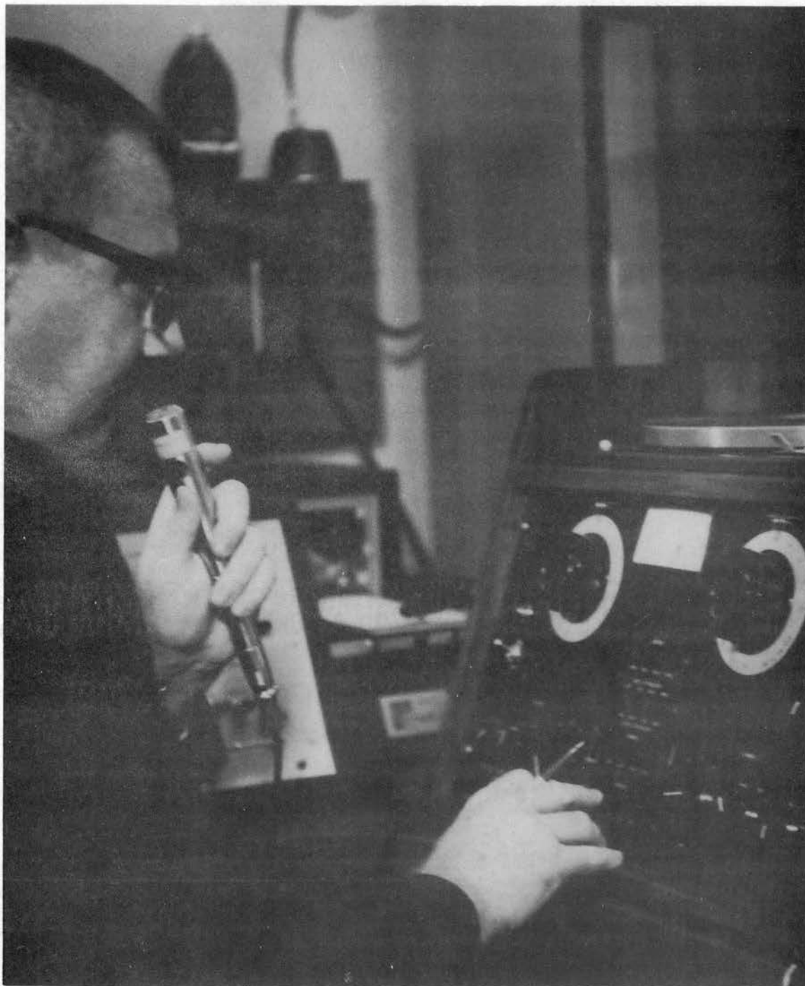
Figure 1. Administration of the SRT and Speech Discrimination Tests on the Grason-Stradler Speech Audiometer
