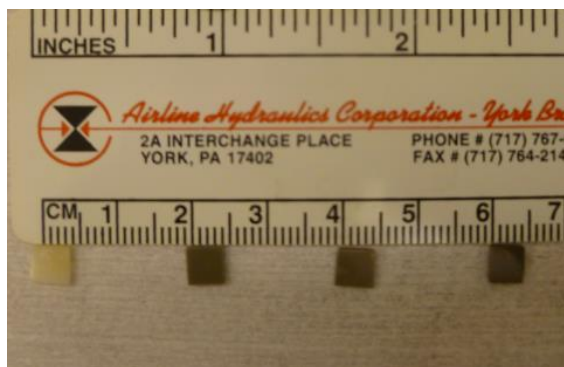
Figure 3.5: AgNW/N66 samples prepared for nano-indentation. Ag weight fraction from left to right is 0%, 1.49%, 3.28% and 6.74%, respectively.
