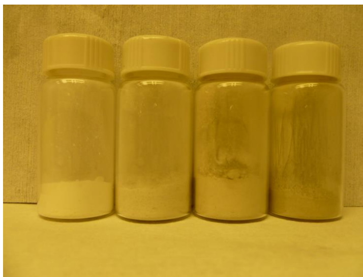
Figure 4.4: AgNW/N66 composite microparticles. Weight fraction of Ag from left to right is 0%, 1.49%, 3.28% and 6.74%.
