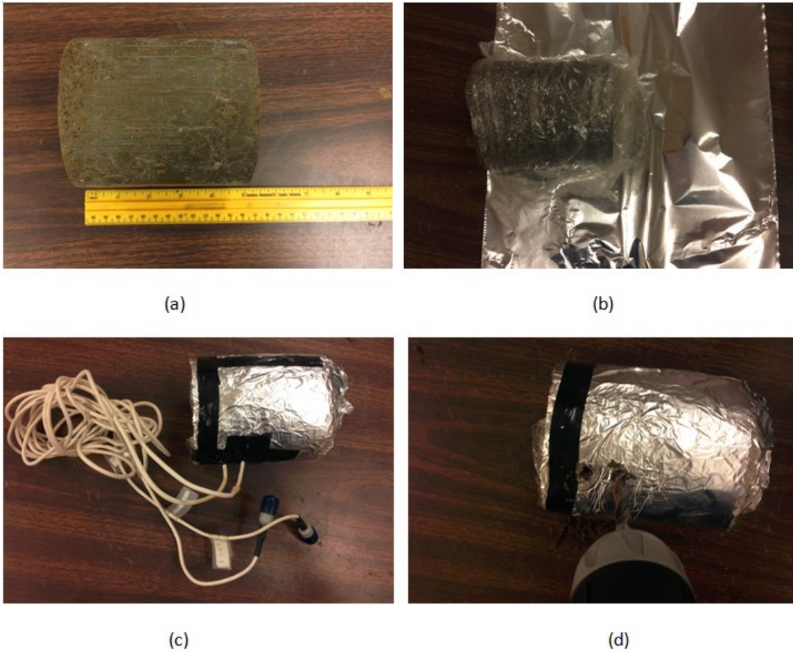
Figure 4.9 Thermocouple Psychrometer Installations
