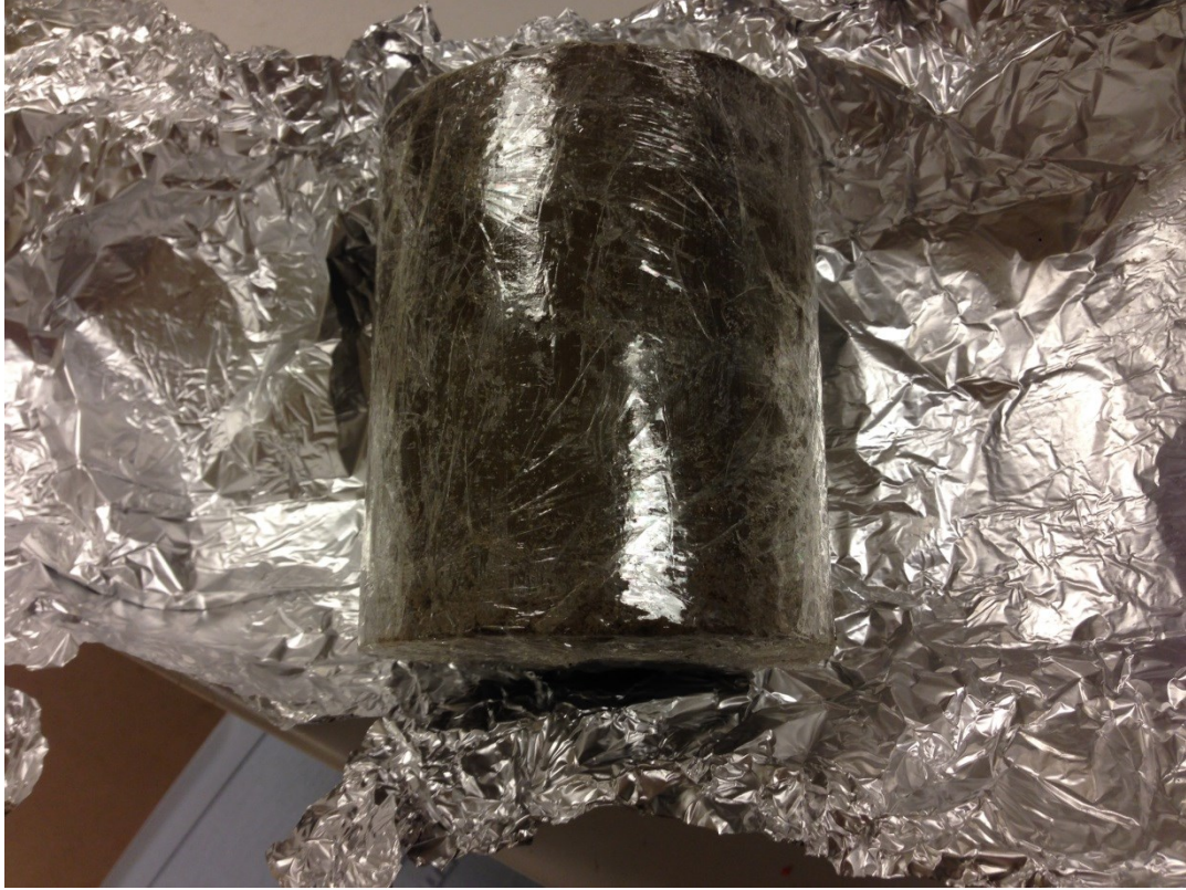
Figure 4.1 Compacted Soil Specimen Curing in Plastic Wrap and Aluminum Foil
