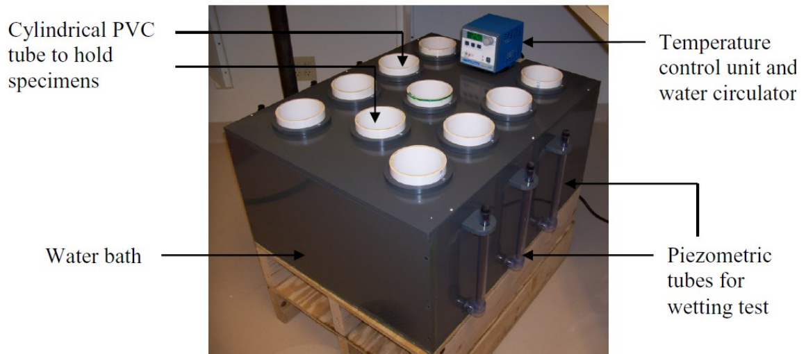
Figure 4.4 Water Bath for Calibration (Mabirizi 2010)
