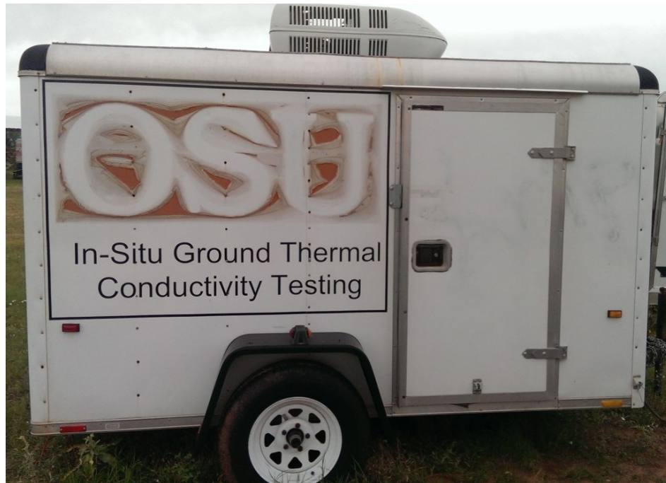
Figure 3-4: Heat injection trailer
