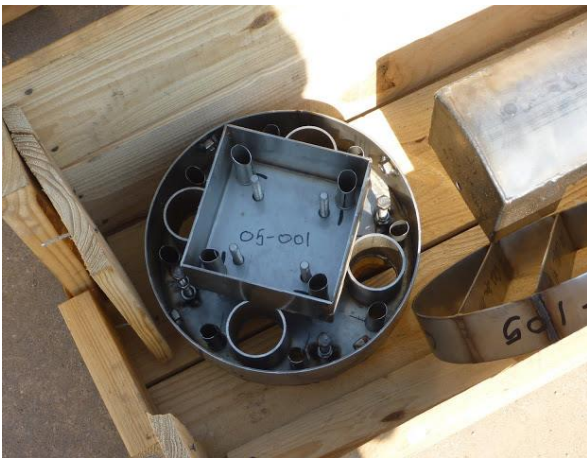
(e) Liquid distributor for rectifier and packing support plate
