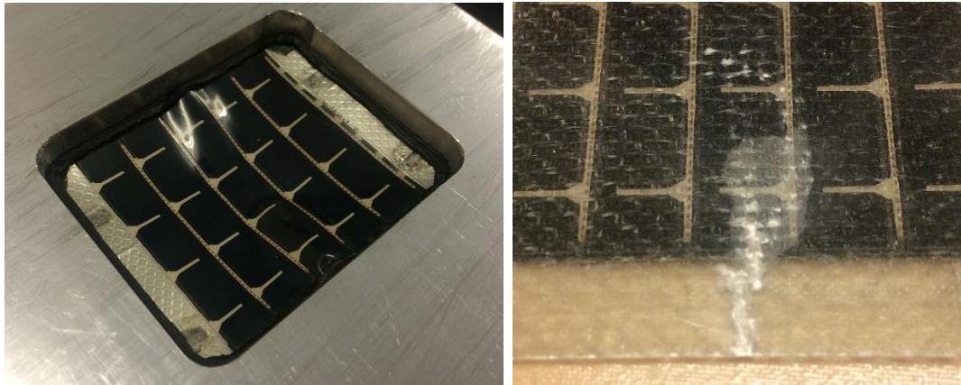
Figure 78: Left: The specimen with no laminated was observed to experience a significant level of delamination from its fiberglass backing. Right: The delamination experienced in the 9.0 oz laminated sample produced a noticeable defect in the specimen in the form of a void, which is believed to have reduced cell performance significantly by reducing light transmission
