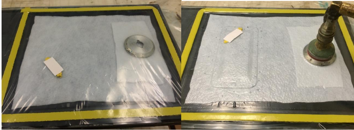
Figure 29: Bagging material is sealed around layup specimen (left) and vacuum is applied (right)
