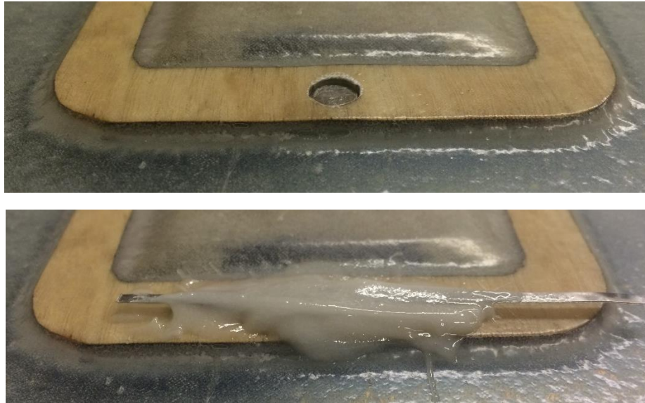
Figure 85: An external view of the socket after holes for the socket's magnets have been drilled with the corresponding magnet of the panel visible through the hole (Top) and the magnet, with its tabs exposed, after it has been epoxied into place with electrical contact between the socket and the panel established (Bottom)
