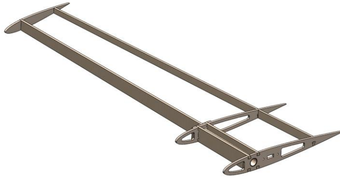
Figure 57: Wing structure, showing ribs, shear webs and joinin rod structure
