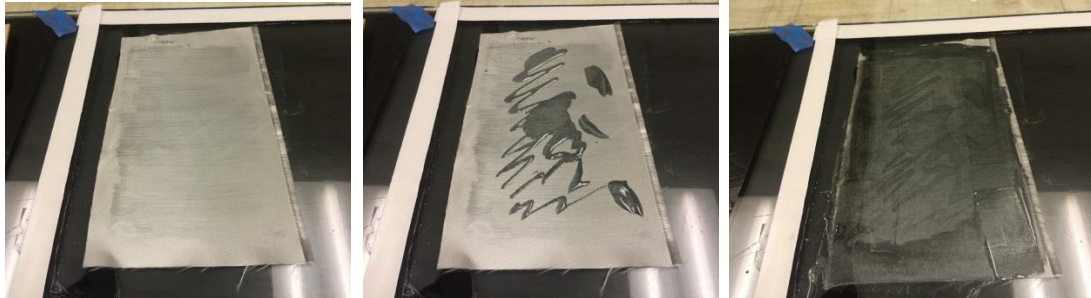
Figure 26: A sample of fiberglass as it is infused with epoxy on its parting surface from left to right
