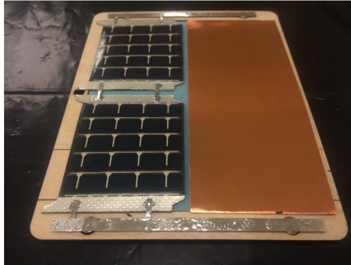
Figure 86: The materials of the prototype removable solar panel with working cells, test fitted prior to layup
