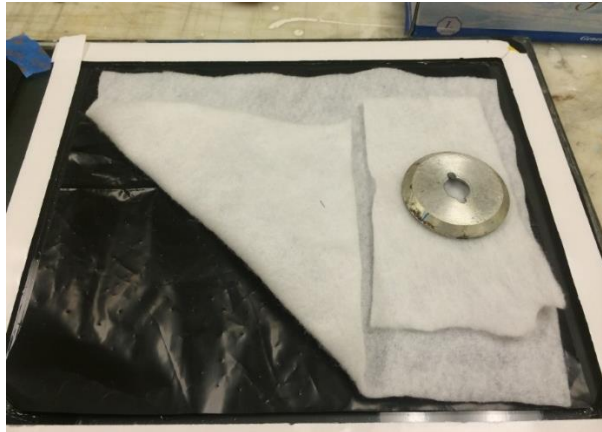
Figure 28: Bagging materials; Bleeder is black and porous with white Breather placed on top.
