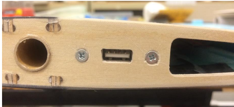
Figure 90: The female USB connector, as it was mounted in the root rib of the wing near the main spar
