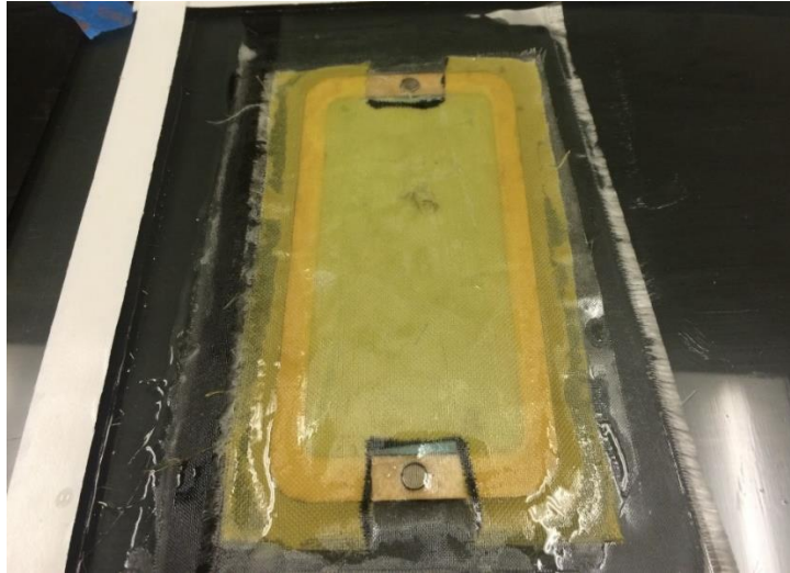
Figure 27: A multi-layer layup specimen before it is bagged and vacuumed to the parting surface
