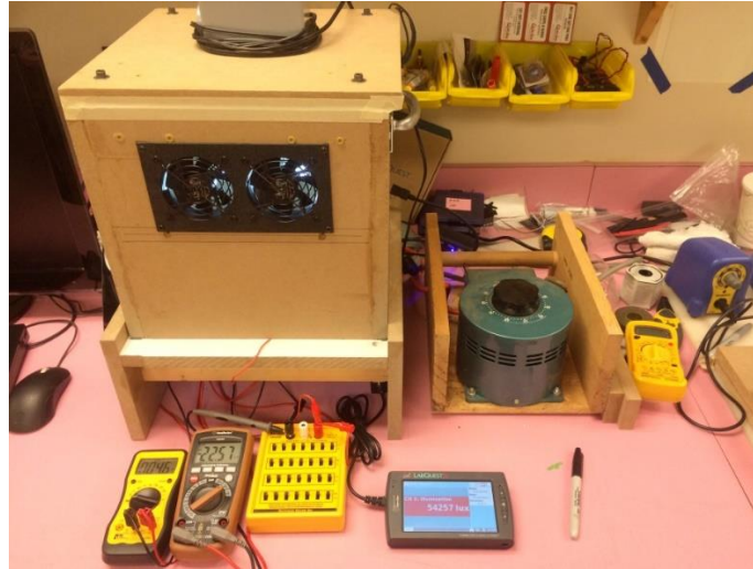
Figure 51: Cell testing apparatus with light box, test platform, multimeters, decade resistance box and vernier datalogger connected to thermocouple and light intensity sensor
