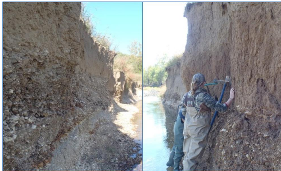
Figure 2.6. Example of “mini” JET being performed (right) and example of typical bank profile (left).
