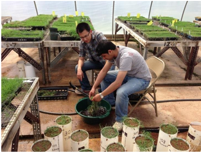
Fig 1. Washing and planting of grasses in mini-lysimeters.
