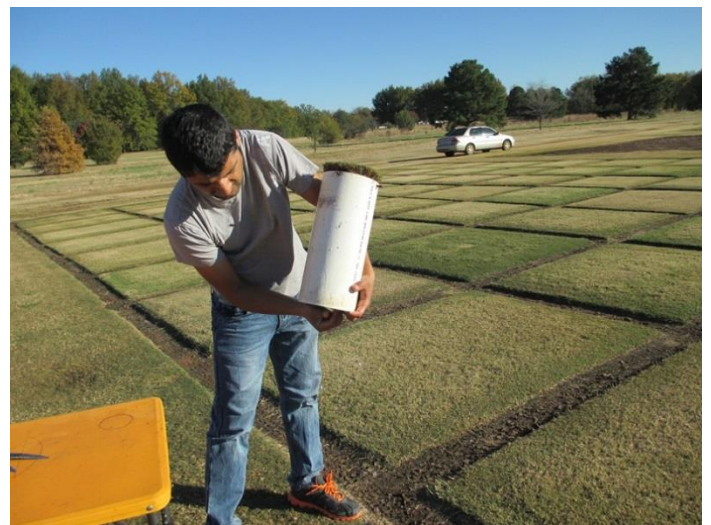
Fig 8. Opening of valve to bring a mini-lysimeter in field capacity.
