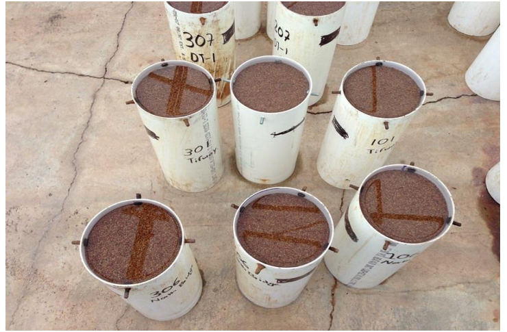
Fig 2. Mini-lysimeter filled with calcined clay as a growing medium.
