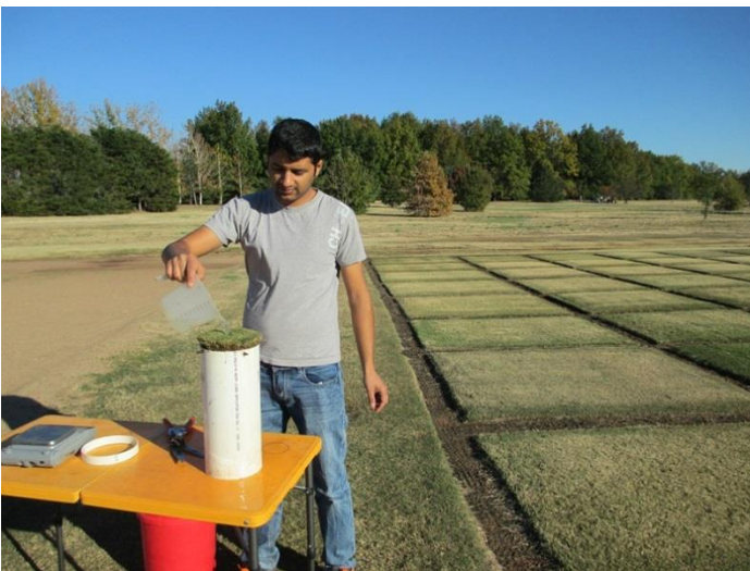
Fig 7. Saturation of a mini-lysimeter.
