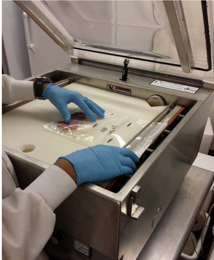
Figure 4. Vacuum-packaging using a Hobart's H-Series vacuum-packaging equipment.
